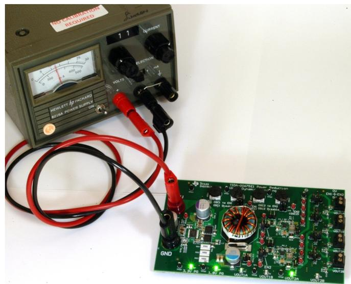
**Figure 11. Test Setup, Board Powered-Up**
