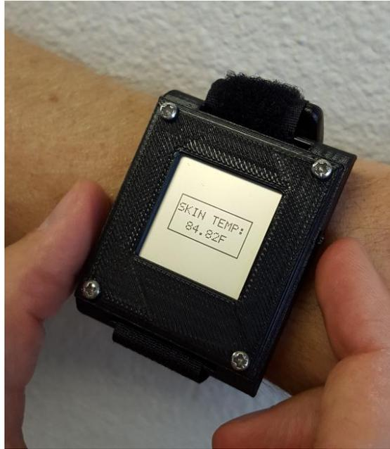
Figure 21: Holding the Button for Two Seconds Changes Temperature to Fahrenheit
