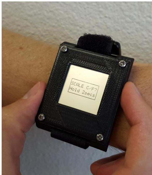
**Figure 20: Pressing the Button Again for the Scale Change Menu**
