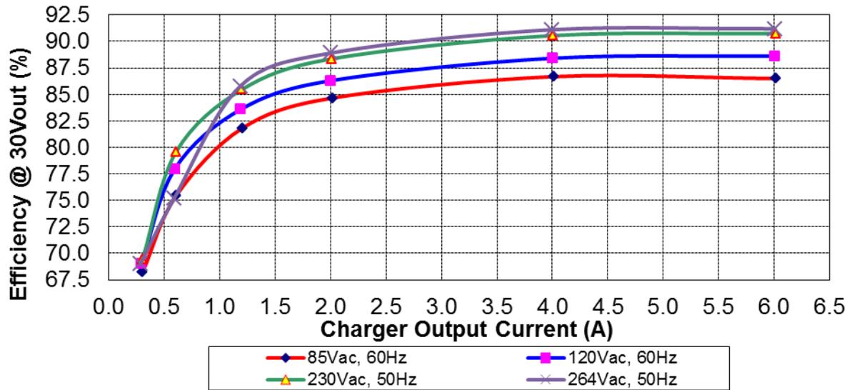
Efficiency of the converter (plug-to-plug) versus Vac & Output current with different Vout:
