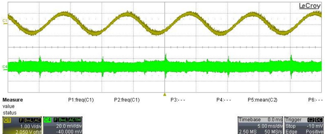
This picture below shows the ripple voltage on 5Vout and 12Vout, both fully loaded, while the main output was off (S1 switch was OFF); the input voltage was 230Vac.
