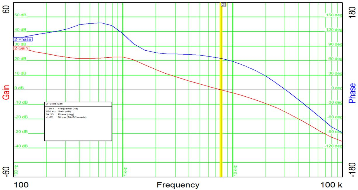
Current loop (TP23, TP24, TP25):  $F_{co} = 6.944\text{KHz}$ ,  $PM = 68.22\text{ deg}$ ,  $GM = 15.41\text{dB}$ .
