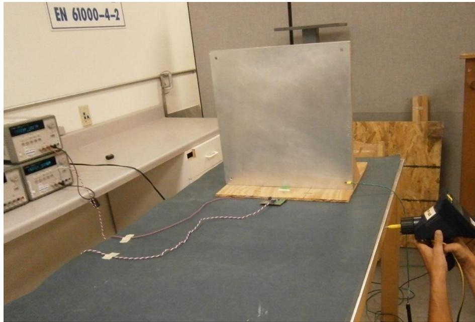
**Figure B-3: 8kV ESD Horizontal Contact Discharge**
