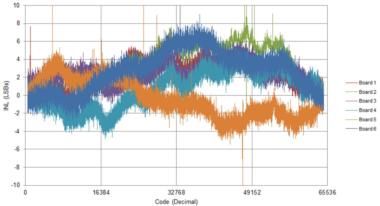
Figure 10: Output Current INL vs. Input Code
