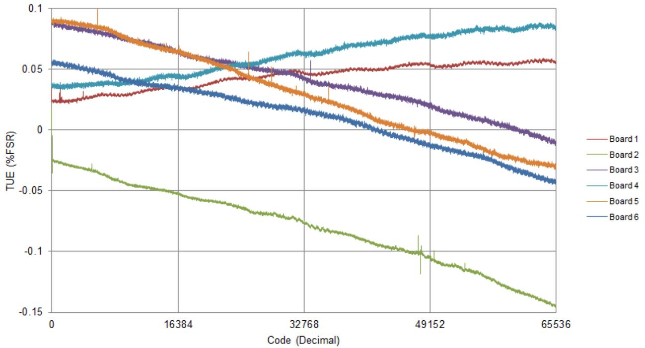
Figure 9: Output Current TUE vs. Input Code
