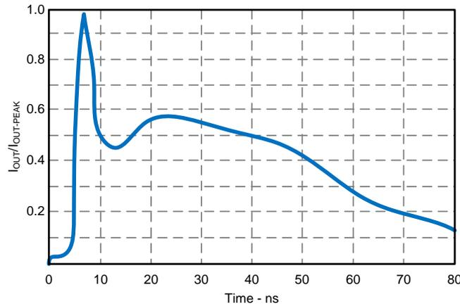
Figure 4: IEC61000-4 ESD Test Pulse
