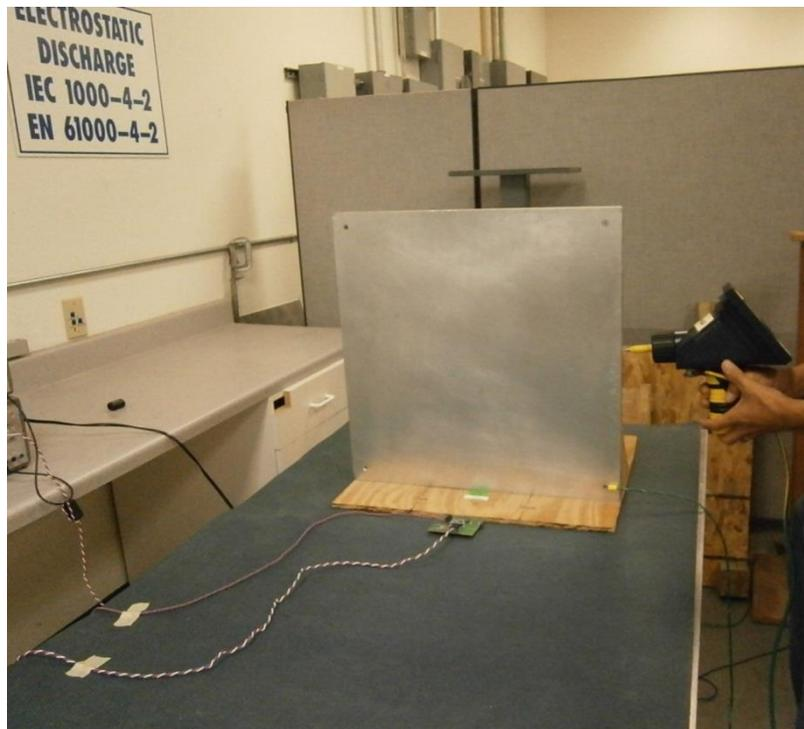
Figure B-2: 8kV ESD Vertical Contact Discharge
