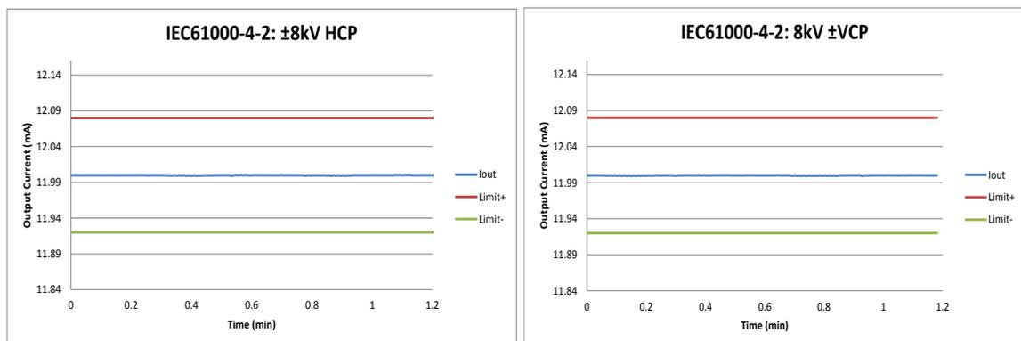
**Figure 11:  $\pm 8$  - kV ESD Horizontal (left) and Vertical (right) Coupling Planes (HCP and VCP)**
