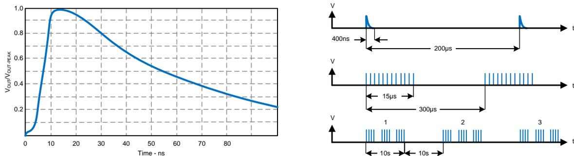
Figure 5: IEC61000-4 EFT Test Pulses
