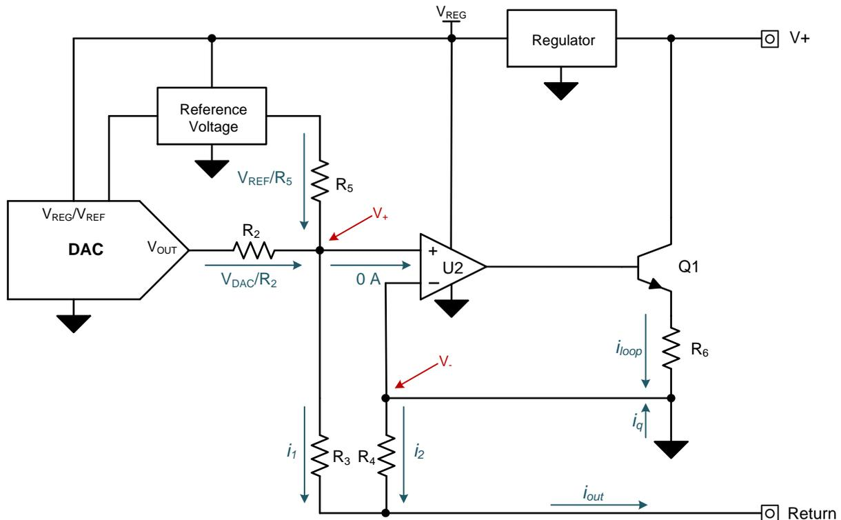
**Figure 2: Simplified Voltage to Current Converter Circuit**
