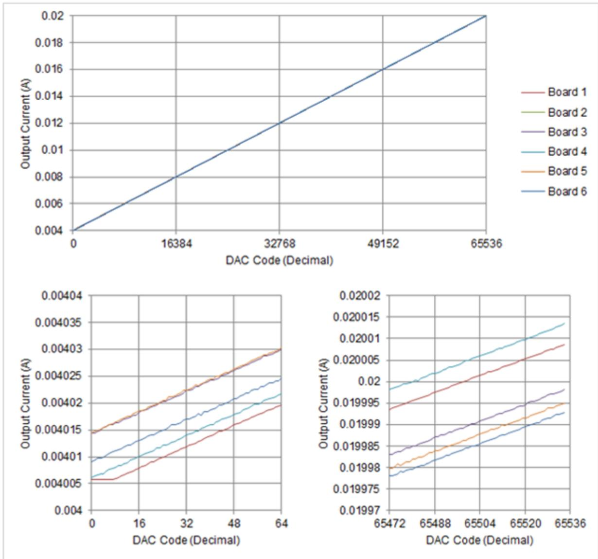
**Figure 8: Output Current vs. Input Code**
