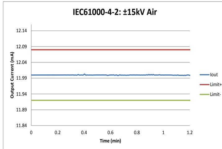
**Figure 13: ±15 kV ESD Air Discharge**
