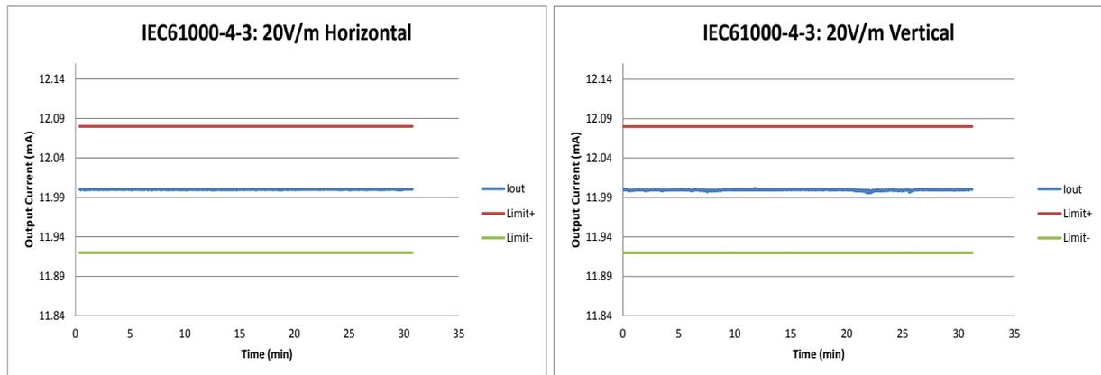
Figure 14: Horizontal (left) and Vertical (right) Polarity at 20V/m
