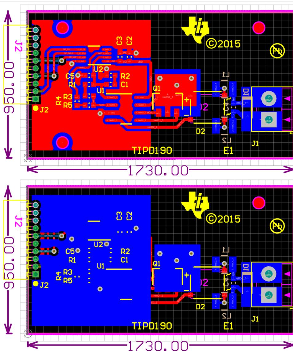
Figure 7: PCB Layout
