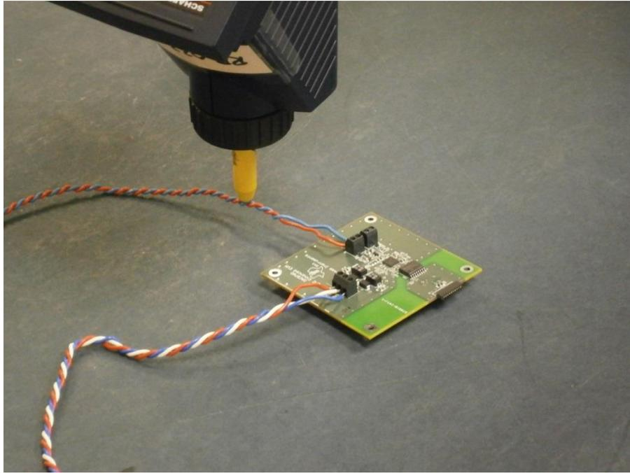
Figure B-1: 15kV ESD Air Discharge
