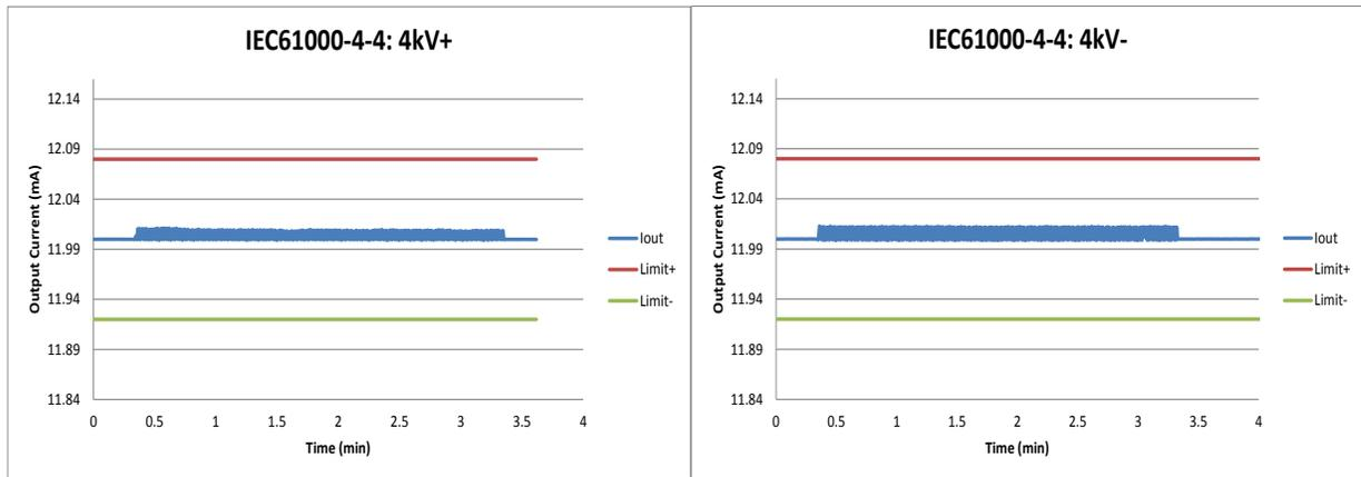
**Figure 16: 4kV EFT Positive (left) and Negative (right)**
