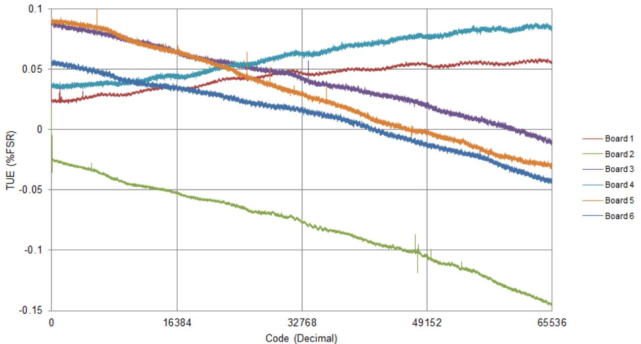
**Figure 1: Measured TUE vs. Input Code**
