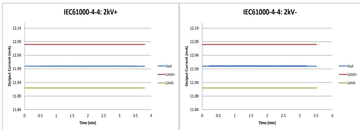
Figure 15: 2kV EFT Positive (left) and Negative (right)
