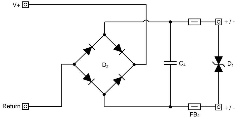
**Figure 3: Diode Bridge & Protection Circuit**
