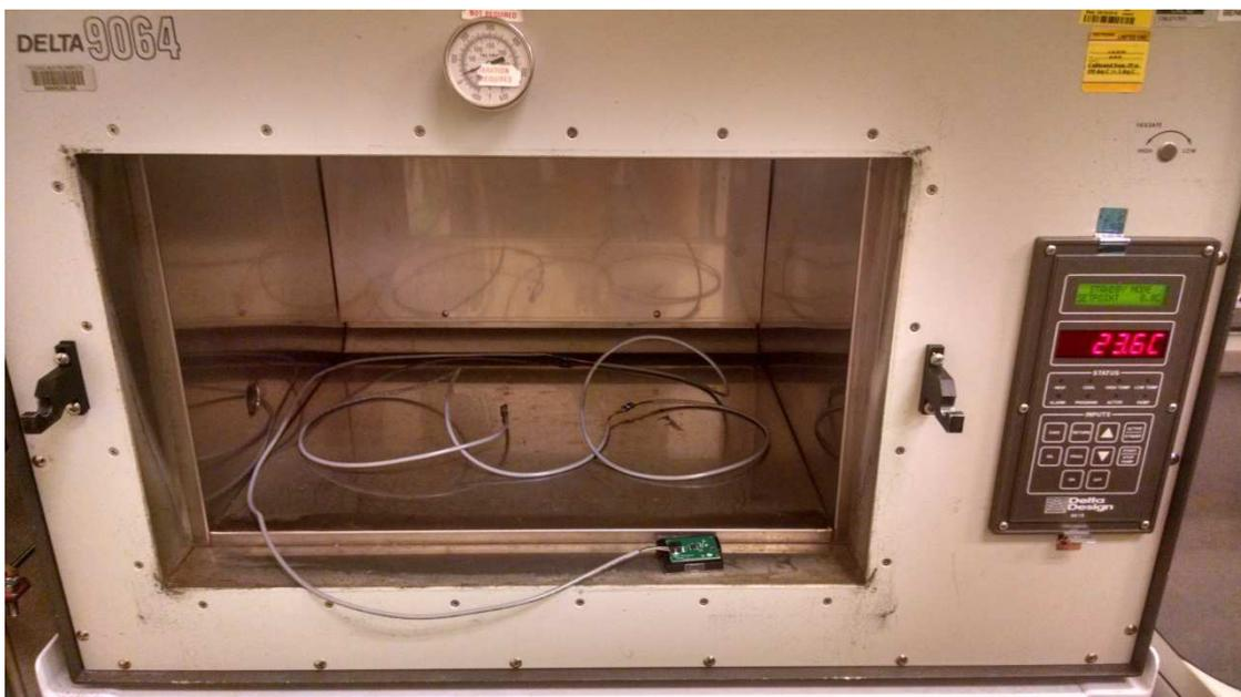
**Figure 12: Delta 9064 Environmental Test Chamber and Test Setup**
