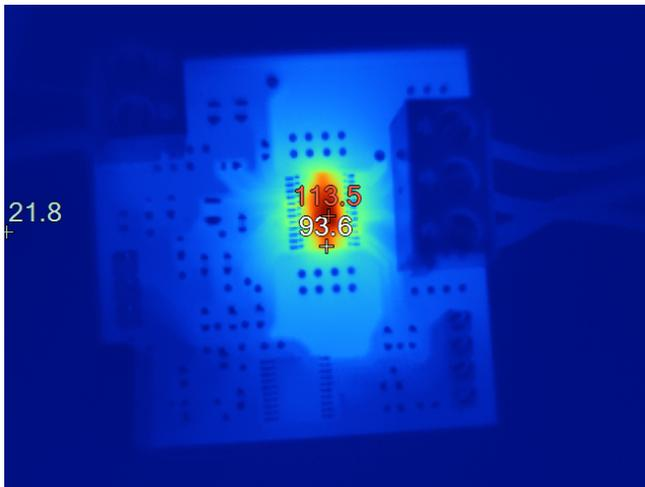
Figure 17. Top Side Thermal Image at 50.4 W, and ≈220°C Ambient
