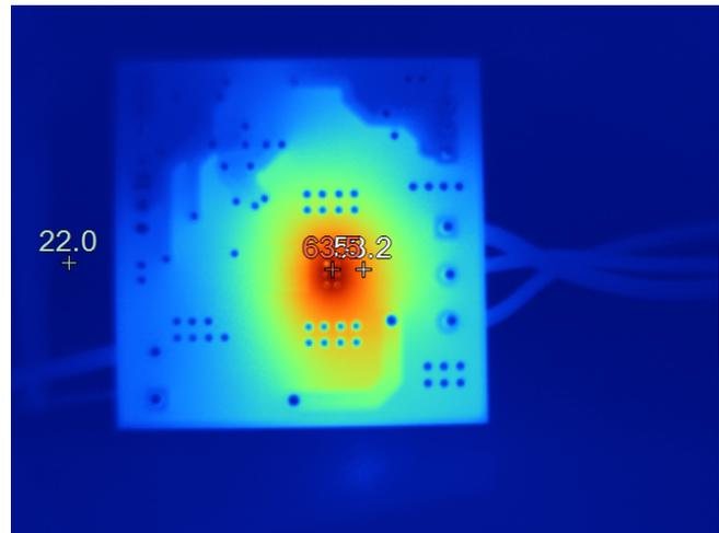
Figure 18. Bottom Side Thermal Image at 50.4 W and ≈220°C Ambient
