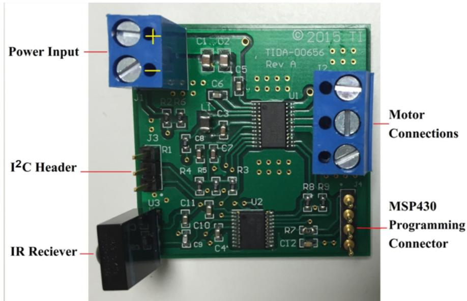
Figure 11. Assembled TIDA-00656 Rev A Board
