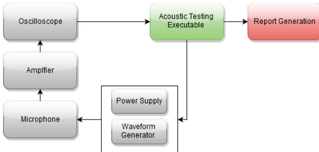
Figure 20. Test Setup Block Diagram
