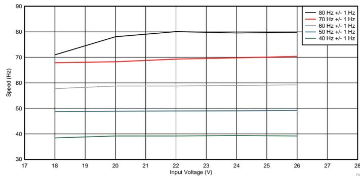
Figure 19. Speed Regulation wrt Input Voltage
