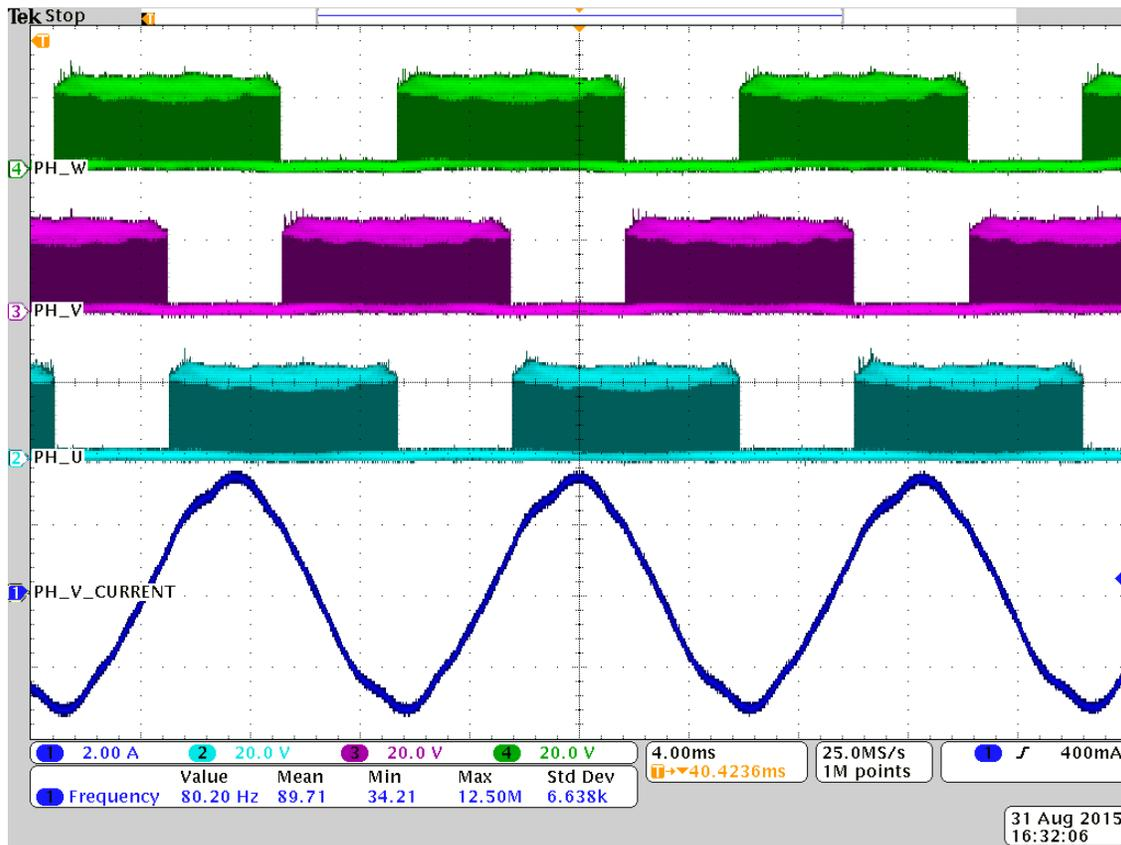
Figure 14. Runtime at 24 V, 2.1 A,  $\approx 80$  Hz, and 50 W
