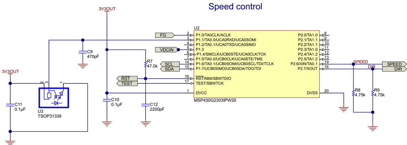
Figure 3. Speed Control Section
