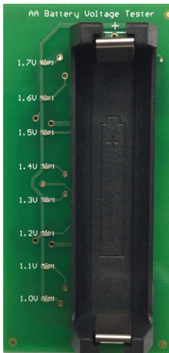
Figure 7. AA Battery Tester Without Battery
