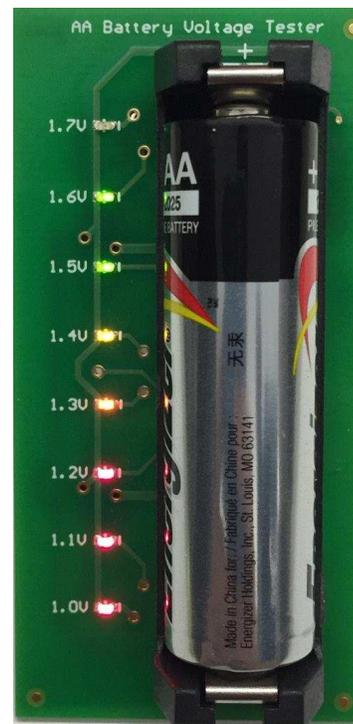
Figure 8. AA Battery Tester With Battery
