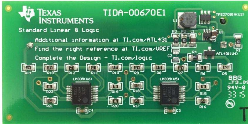
Figure 6. Top View of AA Battery Tester
