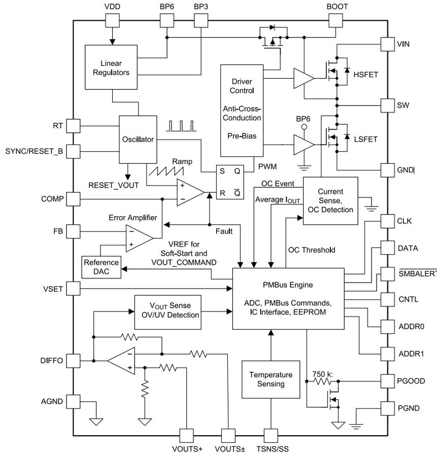
Figure 3. TPS544C25 Functional Block Diagram
