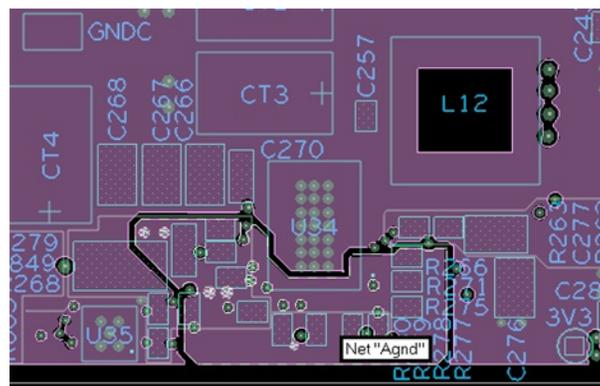
Figure 7. Analog Ground on Layer 2
