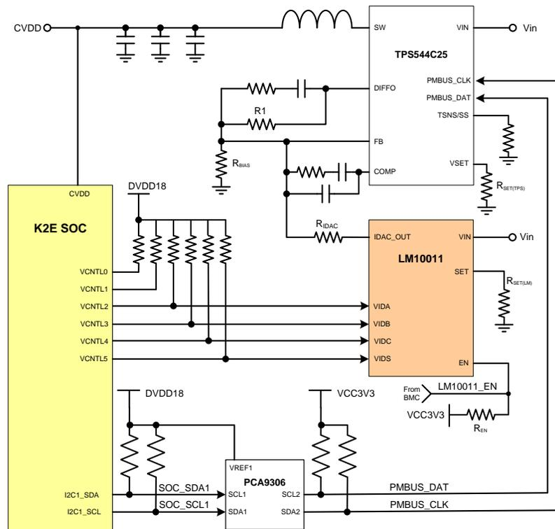
Figure 2. Circuit Supporting Both LM10011 and PMBus Control
