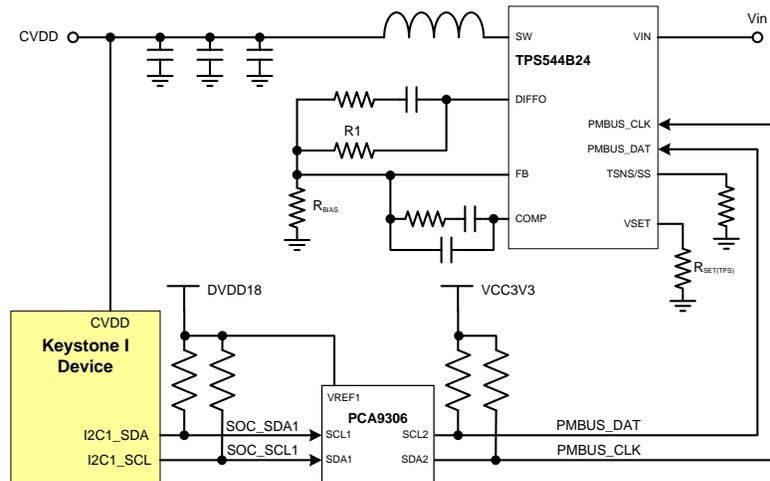
Figure 1. CVDD Power Circuit Using the TPS544C25 Controlled by PMBus
