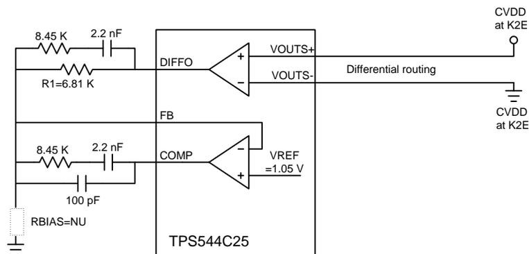
**Figure 4. Output Voltage Control Diagram**
