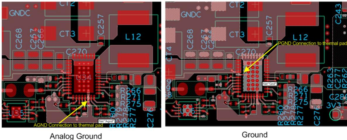
Figure 6. Analog Ground and Ground
