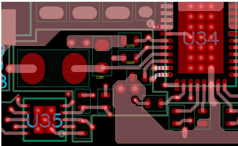
Figure 8. BP3, BP6, and VDD Bypass Position
