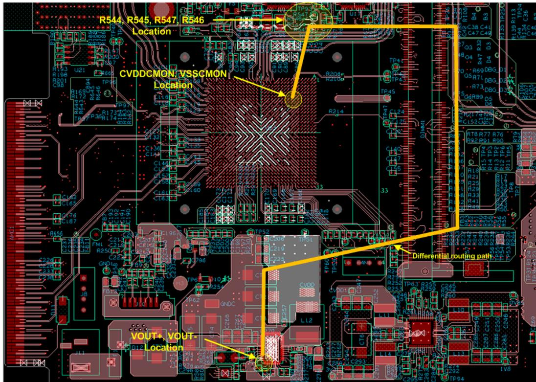
Figure 9. Sense Line Routing
