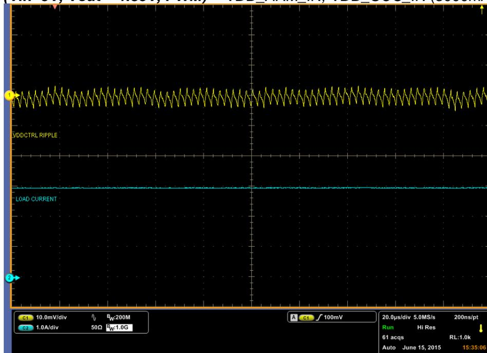
**Figure 15 – VDDCTRL Voltage Ripple @ 25C**
