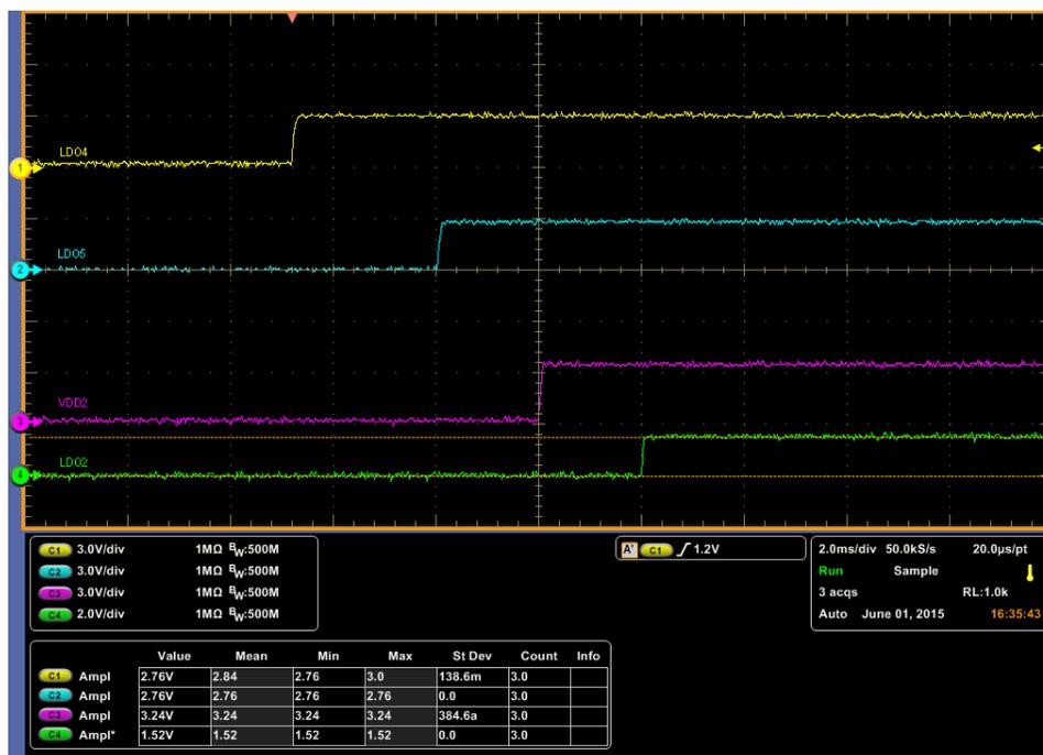
Figure 21 – Power-Up Sequence (No Load) Voltage Waveforms (LDO4\_3.0V, LDO5\_2.8V, VDD2\_3.3V, LDO2\_1.5V)
