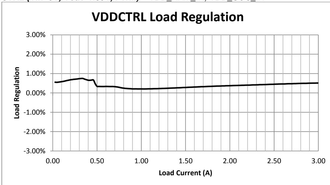
**Figure 11 – CTRL1 Load Regulation @ 25C**
