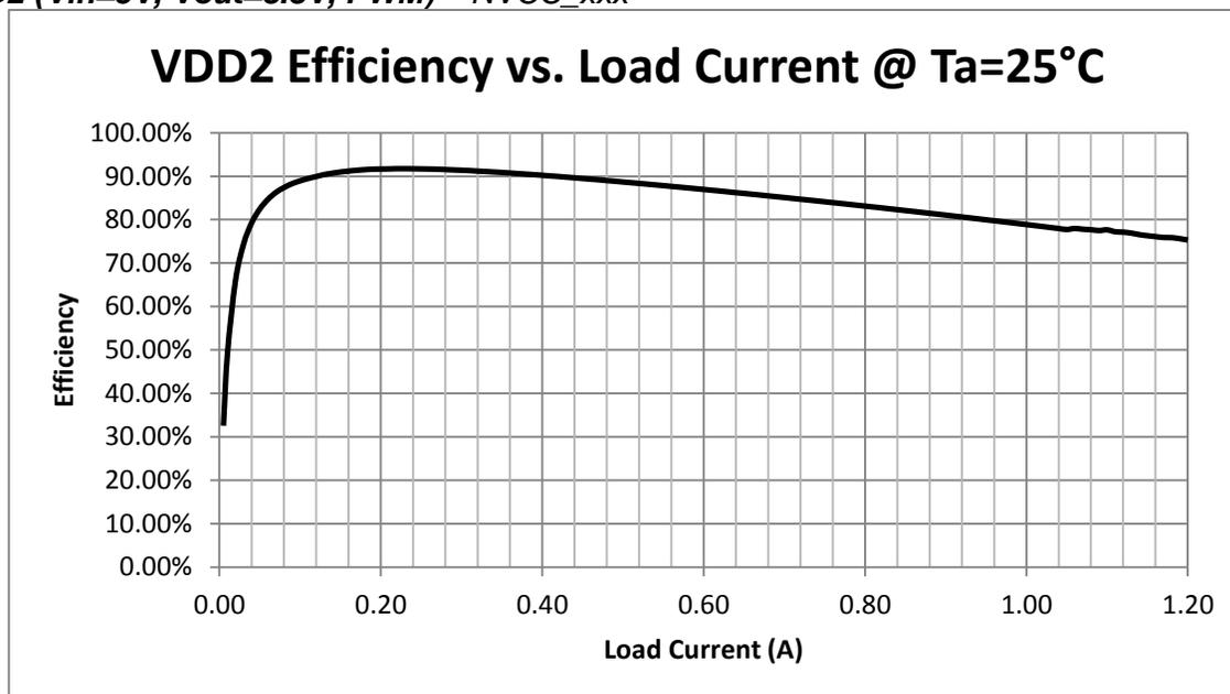
Figure 5 – DCDC2 Efficiency @ 25C
