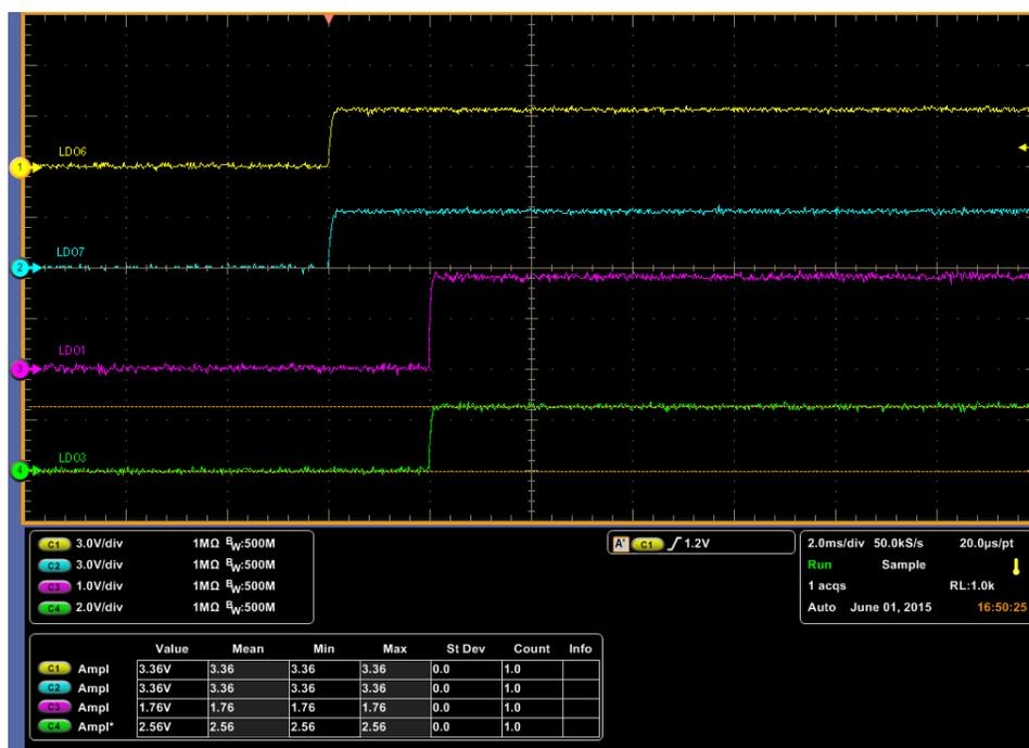
Figure 22 – Power-Up Sequence (No Load) Voltage Waveforms (LDO6\_3.3V, LDO7\_3.3V, LDO1\_1.8V, LDO3\_2.5V)
