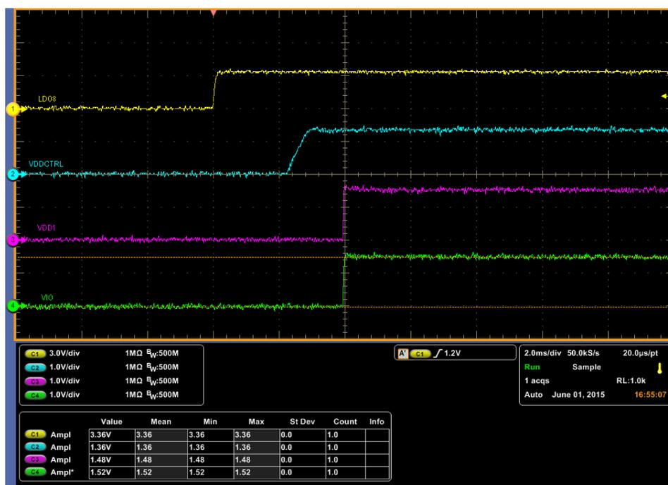
Figure 23 – Power-Up Sequence (No Load) Voltage Waveforms (LDO8\_3.3V, VDDCTRL\_1.35V, VDD1\_1.5V, VIO\_1.5V)
