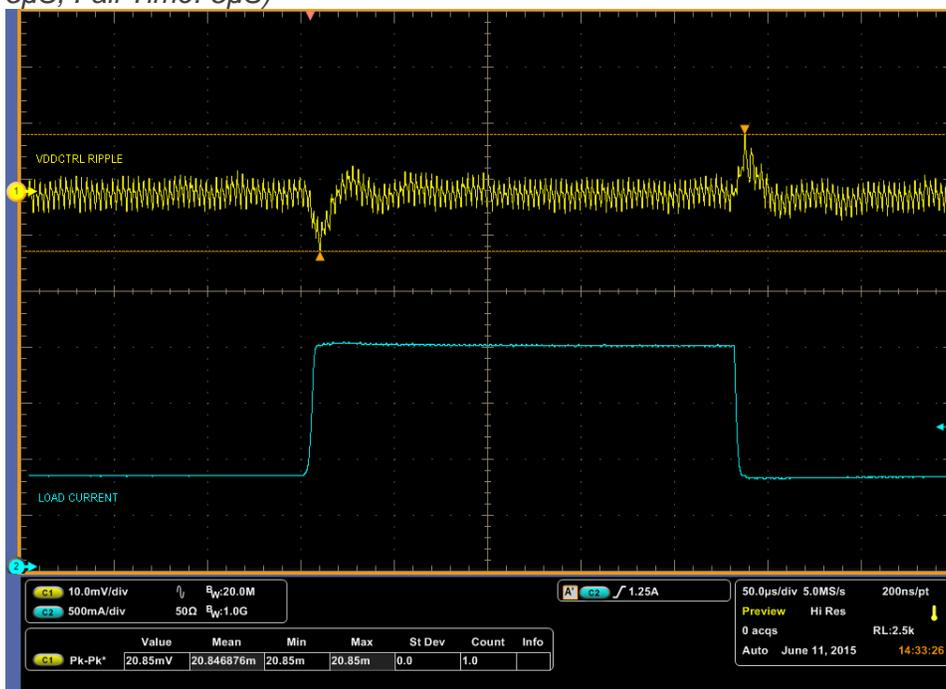
**Figure 19 – VDDCTRL Load Transient @ 25C**
