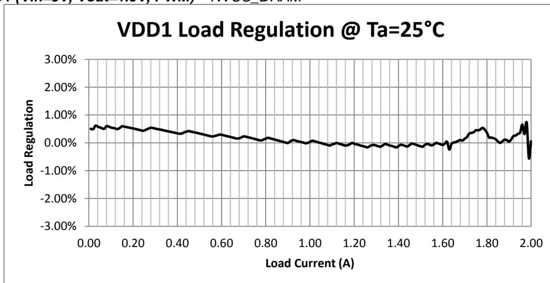
Figure 8 – DCDC1 Load Regulation @ 25C
