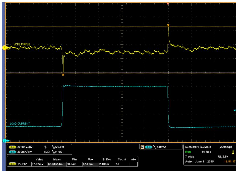
Figure 17 – DCDC2 Load Transient @ 25C
