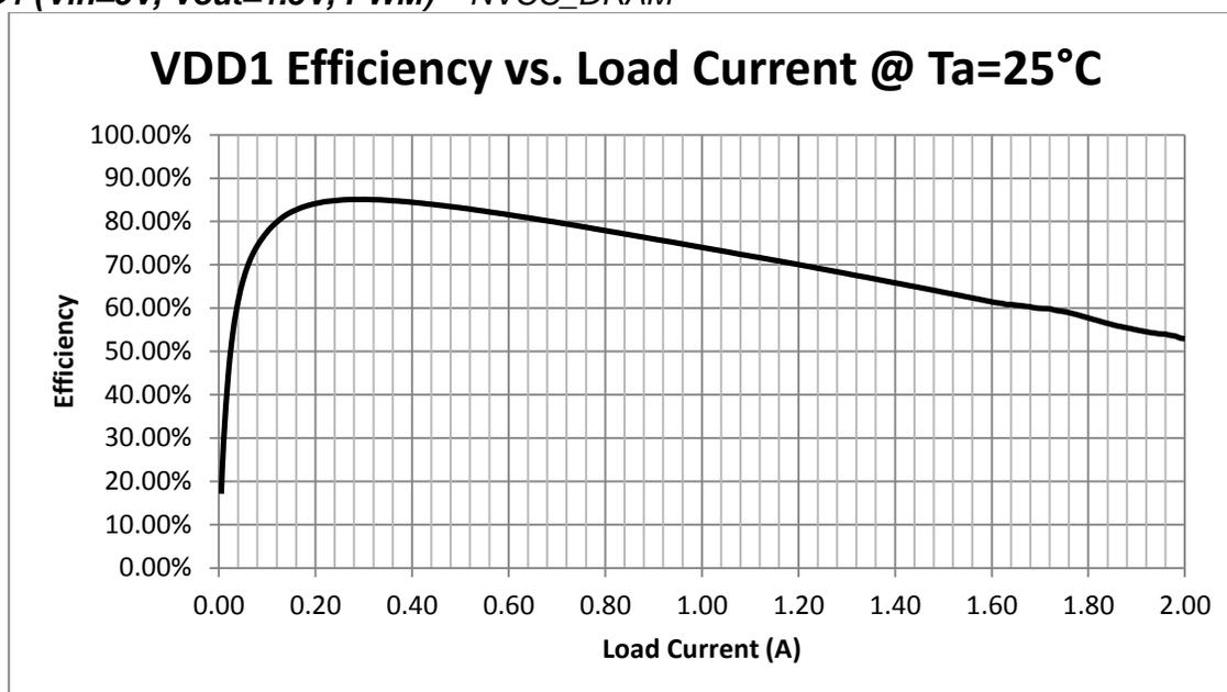
Figure 4 - DCDC1 Efficiency @ 25C
