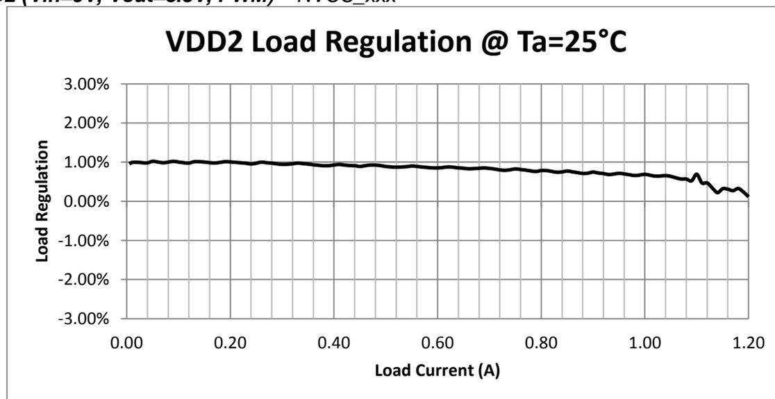
Figure 9 – DCDC2 Load Regulation @ 25C
