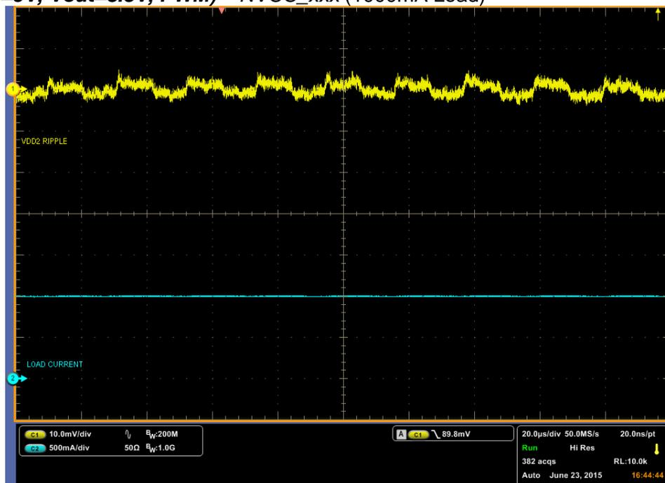
Figure 13 – DCDC2 Voltage Ripple @ 25C
