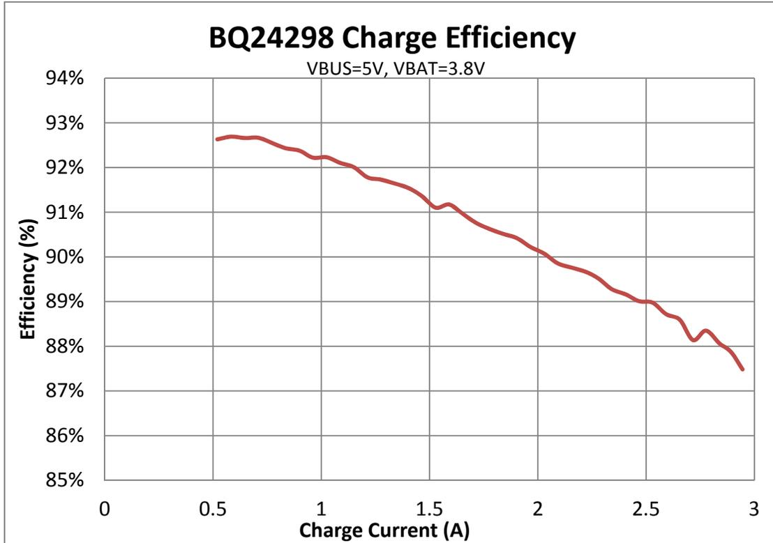
**Figure 3. TIDA-00591 Charging Efficiency**
