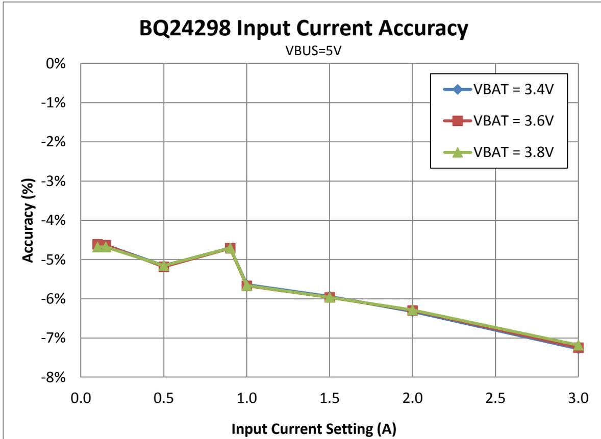
**Figure 6. TIDA-00591 Input Current Accuracy**
