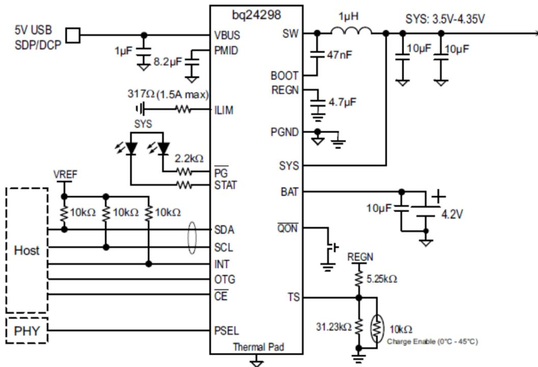
**Figure 2. bq24298 Application Circuit**
