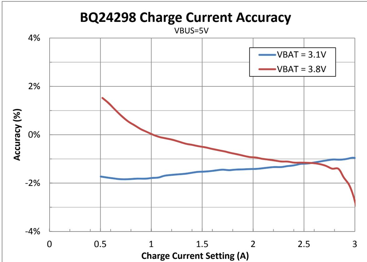
**Figure 5. TIDA-00591 Charge Current Accuracy**
