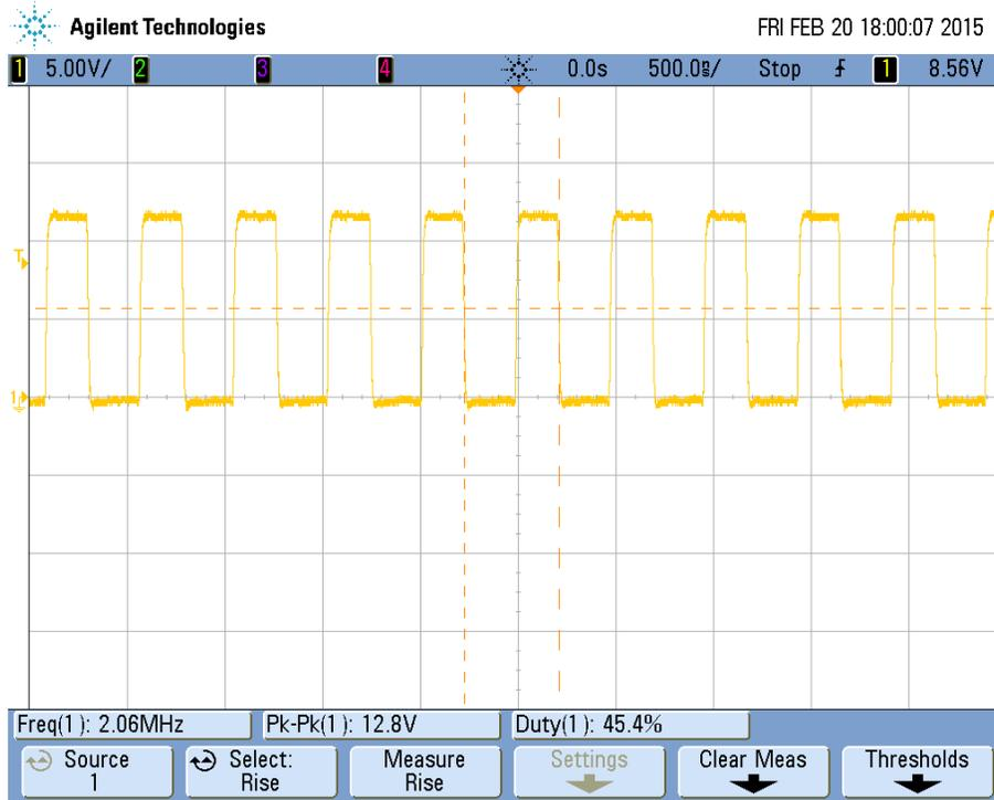
Figure 15 Switching waveform at 3A load, 12Vin, PWM
