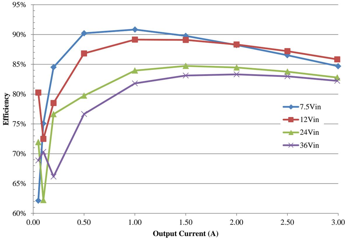
Figure 3 Power efficiency
