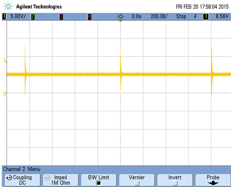
Figure 16 Switching waveform at no load, 12Vin, PFM
