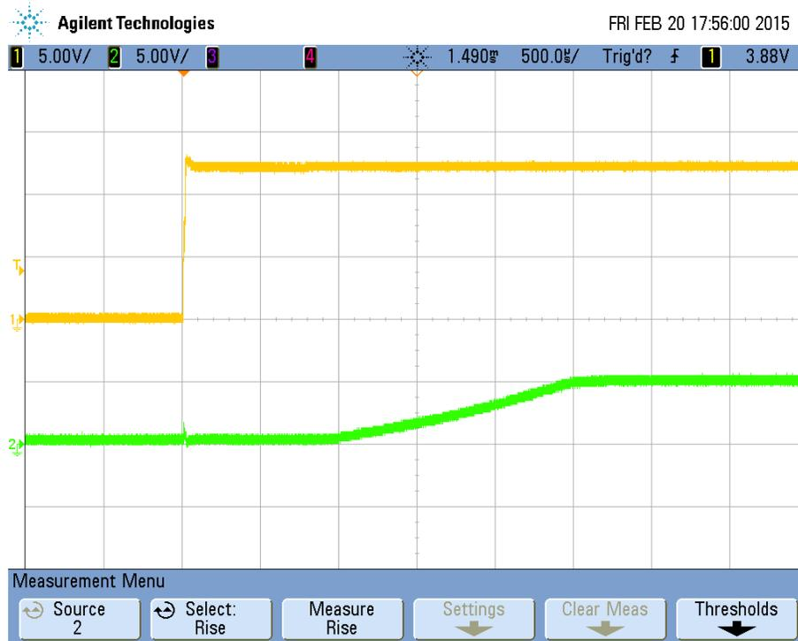
Figure 14 Start up into no load at 12Vin
