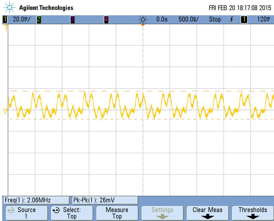
**Figure 21 Output ripple at 3A load, 12Vin**
