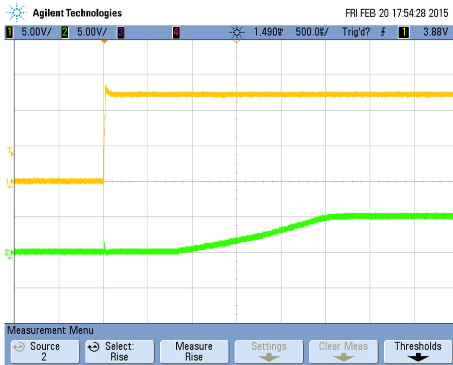
Figure 13 Start up into 3A load at 12Vin
