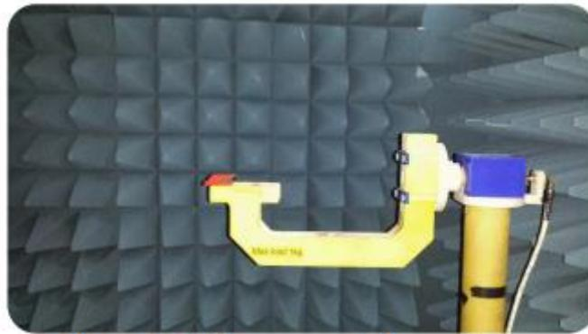
**Figure 4: Anechoic Chamber DUT Placement**
