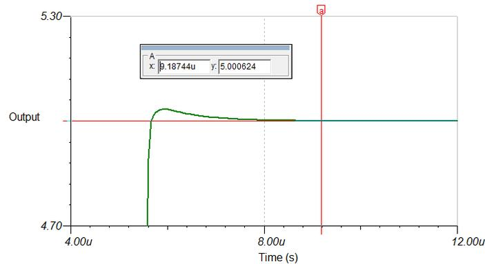
Figure 9. TINA-TI™ Simulated Small-Signal Settling
