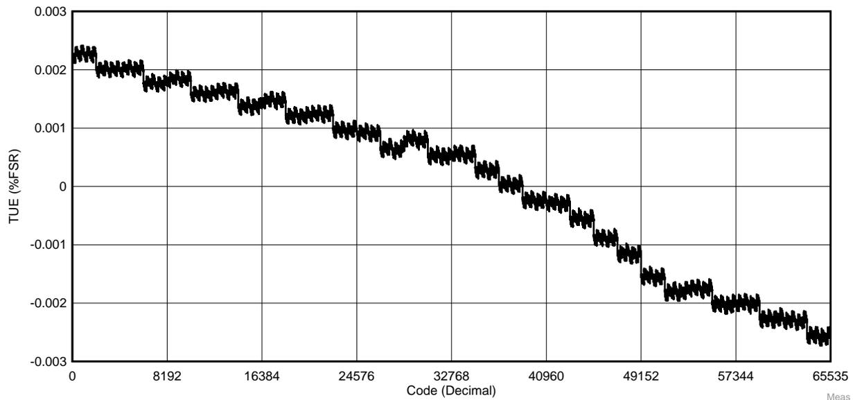
**Figure 11. Measured Total Unadjusted Error**
