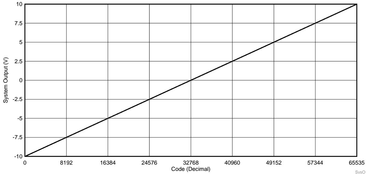
**Figure 10. Measured System Transfer Function**
