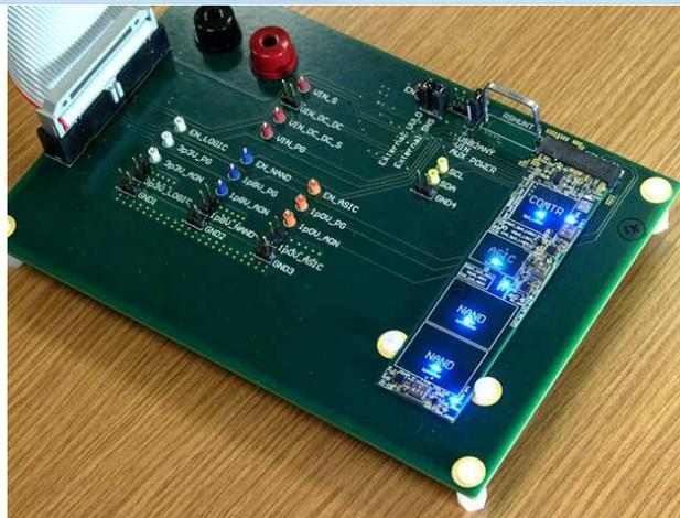
Figure 27. The 1-V Memory ASIC Power is Enabled
