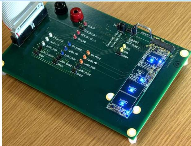
Figure 26. The 1.8-V NAND Power is Enabled
