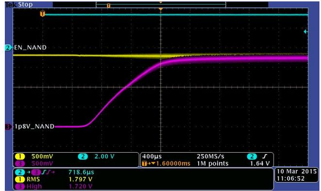
Figure 63. TPS22964C  $t_D$  Measurement at  $V_{IN} = 1.8 V$ ,  $R_L = 0.72 \Omega$ ,  $I_{OUT} = 2.5 A$
