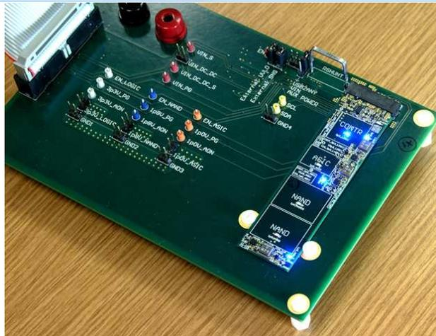
Figure 25. The 3.3-V Controller Power is Enabled
