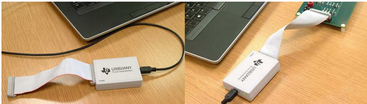
**Figure 20. The Ribbon Cable is Connected Between the USB2ANY and Interposer Board**
