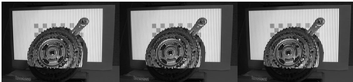
**Figure 35** Vertical three phase patterns
