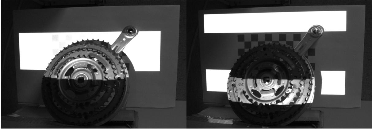
**Figure 48** Non-inverted and inverted horizontal gray code pattern 3 capture
