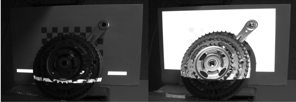
**Figure 46** Non-inverted and inverted horizontal gray code pattern 1 capture
