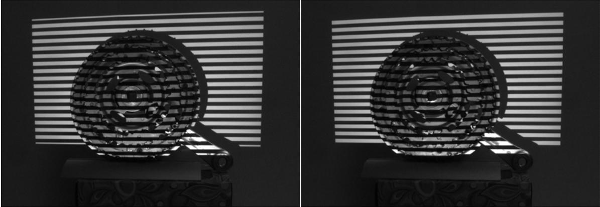
**Figure 29** Non-inverted and inverted horizontal gray code pattern 7 capture
