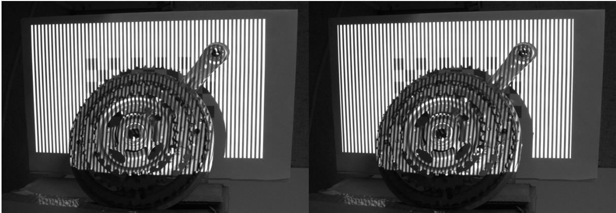
**Figure 43** Non-inverted and inverted vertical gray code pattern 8 capture
