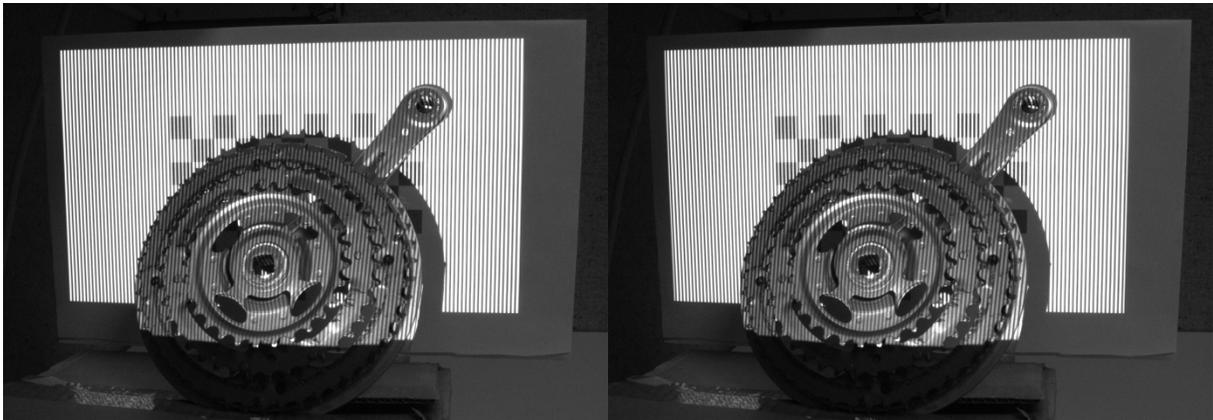
**Figure 44** Non-inverted and inverted vertical gray code pattern 9 capture
