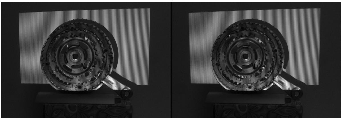
**Figure 22** Non-inverted and inverted vertical gray code pattern 9 capture
