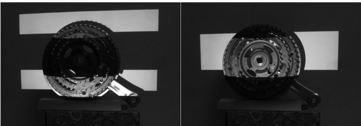
**Figure 25** Non-inverted and inverted horizontal gray code pattern 3 capture
