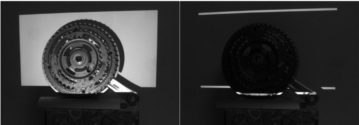
**Figure 24** Non-inverted and inverted horizontal gray code pattern 2 capture
