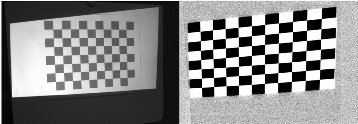
**Figure 5** Printed calibration board and projected calibration board position 4
