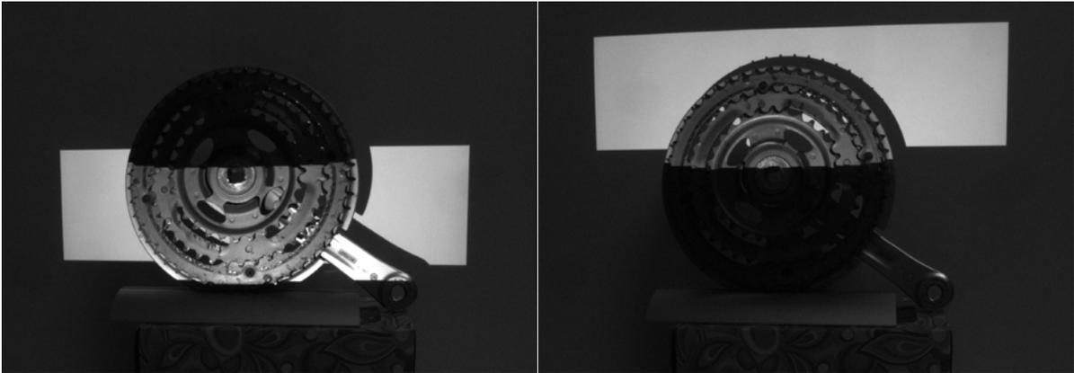
**Figure 23** Non-inverted and inverted horizontal gray code pattern 1 capture
