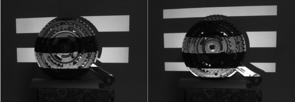
**Figure 26** Non-inverted and inverted horizontal gray code pattern 4 capture
