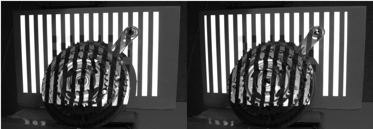
**Figure 41** Non-inverted and inverted vertical gray code pattern 6 capture
