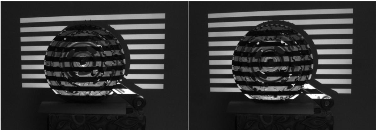
**Figure 28** Non-inverted and inverted horizontal gray code pattern 6 capture
