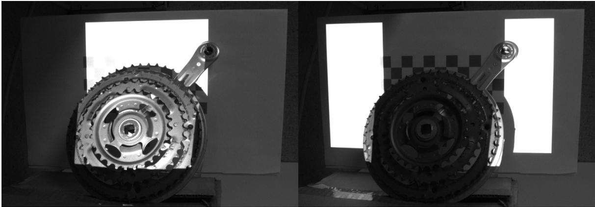
**Figure 37** Non-inverted and inverted vertical gray code pattern 2 capture
