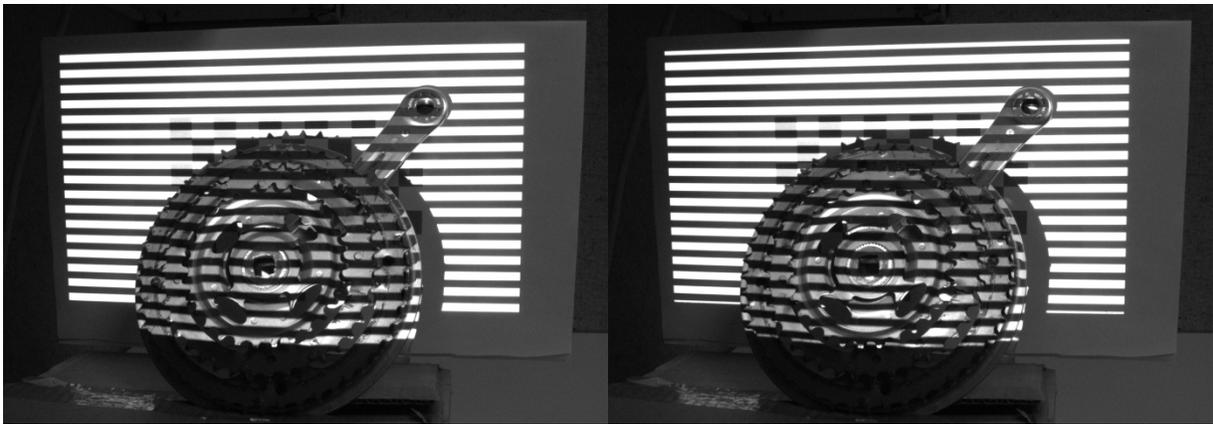
**Figure 52** Non-inverted and inverted horizontal gray code pattern 7 capture
