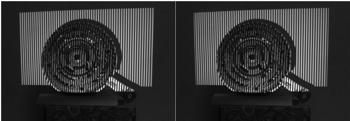
**Figure 21** Non-inverted and inverted vertical gray code pattern 8 capture
