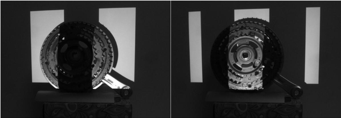
**Figure 16** Non-inverted and inverted vertical gray code pattern 3 capture
