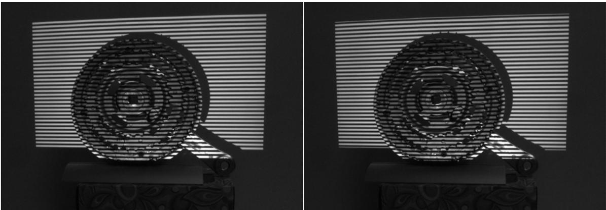
**Figure 30** Non-inverted and inverted horizontal gray code pattern 8 capture
