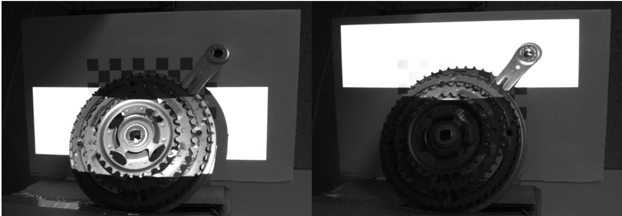
**Figure 47** Non-inverted and inverted horizontal gray code pattern 2 capture
