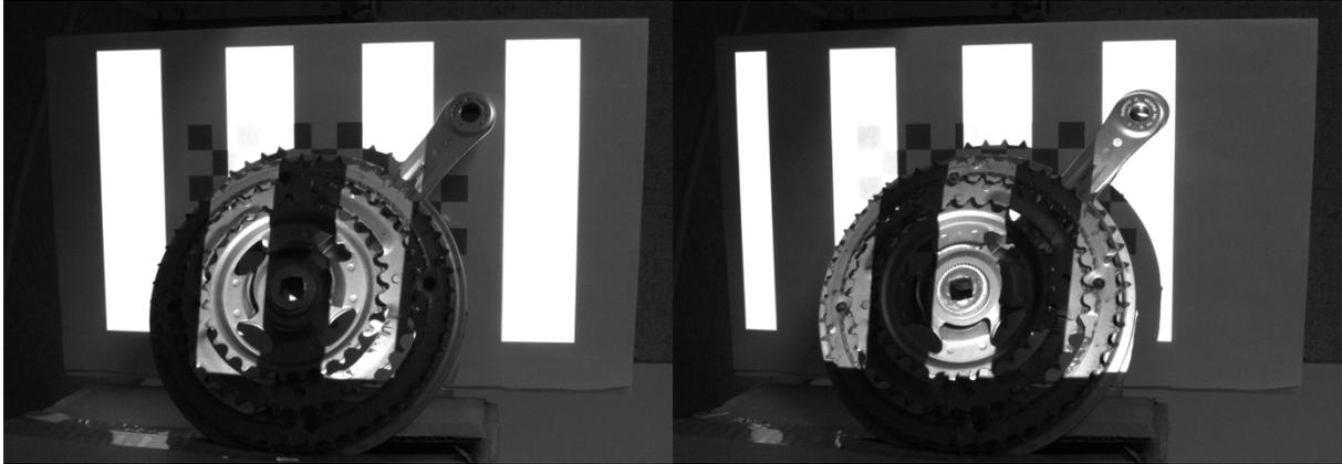
**Figure 39** Non-inverted and inverted vertical gray code pattern 4 capture
