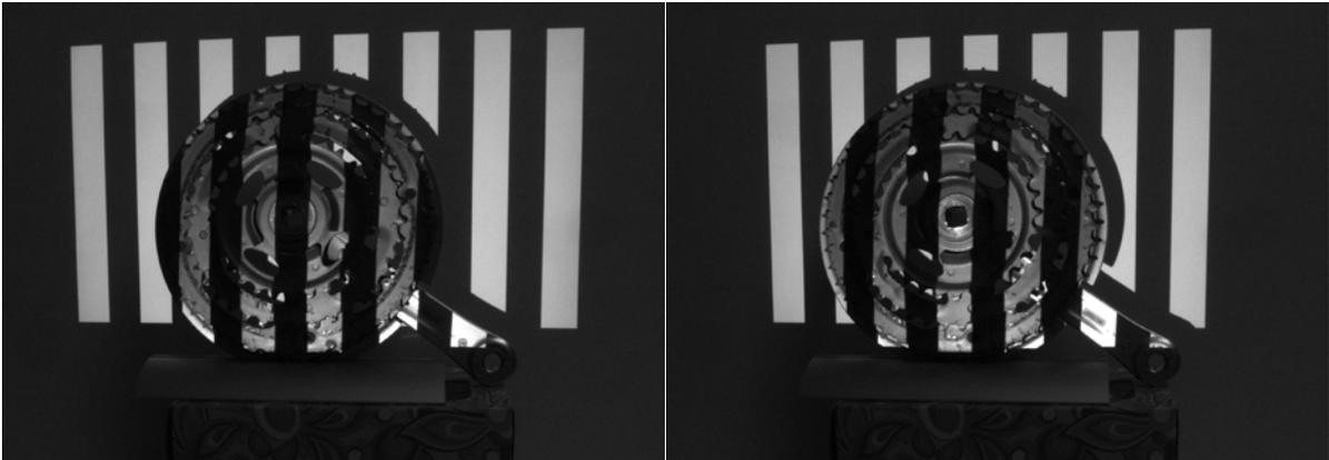
**Figure 18** Non-inverted and inverted vertical gray code pattern 5 capture
