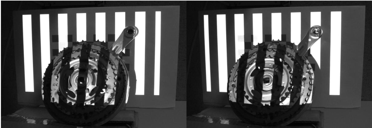
**Figure 40** Non-inverted and inverted vertical gray code pattern 5 capture
