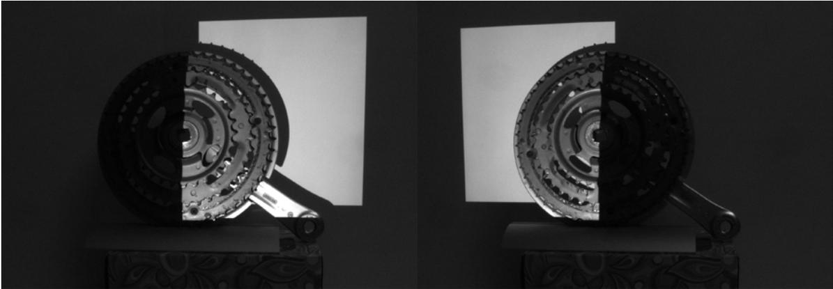
**Figure 14** Non-inverted and inverted vertical gray code pattern 1 capture
