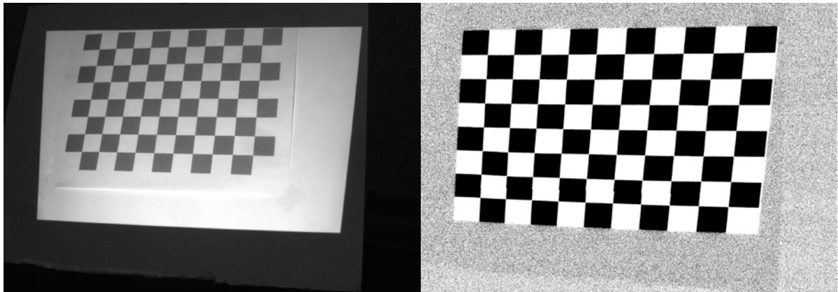
**Figure 4** Printed calibration board and projected calibration board position 3
