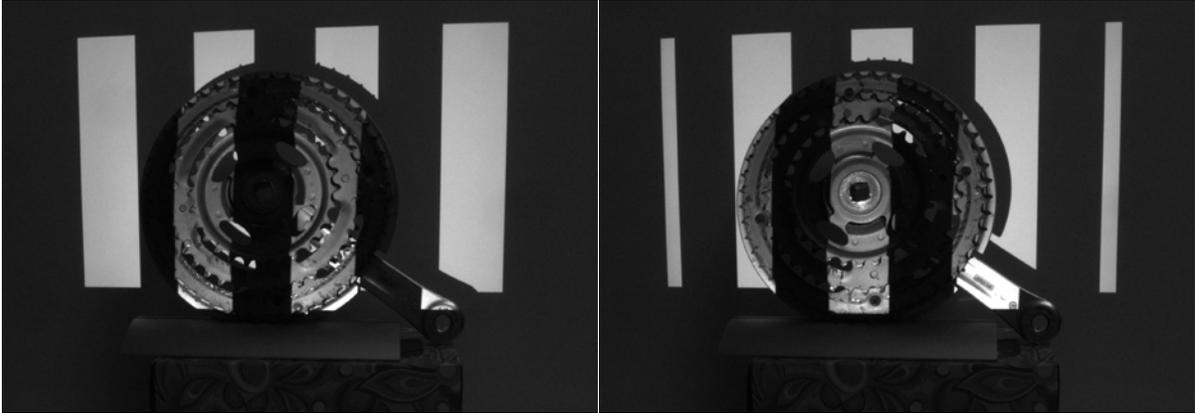
**Figure 17** Non-inverted and inverted vertical gray code pattern 4 capture
