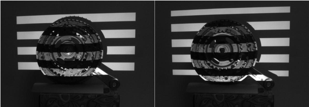
**Figure 27** Non-inverted and inverted horizontal gray code pattern 5 capture
