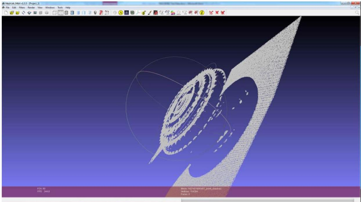
**Figure 34** Isometric view of point-cloud from 3D scan
