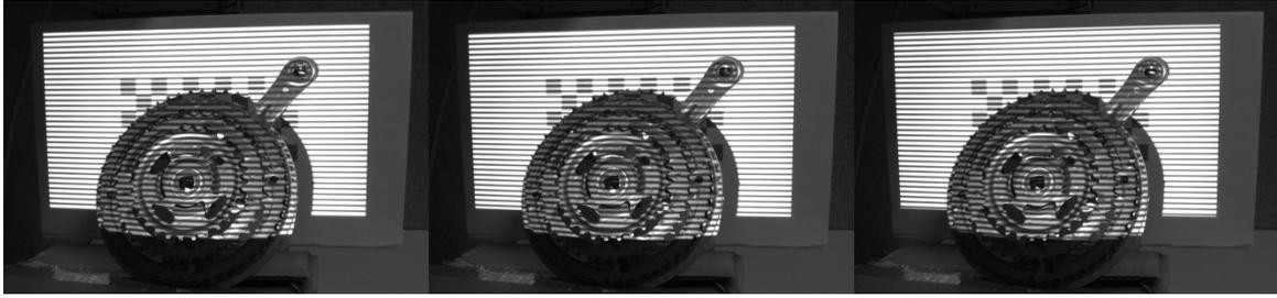
**Figure 45** Horizontal three phase patterns
