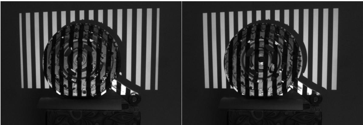
**Figure 19** Non-inverted and inverted vertical gray code pattern 6 capture
