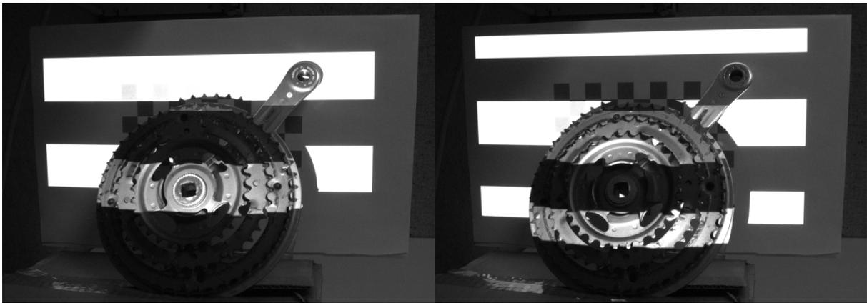
**Figure 49** Non-inverted and inverted horizontal gray code pattern 4 capture
