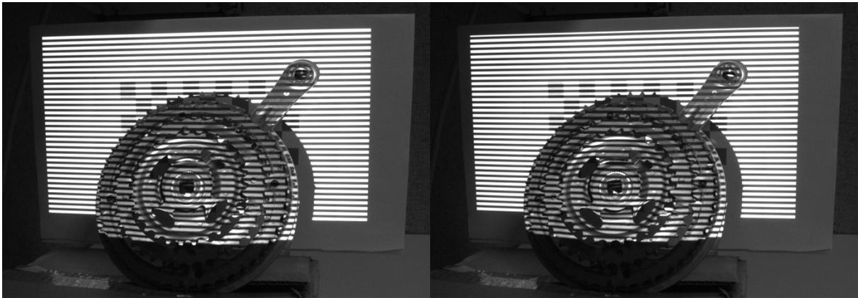
**Figure 53** Non-inverted and inverted horizontal gray code pattern 8 capture
