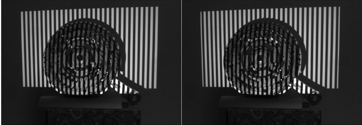
**Figure 20** Non-inverted and inverted vertical gray code pattern 7 capture
