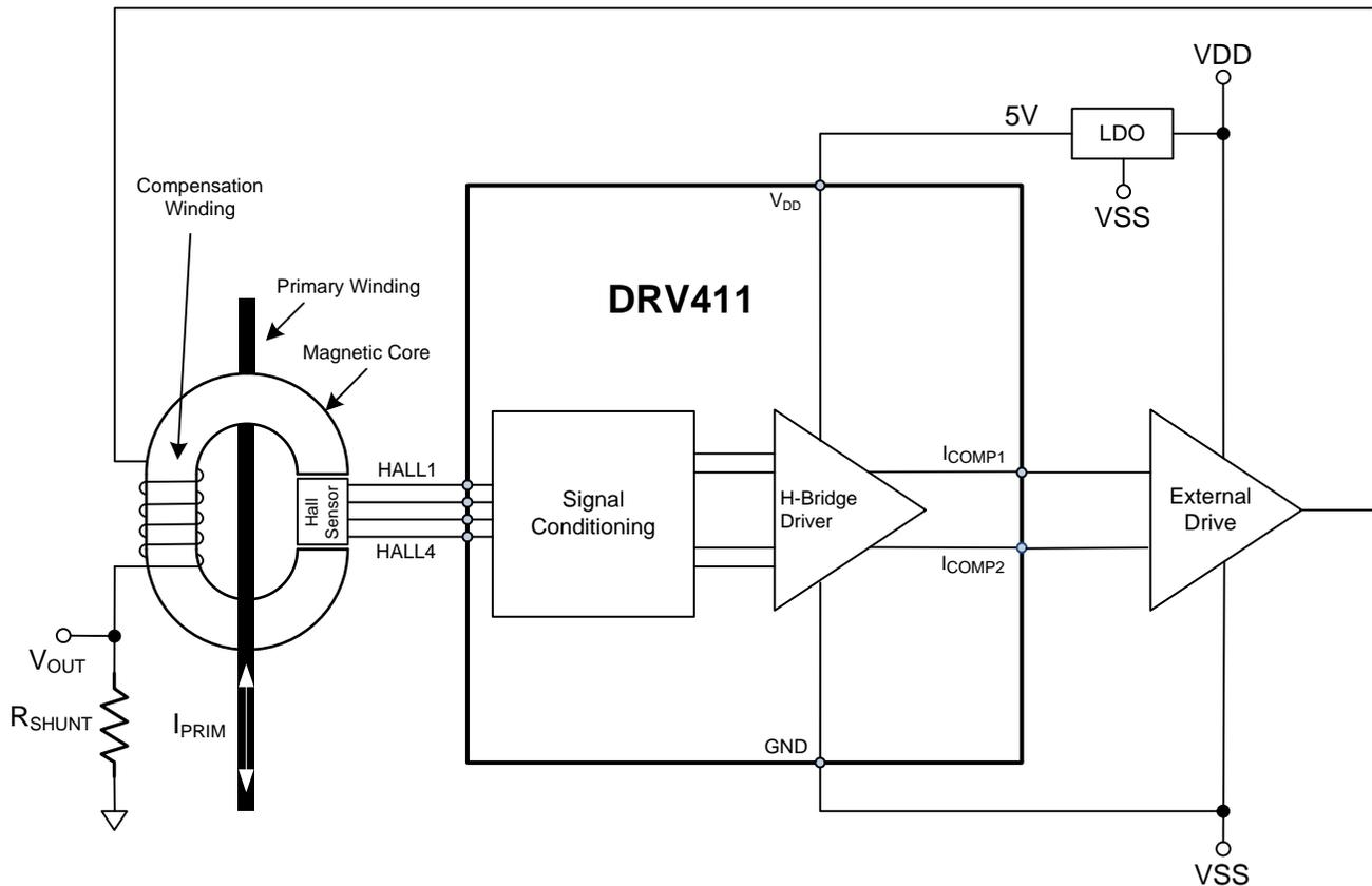
Figure 2: Closed-Loop Sensor Block Diagram
