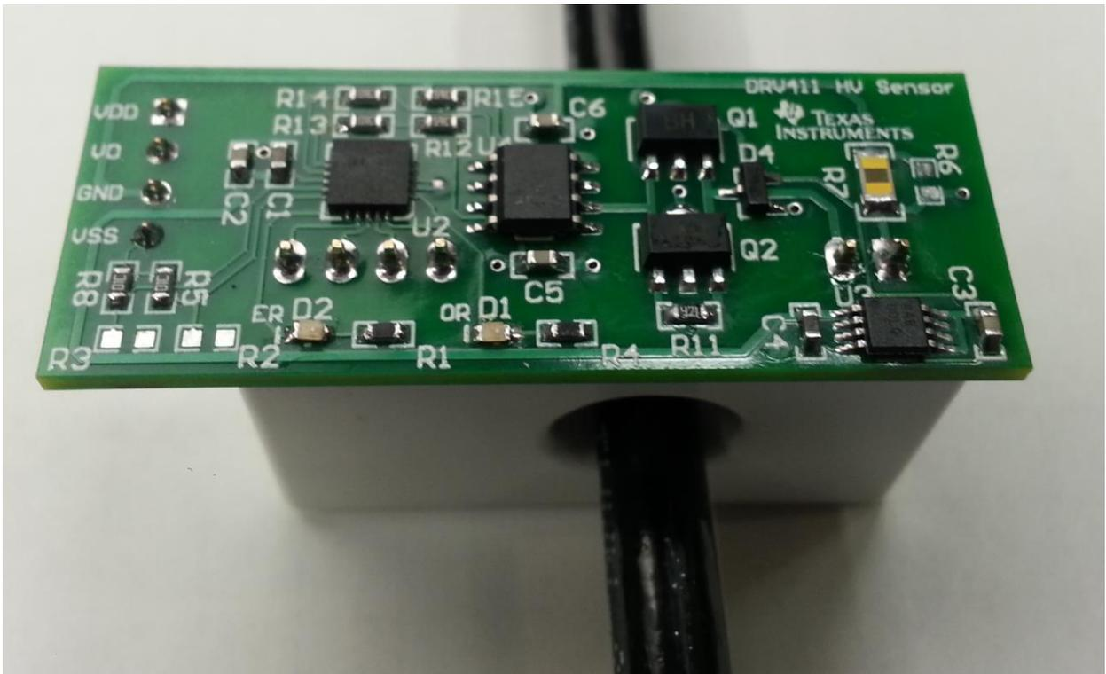
Figure 4: Primary Winding, Sensor and PWB
