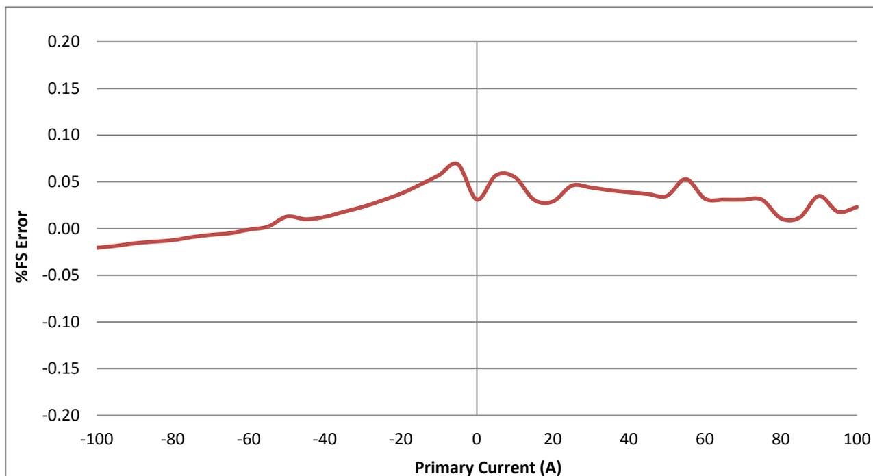
**Figure 6: Full-Scale Error vs. Input Current**
