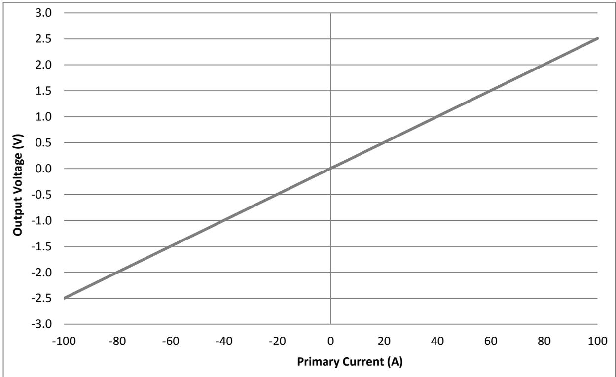
**Figure 5: DC Transfer Function ( $V_{OUT}$  vs.  $I_p$ )**
