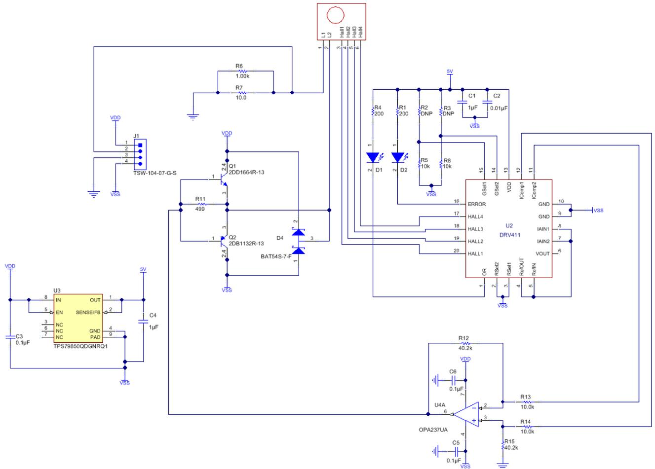
Figure A-1: Electrical Schematic
