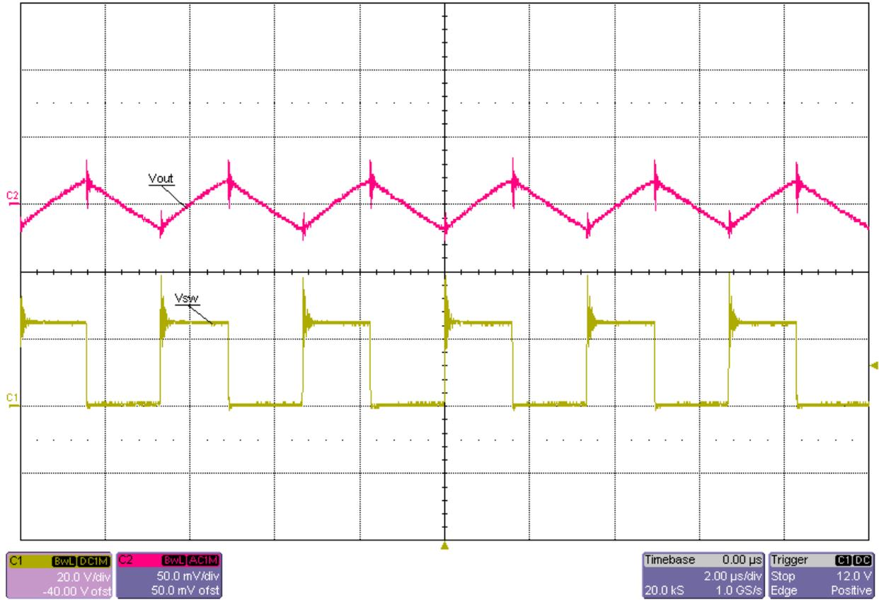
Output Voltage Ripple and Switch Node Voltage at 12Vin 0.25A load on each output (Vripple ≈ 40mVp-p)
