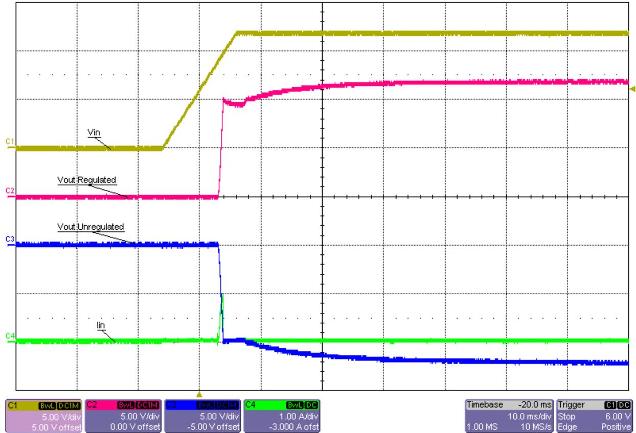
**Startup into No Load (12Vin)**
