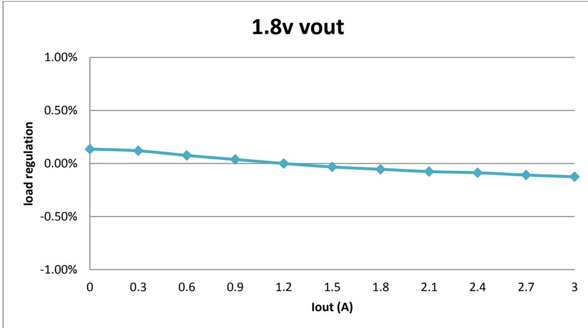
Figure 9. VIN = 12V, VCCAUX Load Regulation
