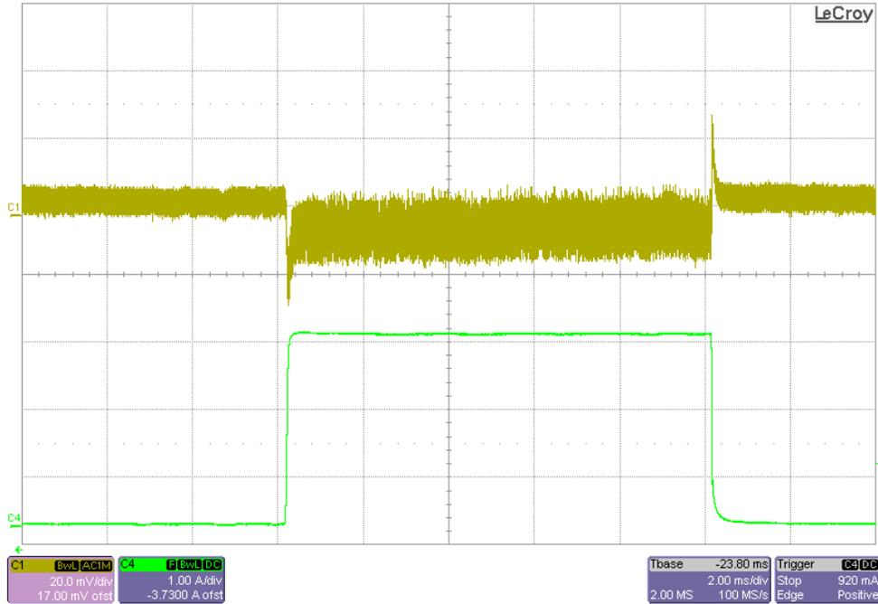
Figure 12. VIN = 12V, VCCINT Load Transient      slew rate=1A/us
