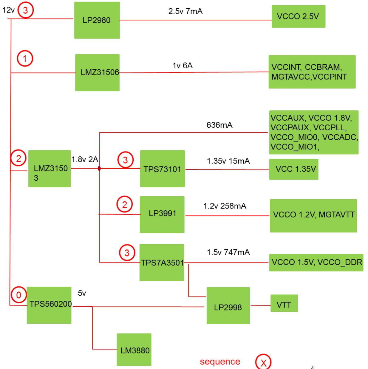
Figure 1. Block Diagram
