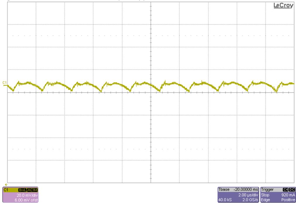
Figure 11. VIN = 12V, VCCAUX Output Ripple @ IOOUT = 3A
