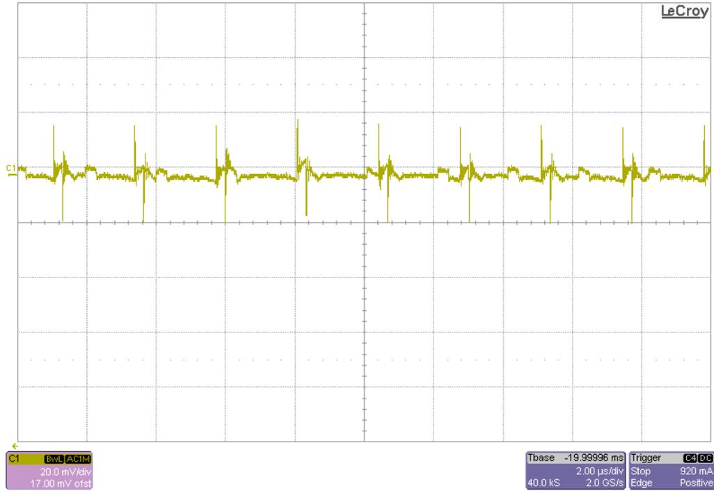
Figure 10. VIN = 12V, VCCINT Output Ripple @ IOOUT = 3A
