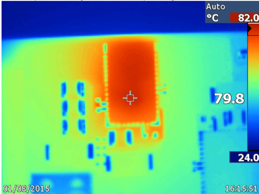
Figure 14. VIN = 12V, VCCINT Thermal Image @ Full Load
