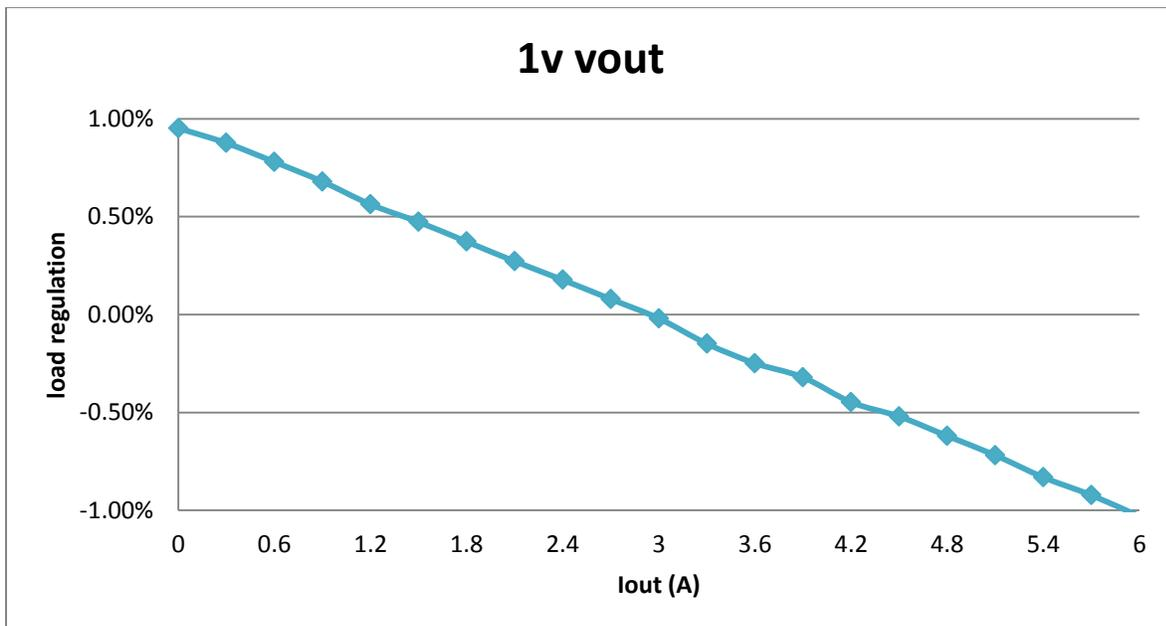
Figure 8. VIN = 12V, VCCINT Load Regulation
