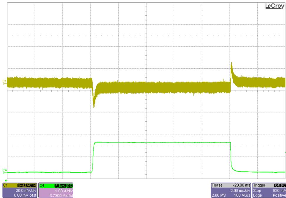
Figure 13. VIN = 12V, VCCAUX Load Transient      slew rate=1A/us
