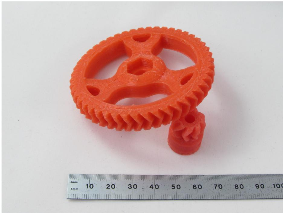
**Figure 20: 3D Printed Gears**
