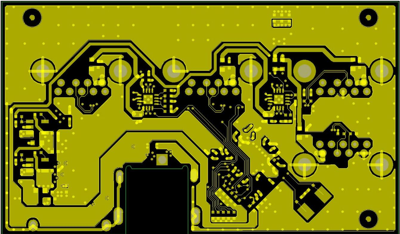
Figure 9. Bottom Side - Routing
