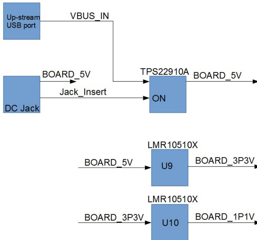
Figure 5. Power Sub-System Block Diagram
