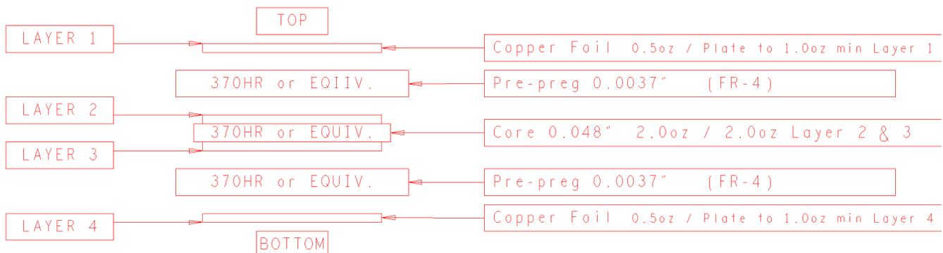
Figure 12. PCB Stack-up
