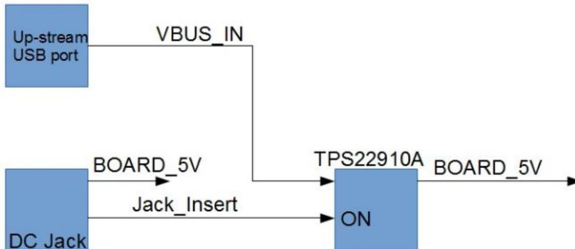
**Figure 2. 5 V Power Switching**
