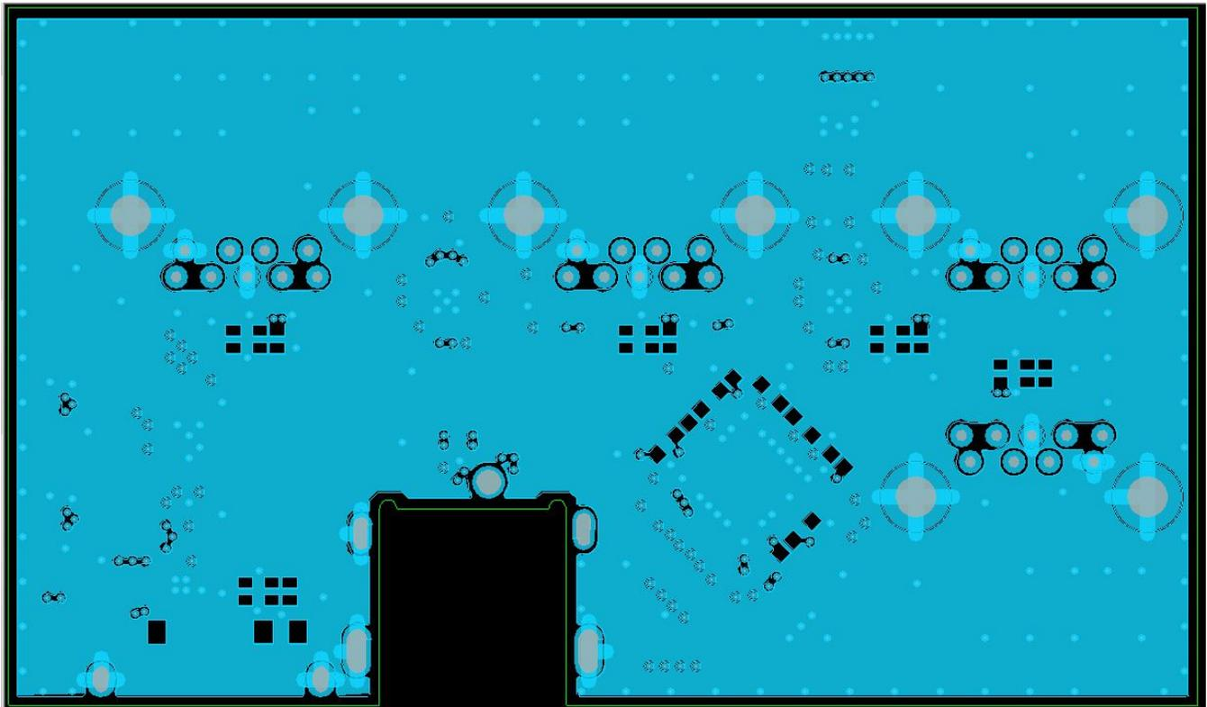
Figure 7. Layer 2 – Ground Plane
