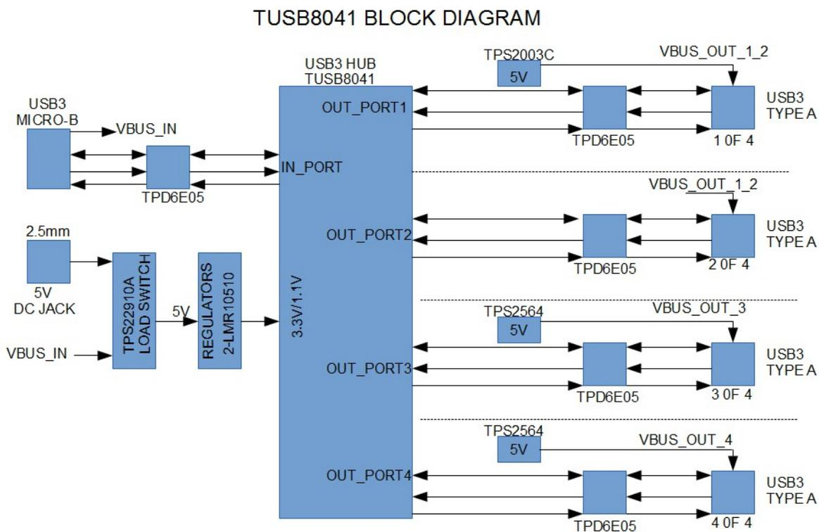
Figure 1. TUSB8041 Functional Block Diagram
