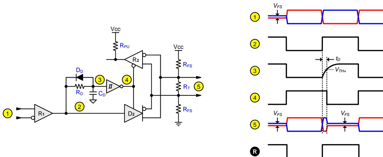
**Figure 3. Data flow-control principle (left) with timing diagram (right)**
