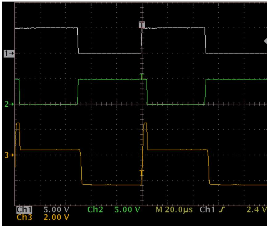
Figure 4. Data flow-control: Ch1 = D, Ch2 = DE, /RE, Ch3 =  $V_{BUS}$
