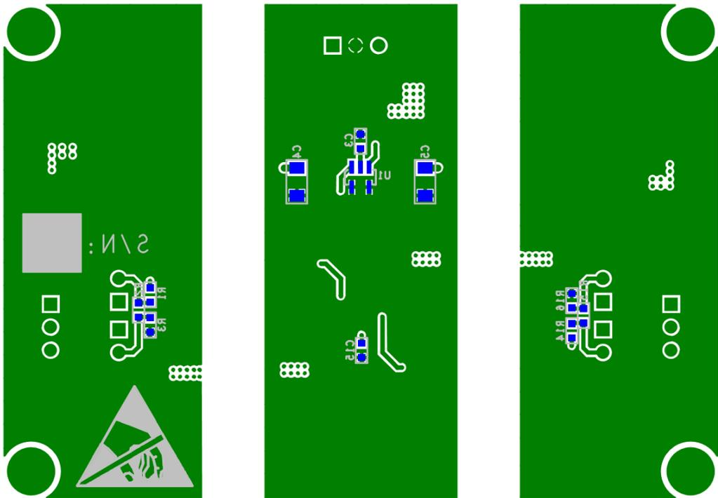
Figure 9: PCB layout bottom
