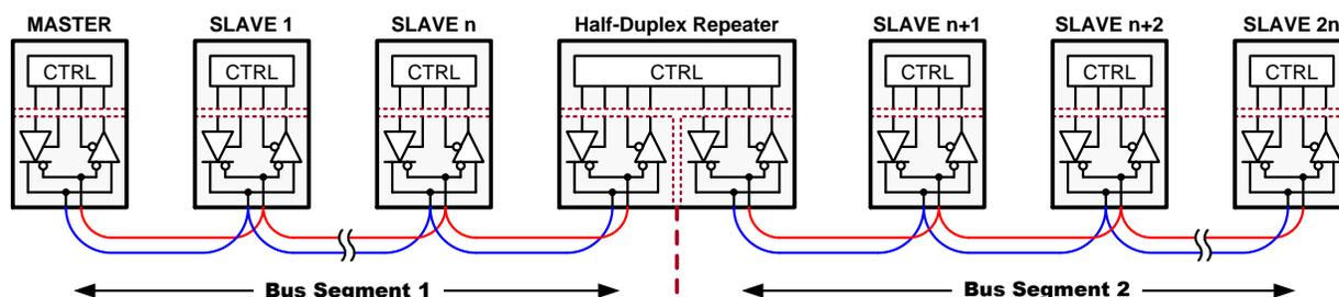
Figure 1. Simplified diagram of a two-segment long-haul network
