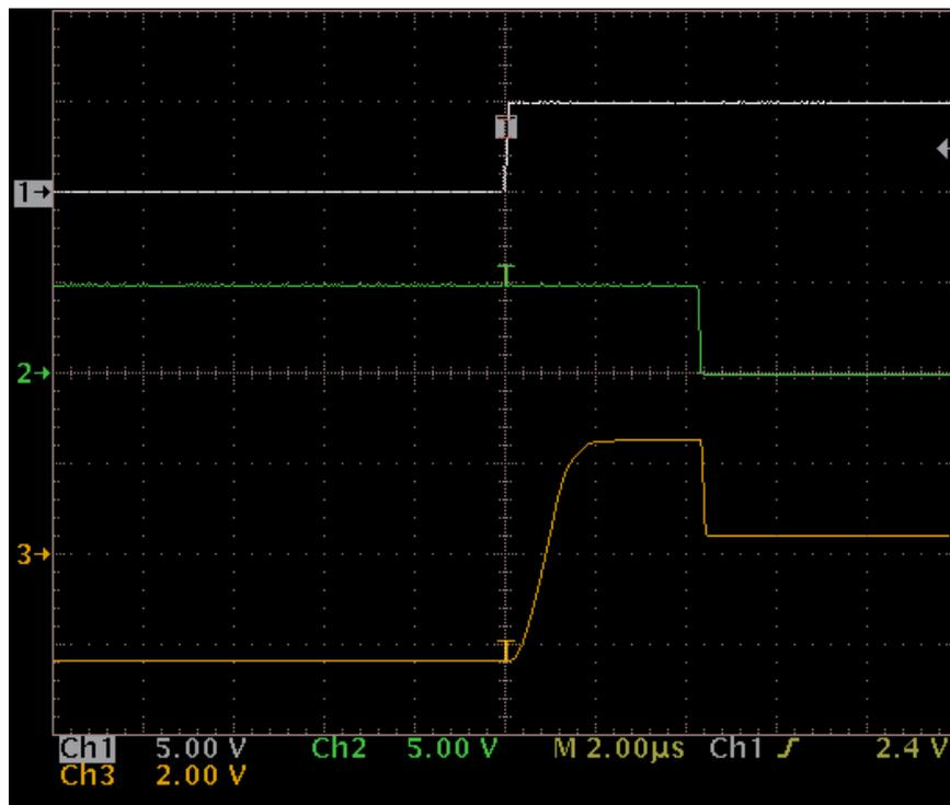
Figure 5. Data flow-control zoomed-in: Ch1 = D, Ch2 = DE, /RE, Ch3 =  $V_{BUS}$
