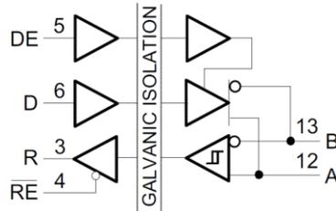
**Figure 2: ISO3082 functional block diagram**
