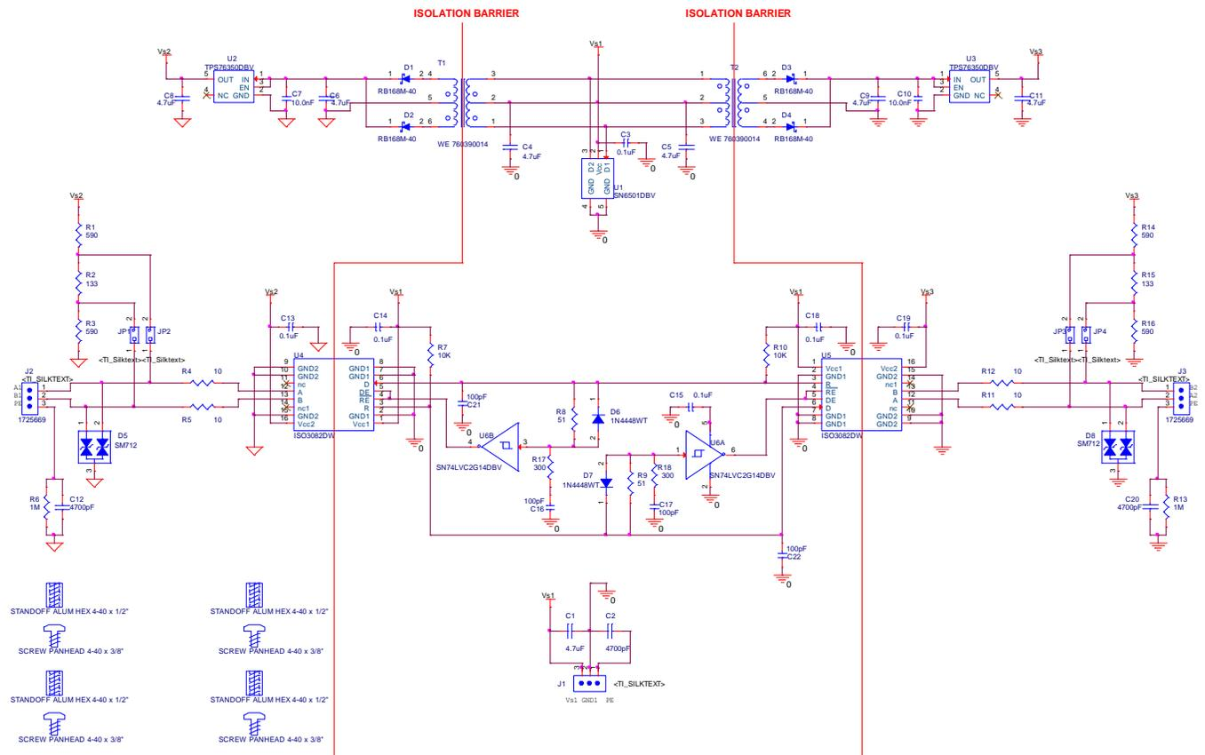
Figure 10: Dual isolated half-duplex RS-485 repeater
