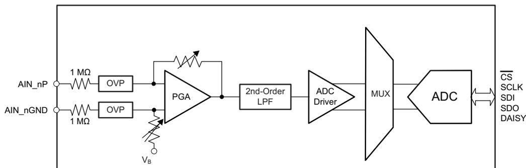
**Figure 3. Front-End Circuit Schematic for Each Analog Input Channel**
