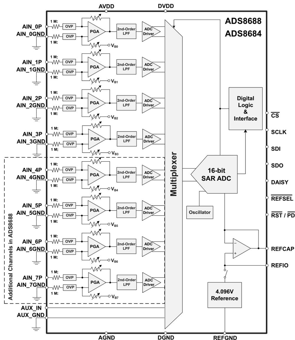
Figure 2. Internal Block Diagram of ADS8684
