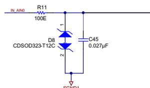
Figure 22. Analog Input EMC Protection
