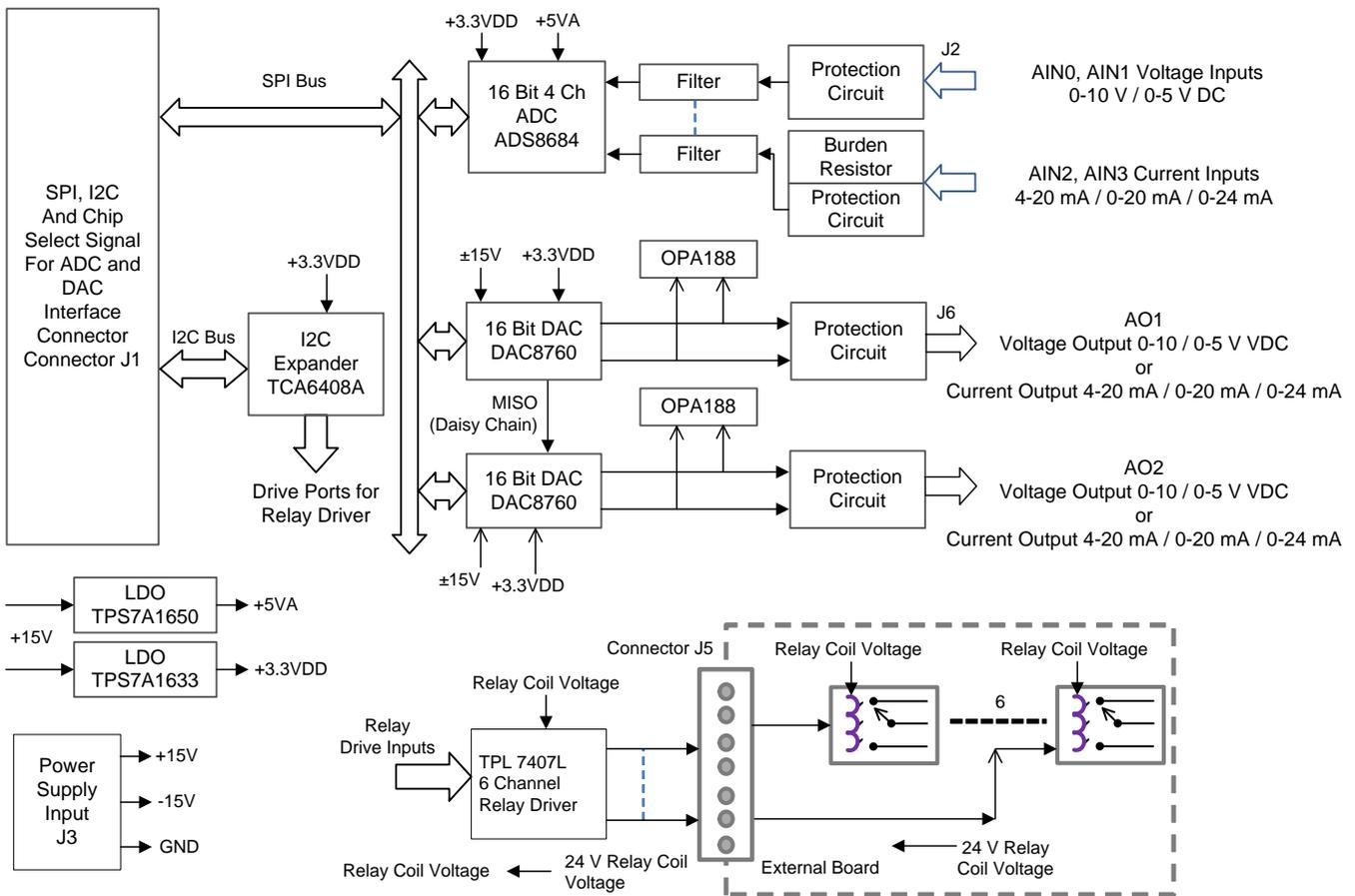
Figure 1. Block Diagram of TIDA-00310
