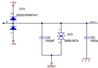
**Figure 23. Analog Output EMC Protection**
