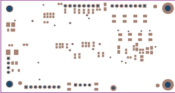
**Figure 49. Bottom Solder Mask**
