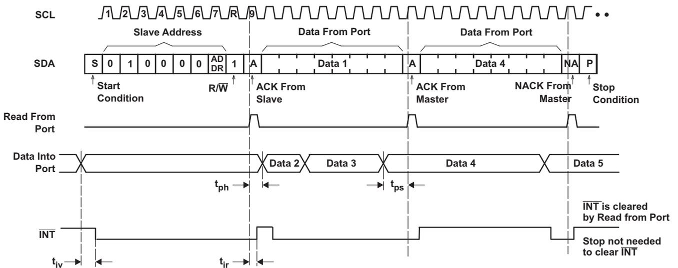
Figure 30. Read From Input Port Register
