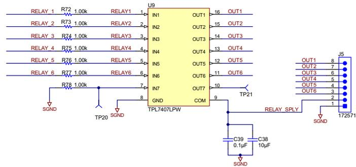
**Figure 17. Digital Output Relay Driver**
