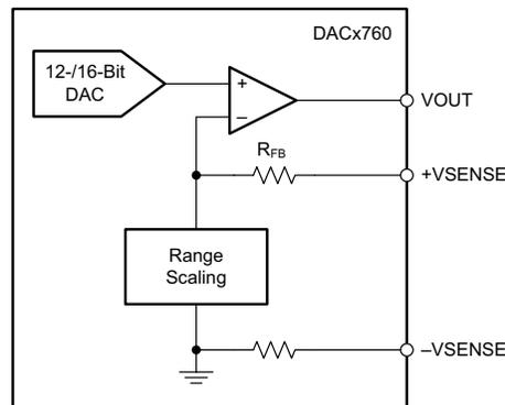
**Figure 9. Voltage Output**
