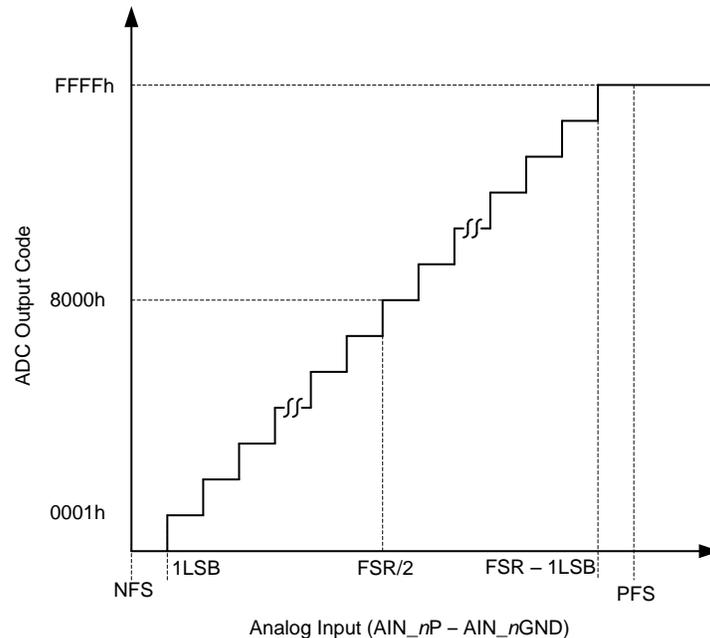
**Figure 24. ADC Transfer Function**
