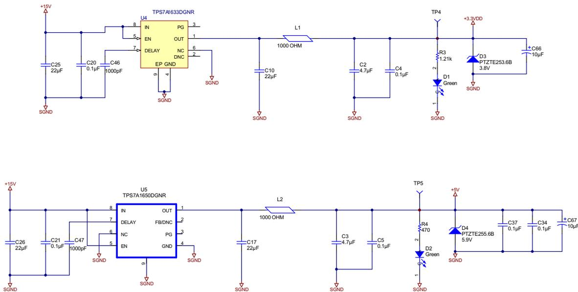
Figure 19. Digital Power Supply 3.3 V and Analog Power Supply 5.0-V Regulators
