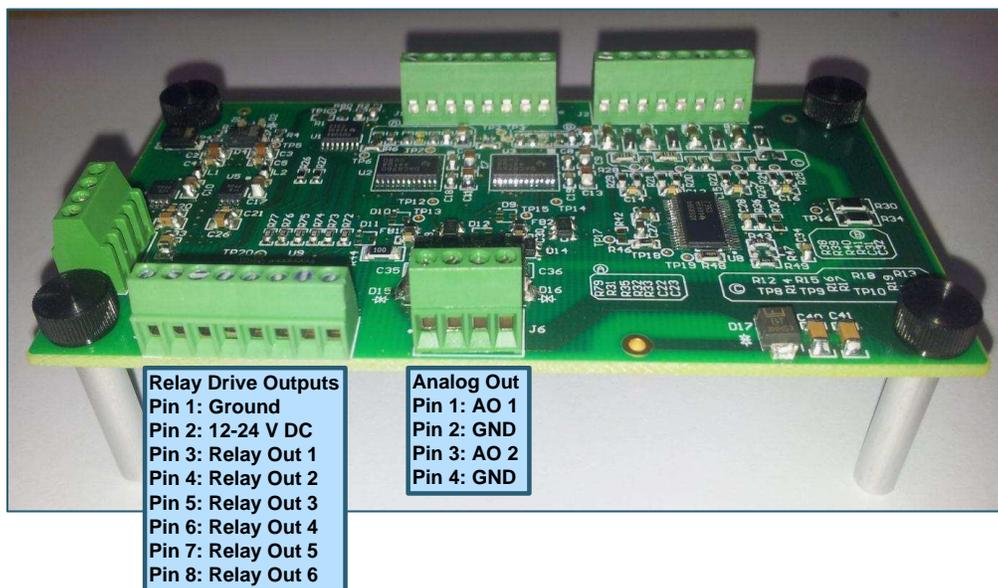
Figure 36. Connector Details Relay Drive Outputs and Analog Outputs
