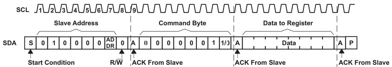
**Figure 28. Write to Configuration or Polarity Inversion Registers**
