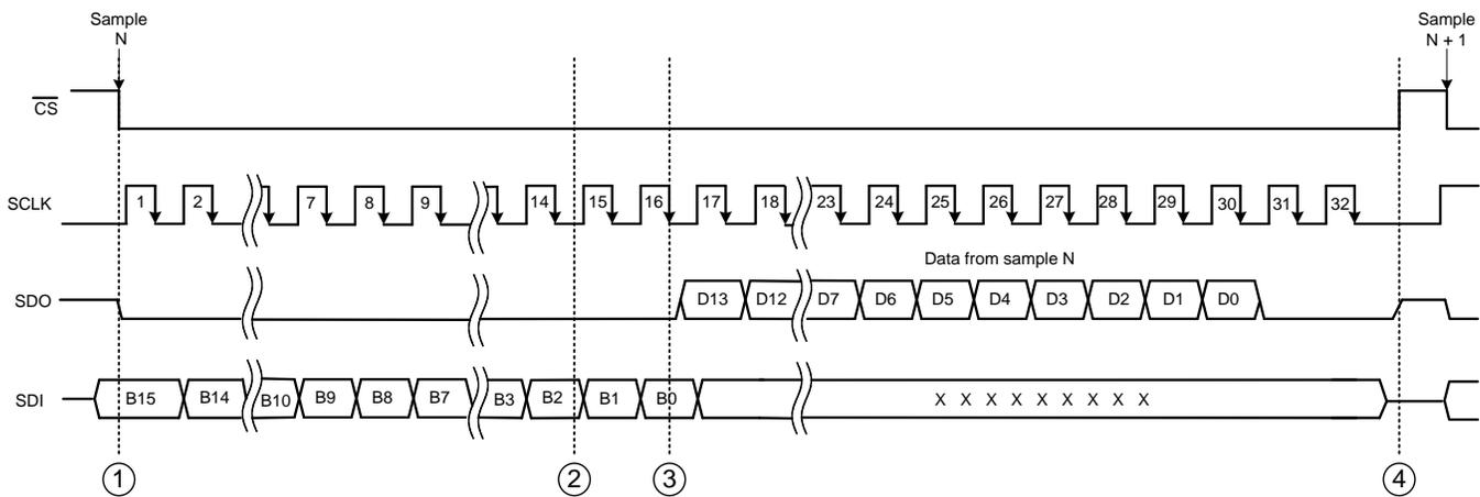
**Figure 25. Device Operation Using the Serial Interface Timing Diagram of ADS8684**
