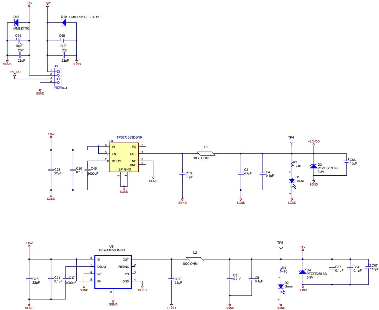
Figure 40. Digital Power Supply and Analog Power Supply Schematic
