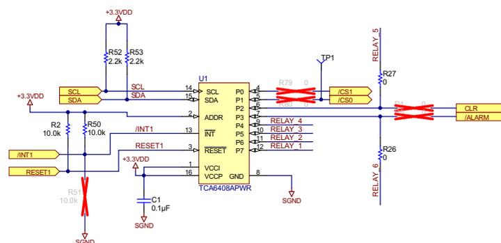
Figure 39. Digital Output and DAC Interface Schematic
