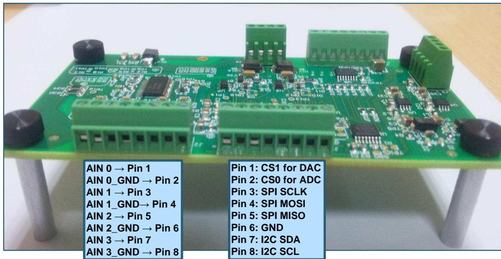
Figure 37. Connector Details Analog Input and Interface Connector
