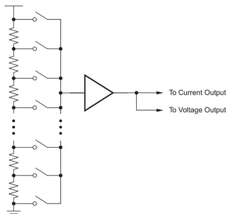
**Figure 8. DAC Structure: Resistor String of DAC8760**
