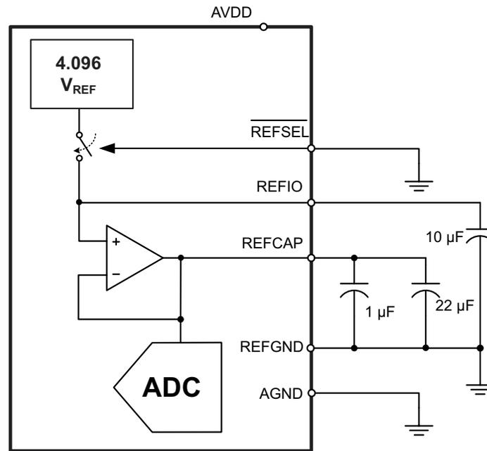
**Figure 4. Device Connections for Using an Internal 4.096-V Reference**
