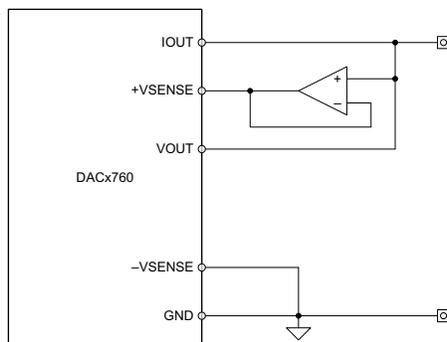
**Figure 12. VOUT and IOUT Tied Together to One Terminal**
