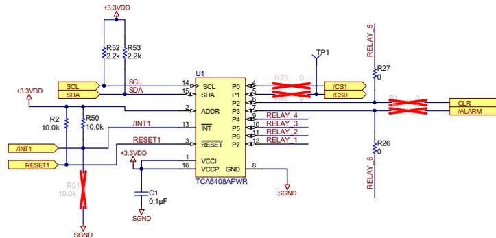
**Figure 16. I2C I/O Expander**
