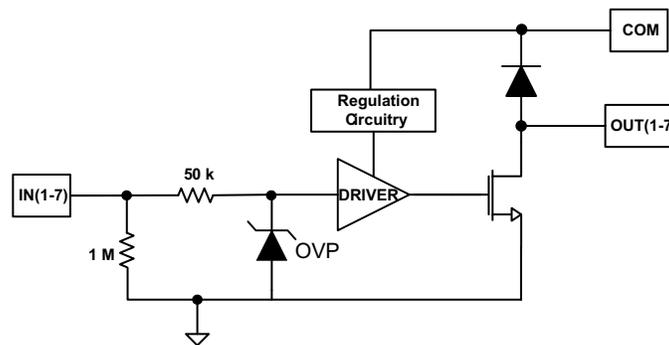
**Figure 14. TPL7407L Functional Block Diagram**
