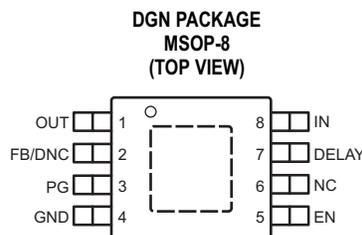
**Figure 18. Pin Configuration TPS7A1633**
