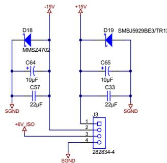
Figure 20. Front End Power Supply Connector and Filter
