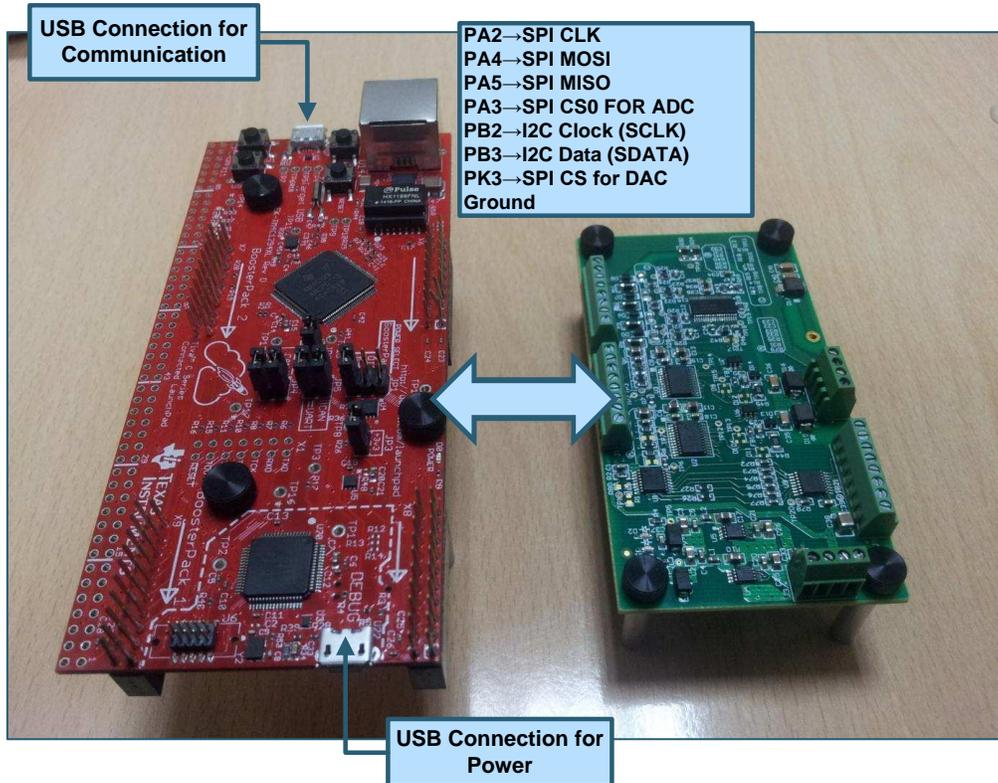
Figure 35. Connection With Host Controller
