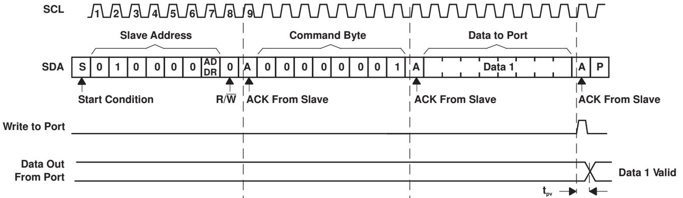
**Figure 27. Write to Output Port Register**
