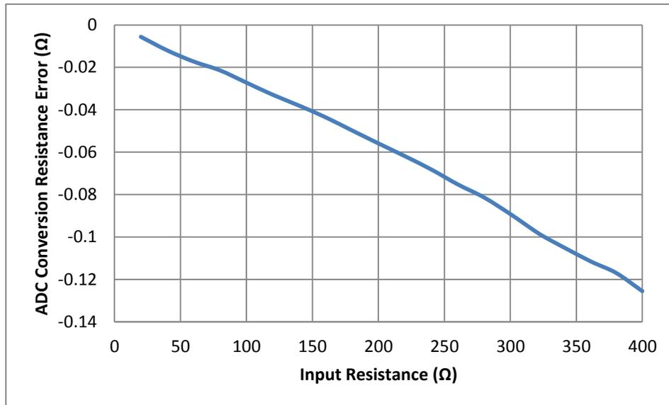
**Figure 27: Measured Resistance Error with Precision Resistor Input**
