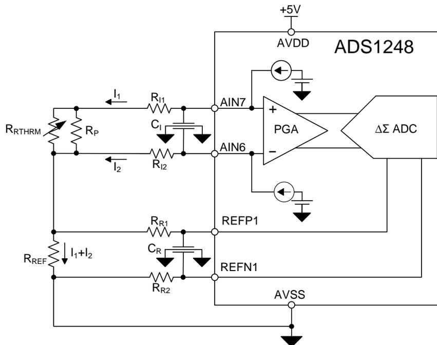
**Figure 5: Thermistor Input Circuitry**
