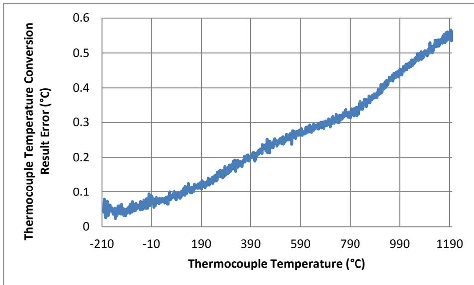
Figure 18: Measured Thermocouple Temperature Error
