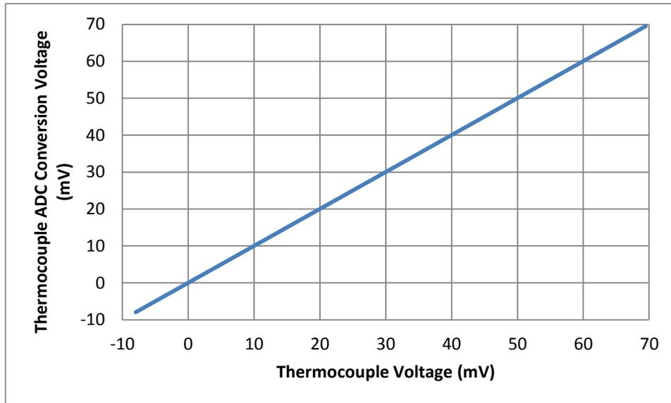
**Figure 15: Measured Thermocouple Input Circuitry Transfer Function**
