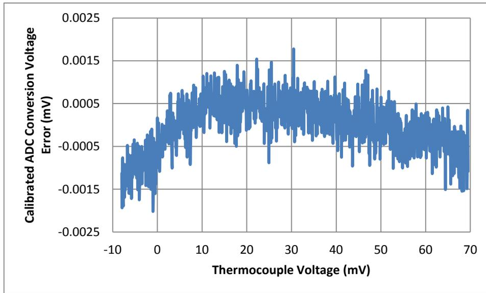
Figure 17: Calibrated Thermocouple Voltage Error
