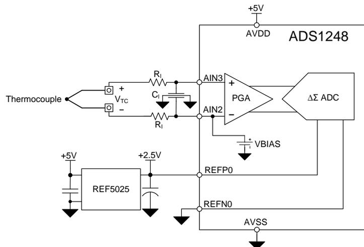
Figure 4: Thermocouple Input Circuitry
