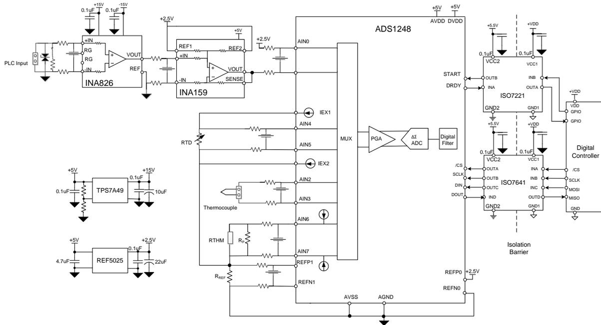
**Figure 2: Detailed Analog Input Schematic**
