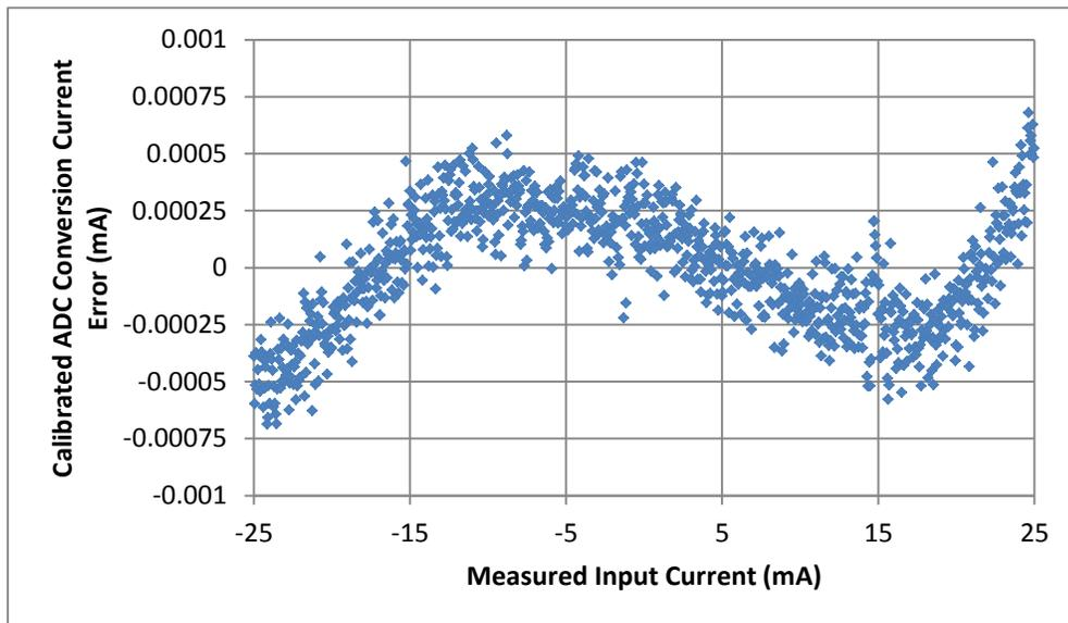
**Figure 14: Calibrated Industrial Current Input Error**
