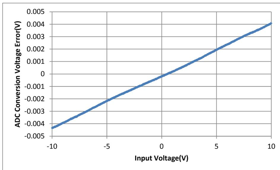
**Figure 10: Measured Industrial Voltage Input Error**
