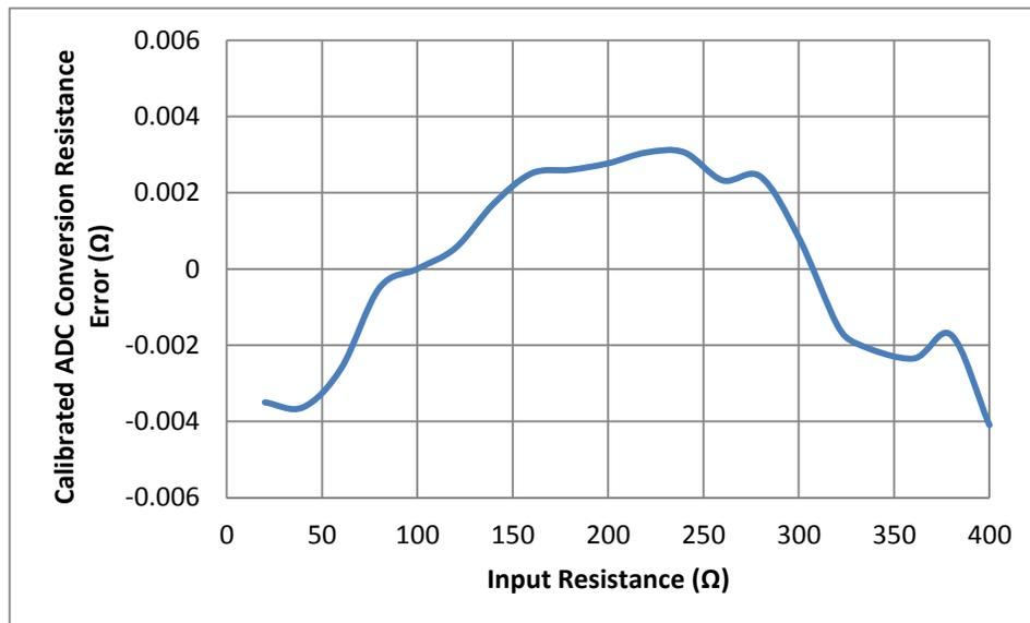
**Figure 28: Calibrated RTD Input Circuitry Error**
