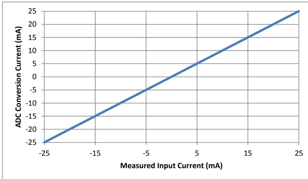
Figure 12: Measured Industrial Current Input Transfer Function
