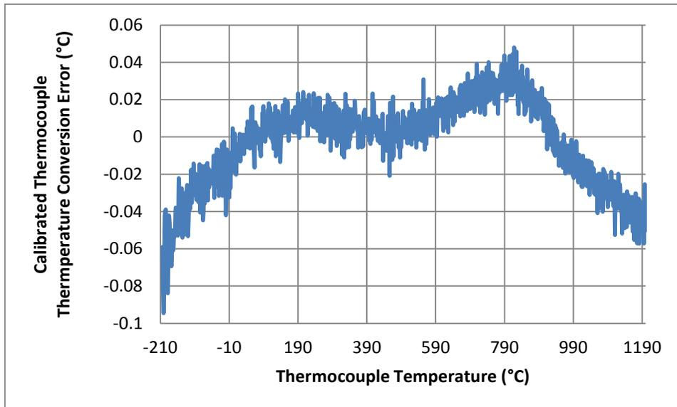
**Figure 19: Calibrated Thermocouple Temperature Error**
