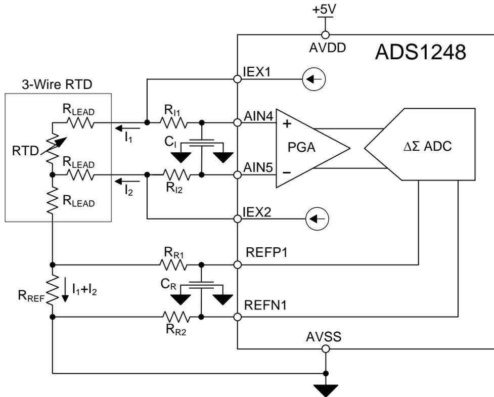
**Figure 6: Ratiometric 3-Wire RTD Input Circuitry**
