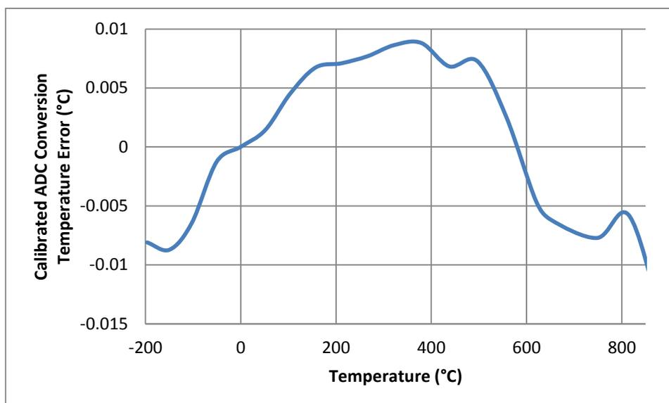
**Figure 29: Calibrated RTD Input Circuitry Temperature Error**
