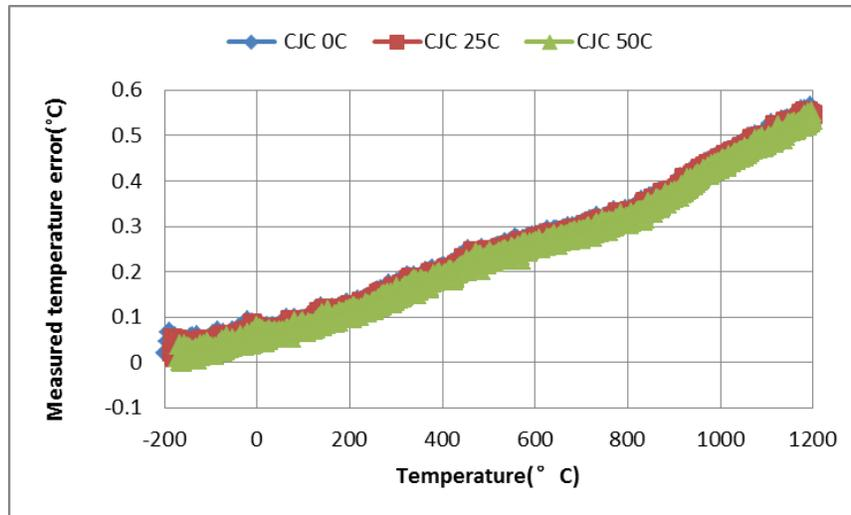
Figure 25: Thermocouple Temperature Error with CJC
