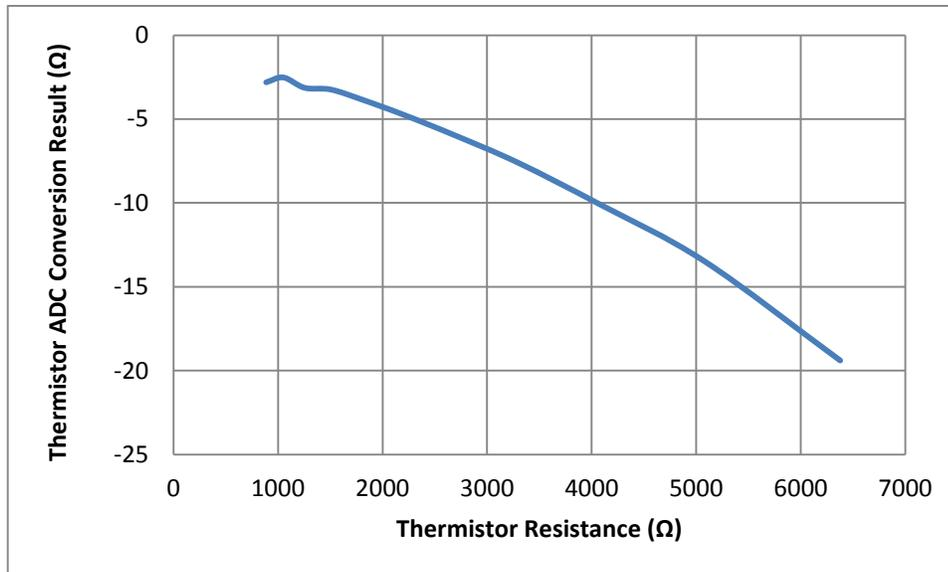
Figure 21: Measured Thermistor Input Circuitry Error
