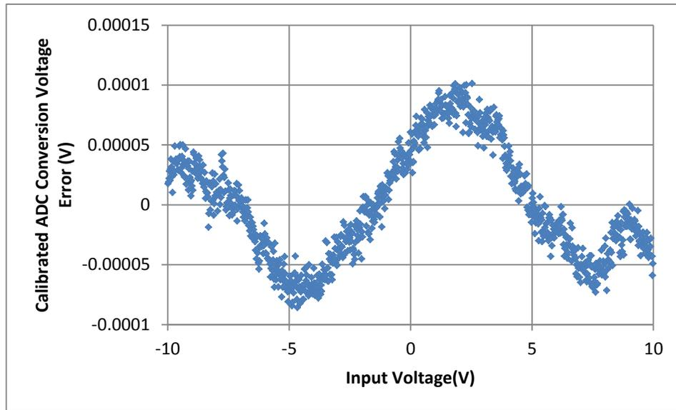
Figure 11: Measured Calibrated Industrial Voltage Input Error
