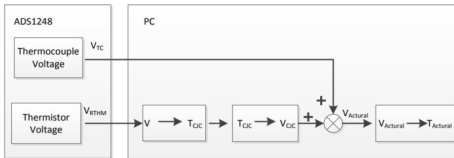
**Figure 24: Software Flow Block Diagram**
