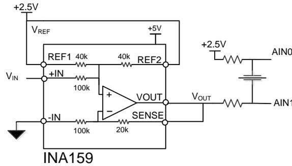
**Figure 7: Detailed INA159 Circuitry**
