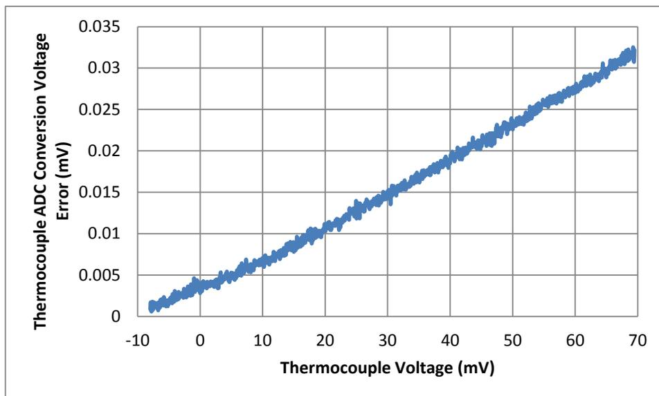
**Figure 16: Measured Thermocouple Voltage Error**
