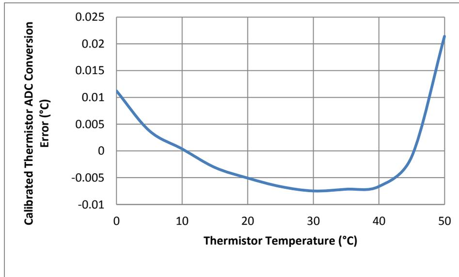
**Figure 23: Calibrated Thermistor Input Temperature Error**
