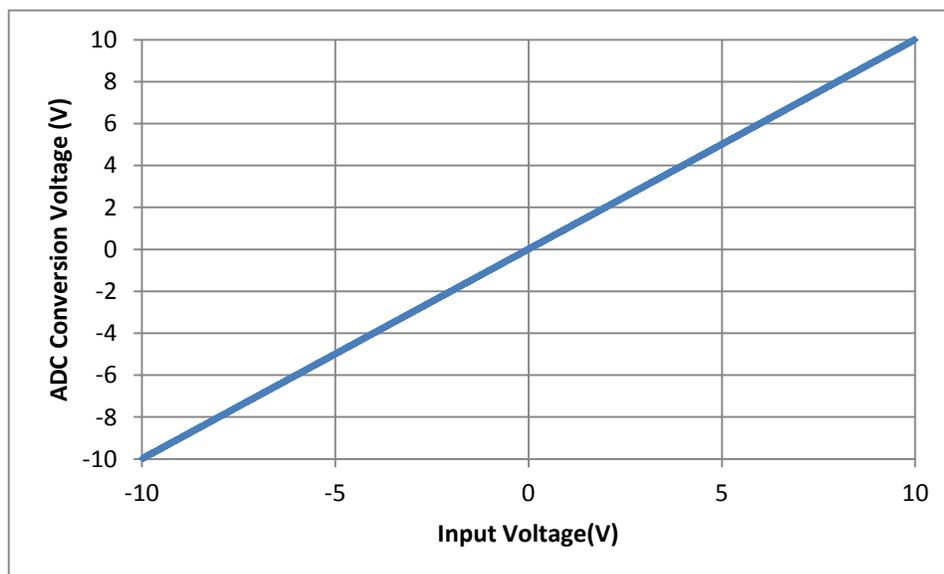
**Figure 9: Measured Industrial Voltage Input Transfer Function**
