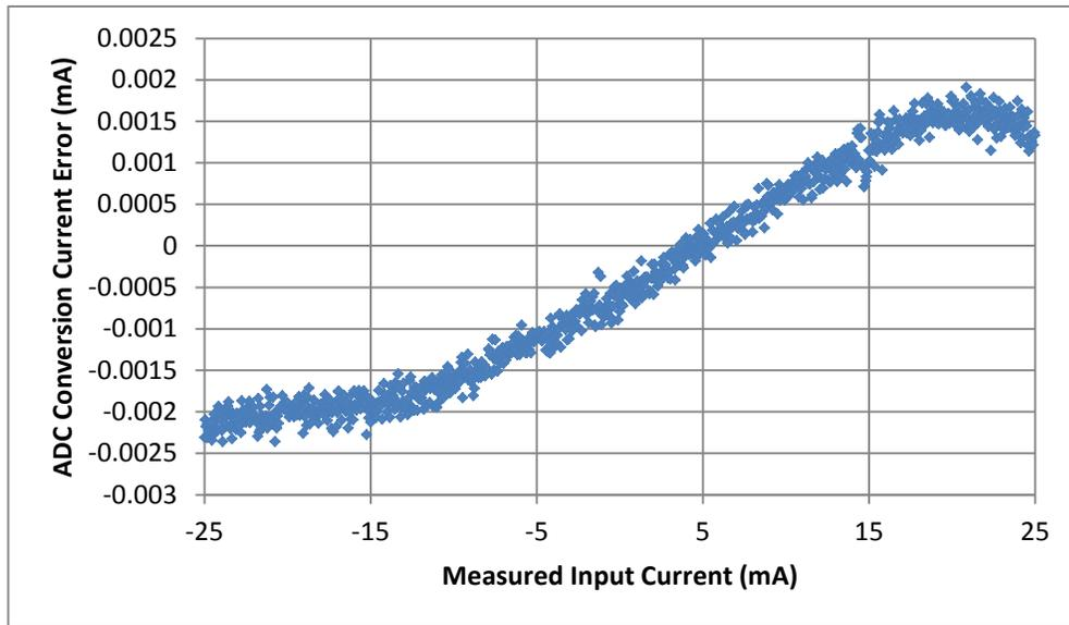
**Figure 13: Measured Industrial Measured Input Error**
