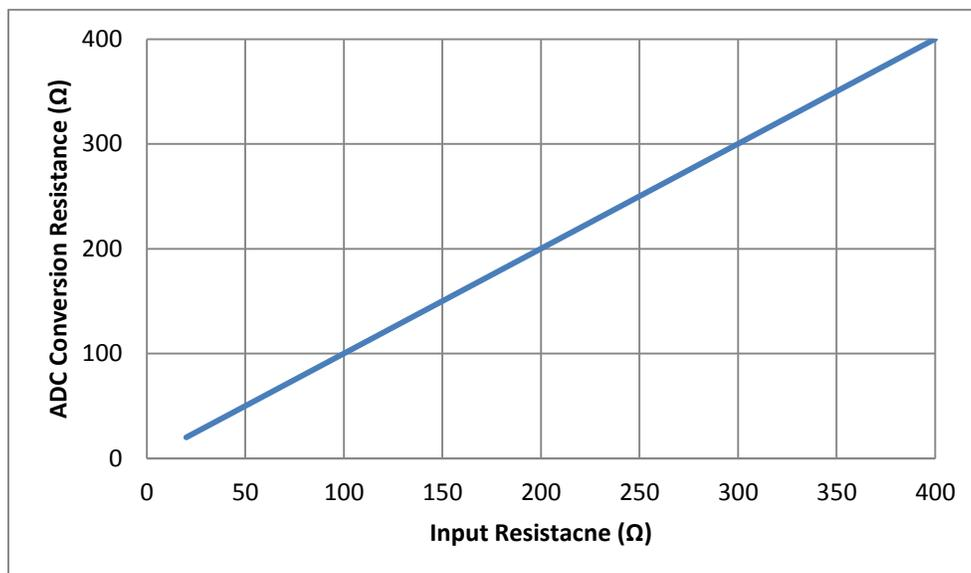
Figure 26: Measured Resistance Results with Precision Resistors
