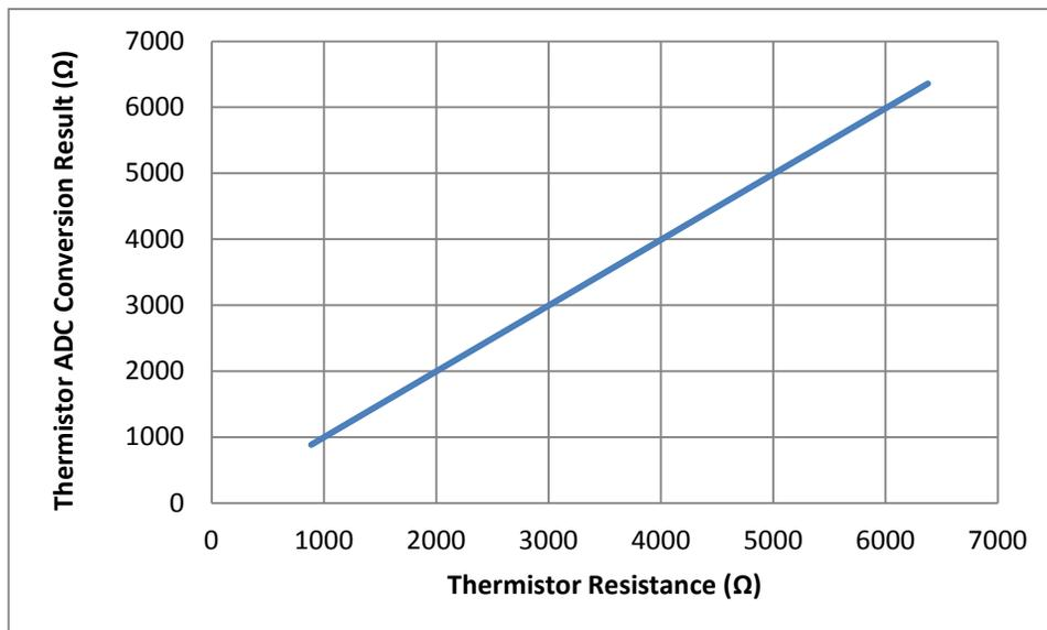
**Figure 20: Measured Thermistor Input Transfer Function**
