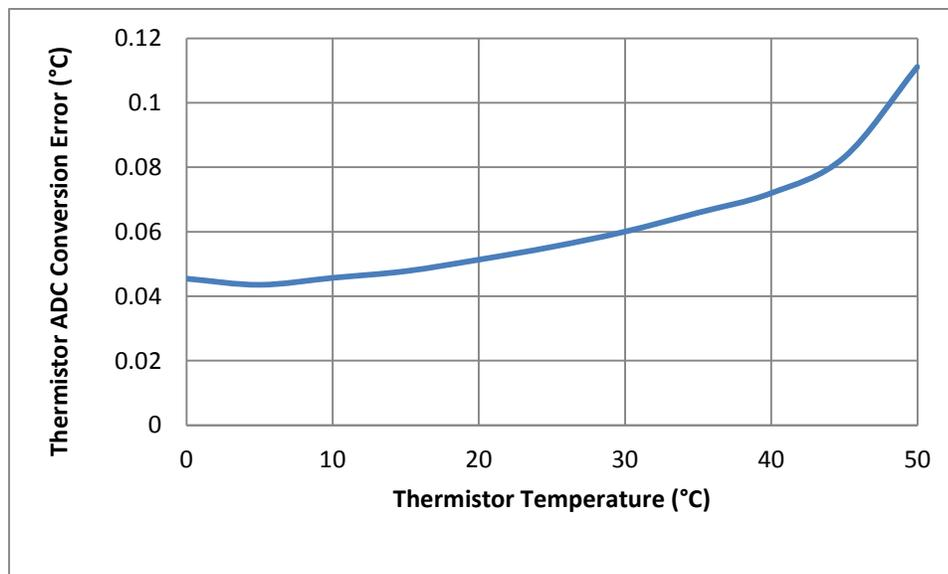
Figure 22: Measured Thermistor Input Circuitry Temperature Error
