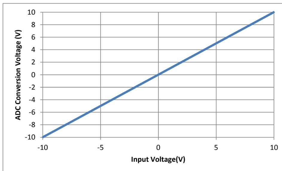
**Figure 1: Measured Industrial Voltage Input Results**
