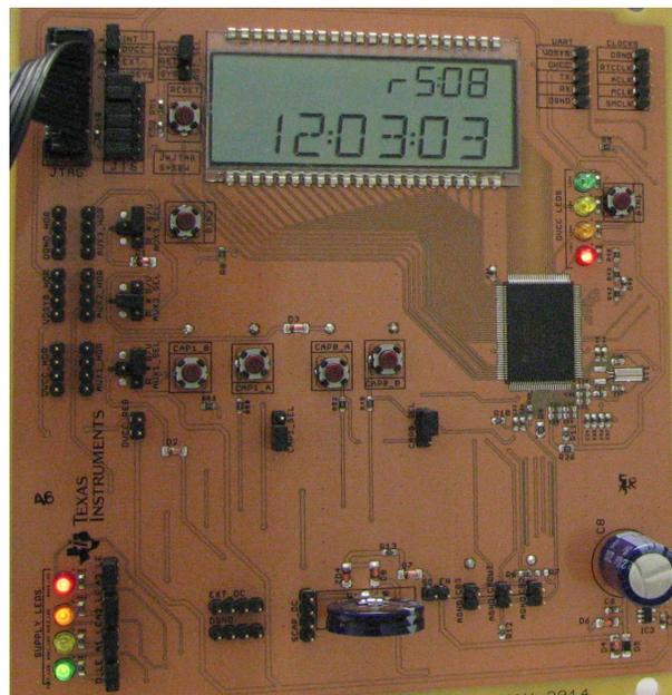
**Figure 17. AUX12 Code Example: Chip Powered from DVCC Again; Previously Reset Due to LPM3.5 Exit**
