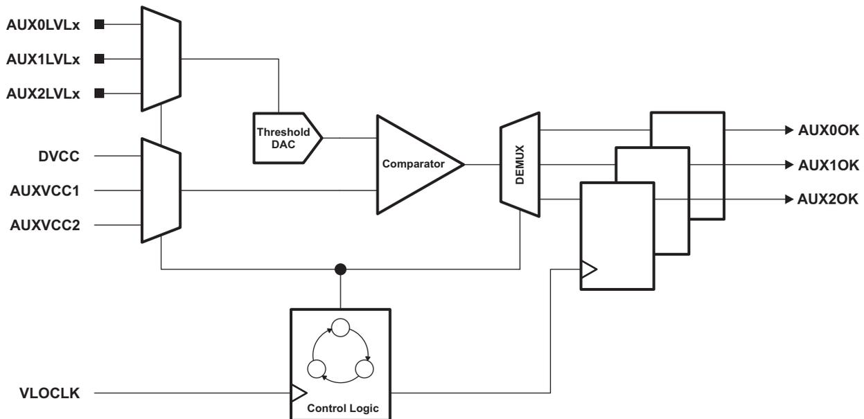
Figure 2. Auxiliary Supply Monitor Block Diagram
