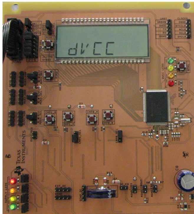
Figure 6. AUX01 Code Example: Chip Powered from DVCC
