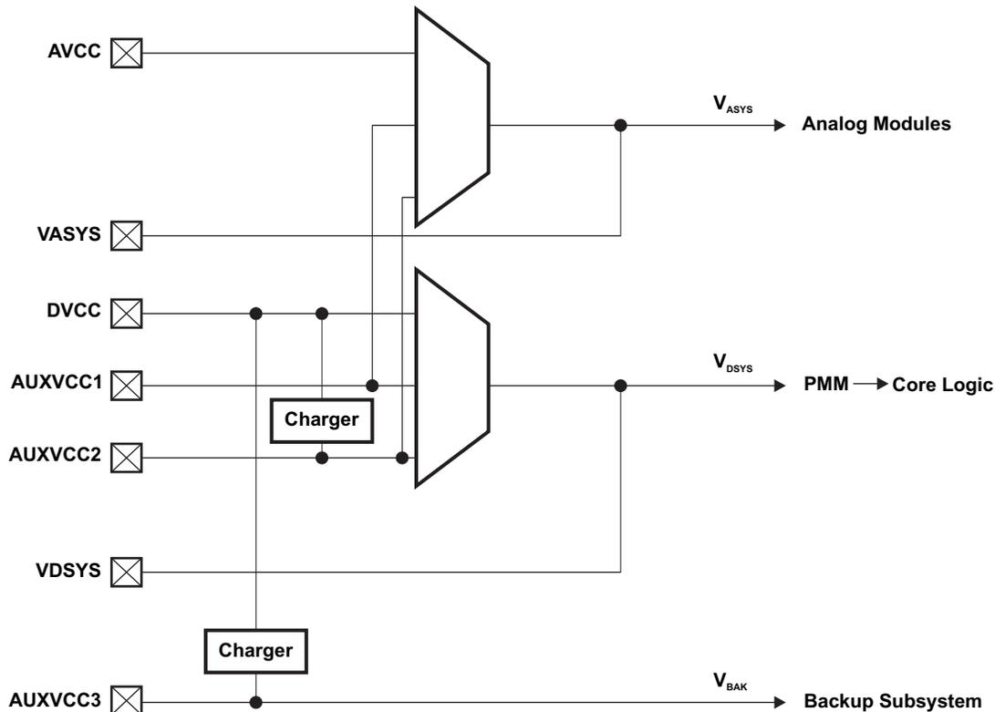
**Figure 1. AUX Module Functional Block Diagram**
