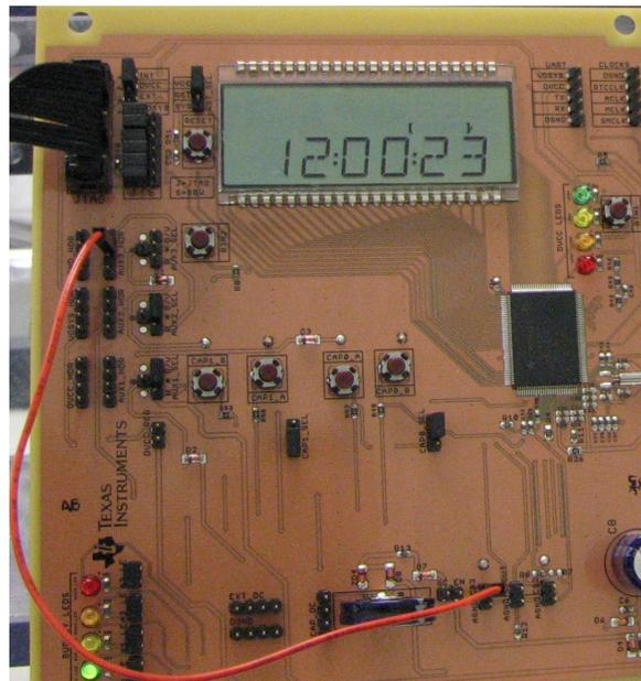
Figure 12. AUX07 Code Example: AUXVCC3 Voltage Falls Below 2.5-V Threshold
