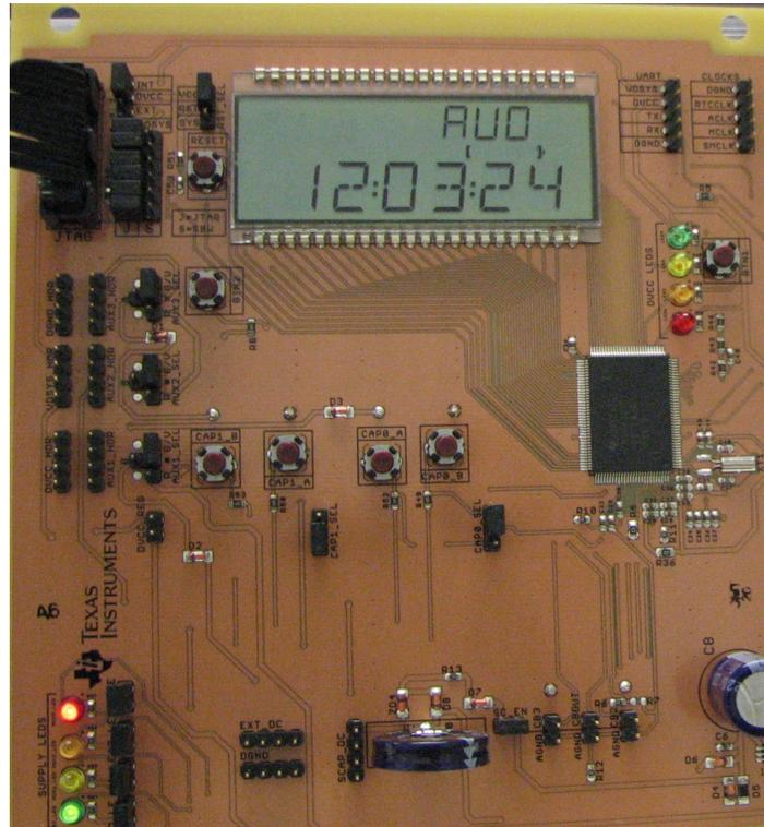
**Figure 11. AUX03 Code Example: Chip Supply Switched Back to DVCC; AUXVCC1 and AUXVCC2 Invalid**
