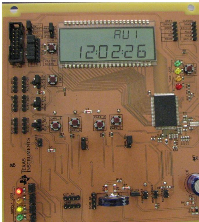
**Figure 10. AUX03 Code Example: Chip Being Powered from AUXVCC1**
