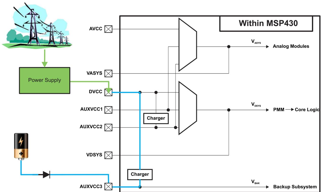
Figure 3. AUX Configuration for RTC-Only Back-Up Power
