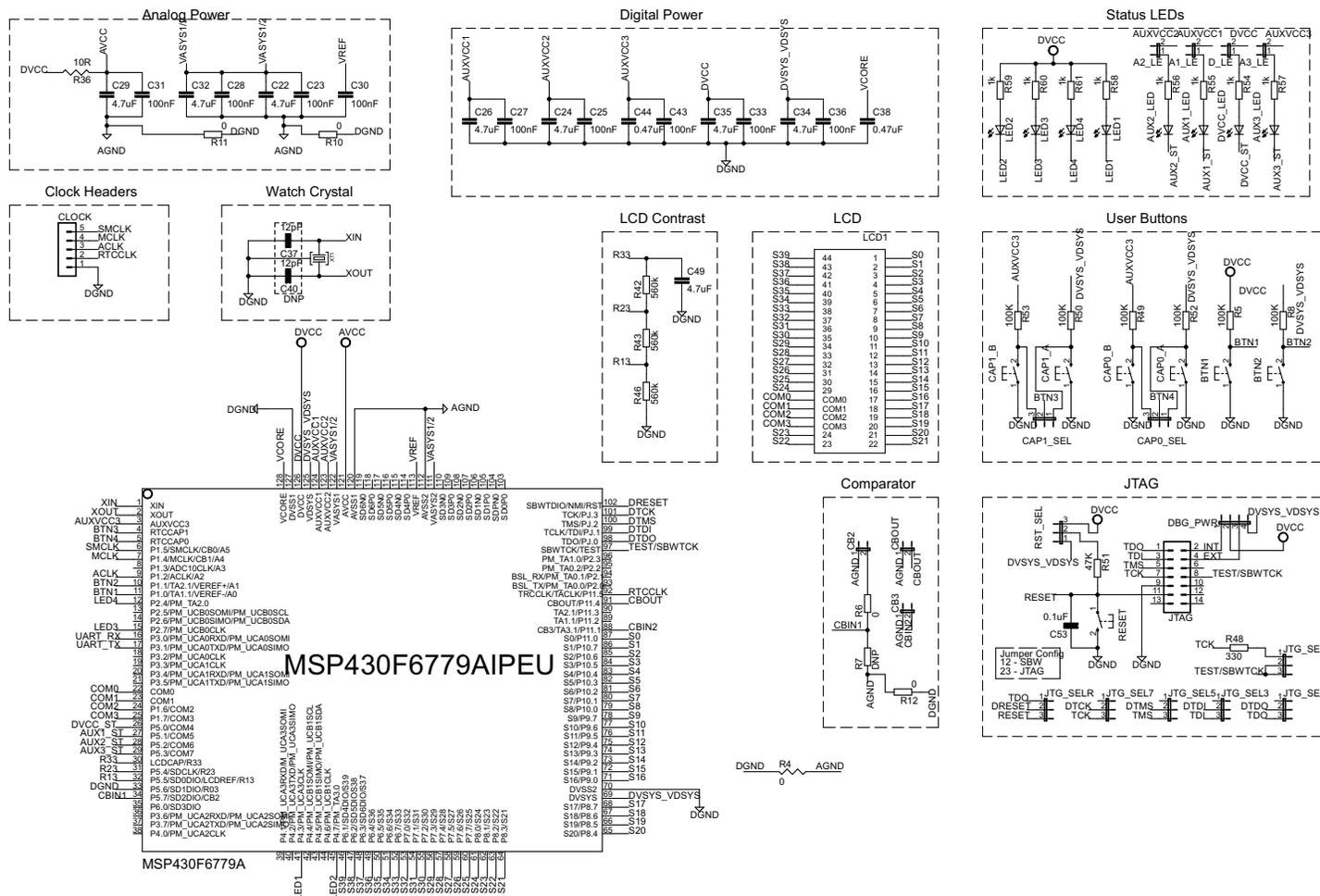
Figure 30. TIDM-AUX-MODULE Schematic Page 1
