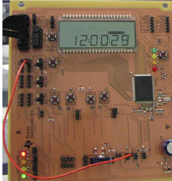
Figure 13. AUX07 Code Example: AUXVCC3 Voltage Rises Above 2.5-V Threshold After Falling Below It
