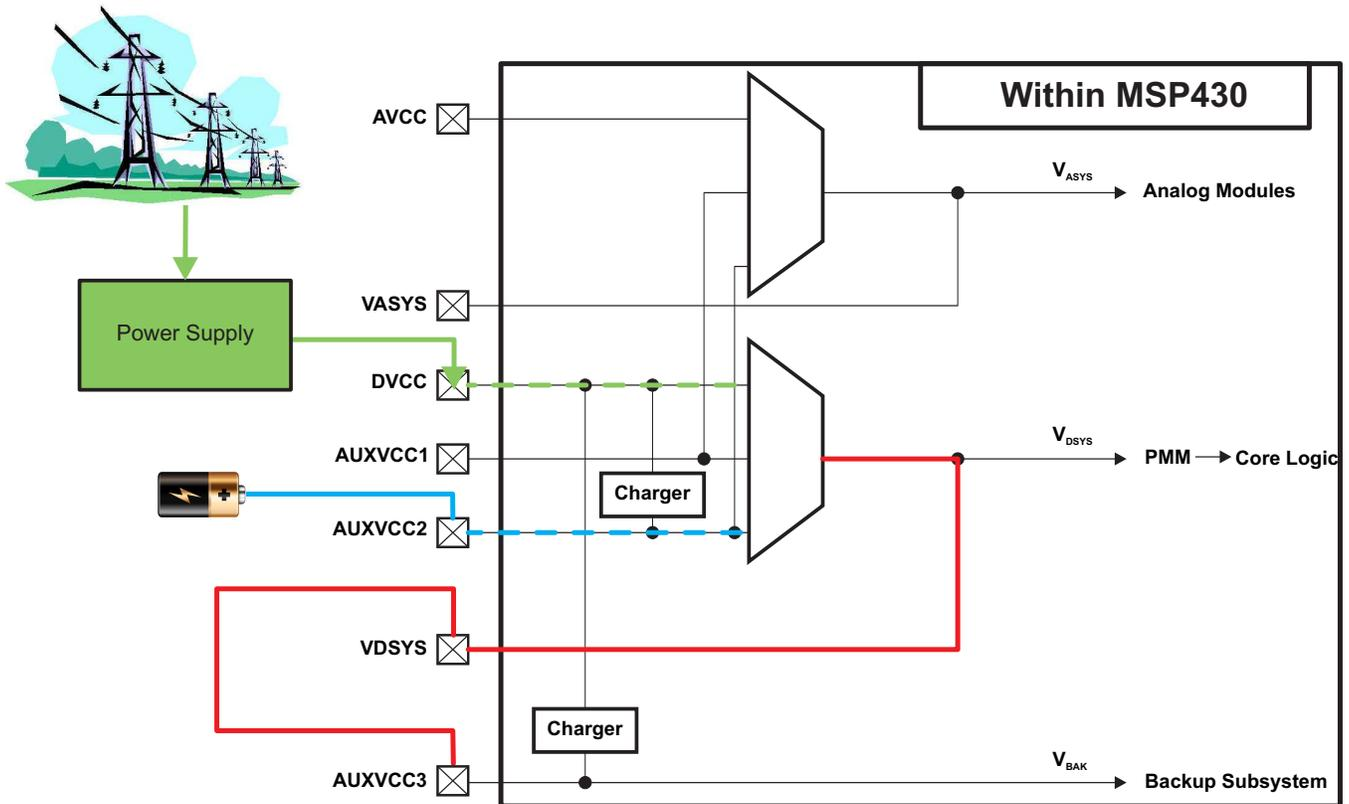
**Figure 4. AUX Configuration for RTC and MSP430 Back-Up Power**
