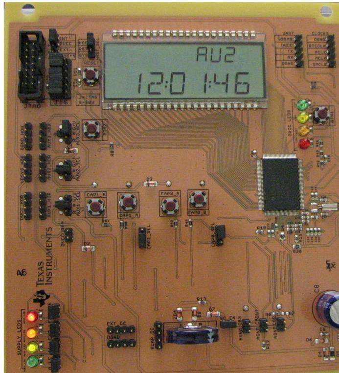
**Figure 9. AUX03 Code Example: Chip Being Powered from AUXVCC2**
