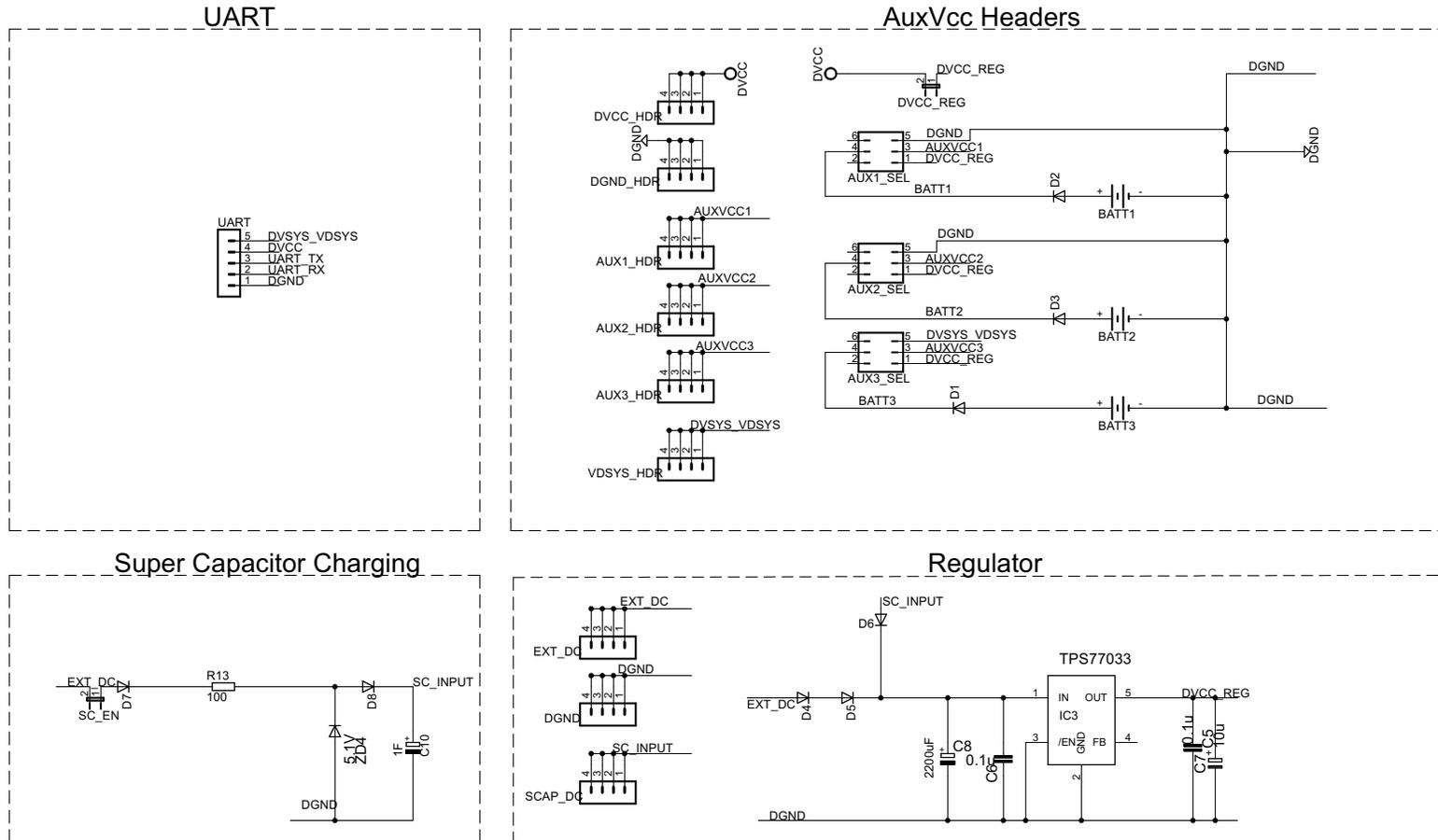
Figure 31. TIDM-AUX-MODULE Schematic Page 2
