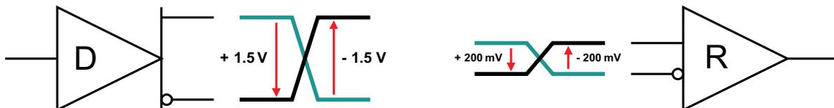
Figure 5. RS-485 Specified Minimum Bus Signal Levels
