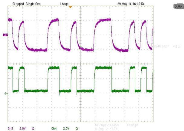
Figure 27. Level-Shifter Output at 1.25-Mbps
