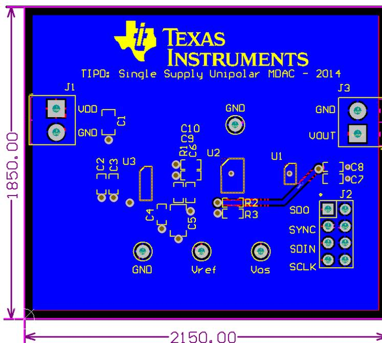
**Figure 8: PCB Layout, Bottom Layer**
