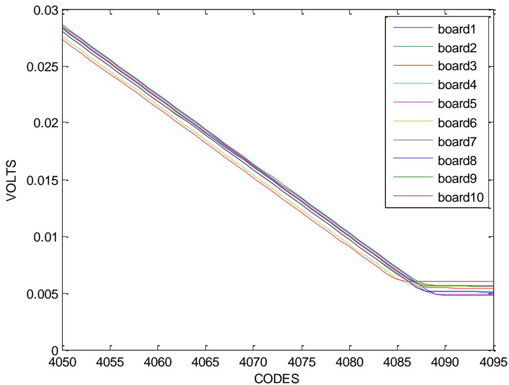
Figure 11: Output voltage for code 4050 to 4095
