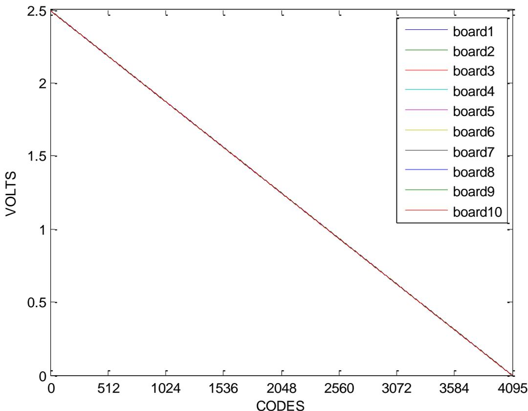
**Figure 9: Measured transfer function**
