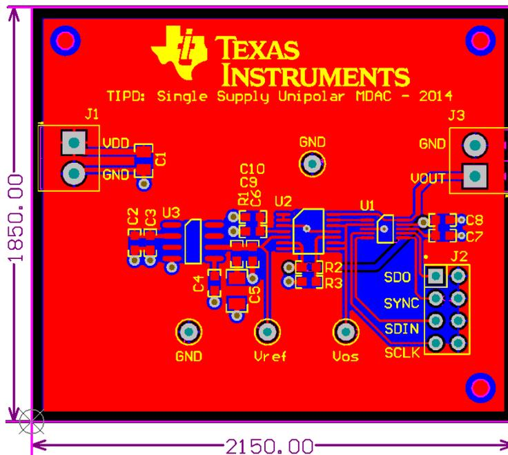
**Figure 7: PCB Layout, Top Layer**
