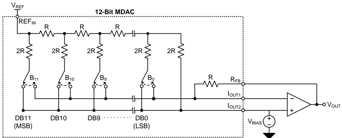
Figure 4: MDAC with offset voltage
