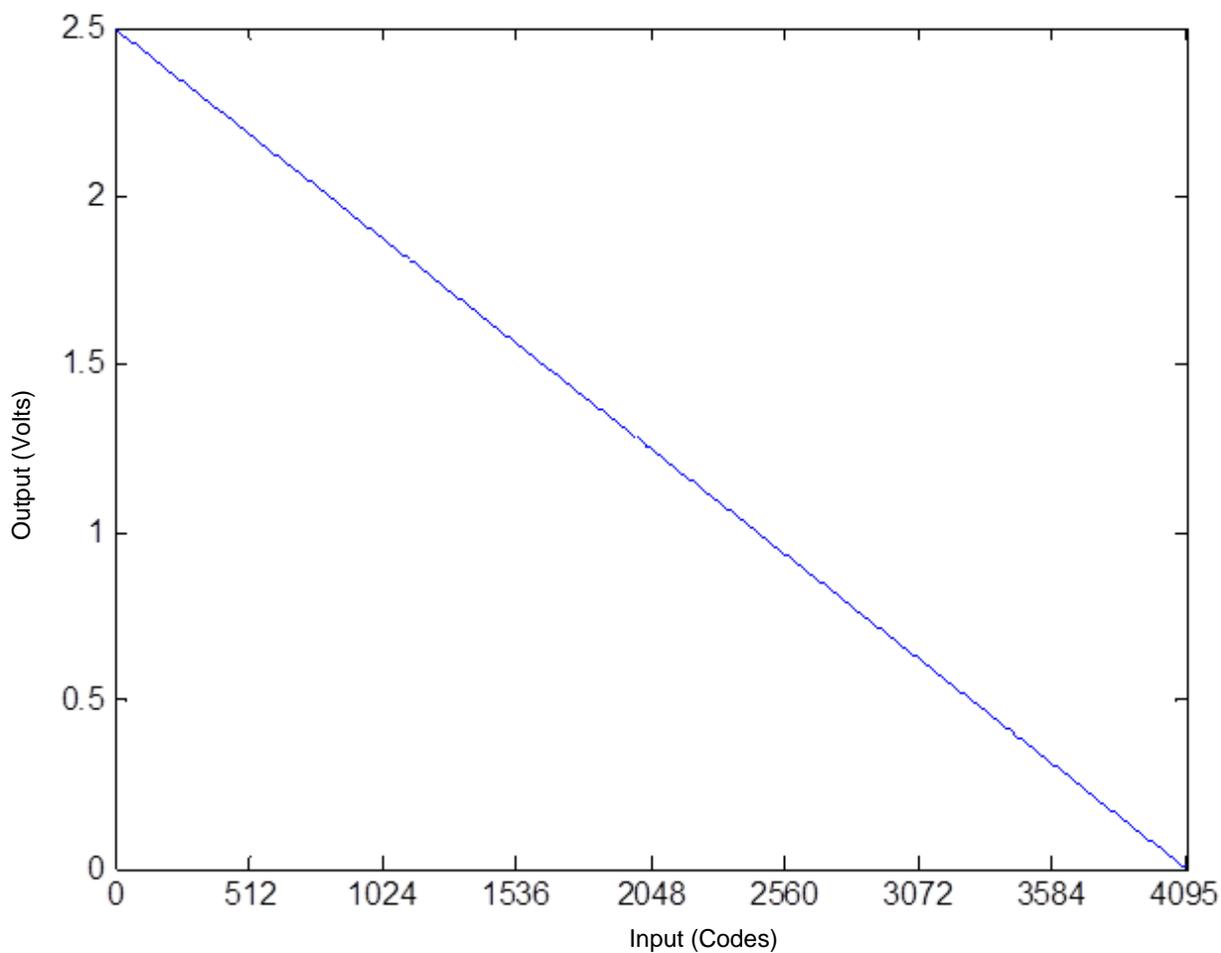
**Figure 1: Measured Transfer Function**
