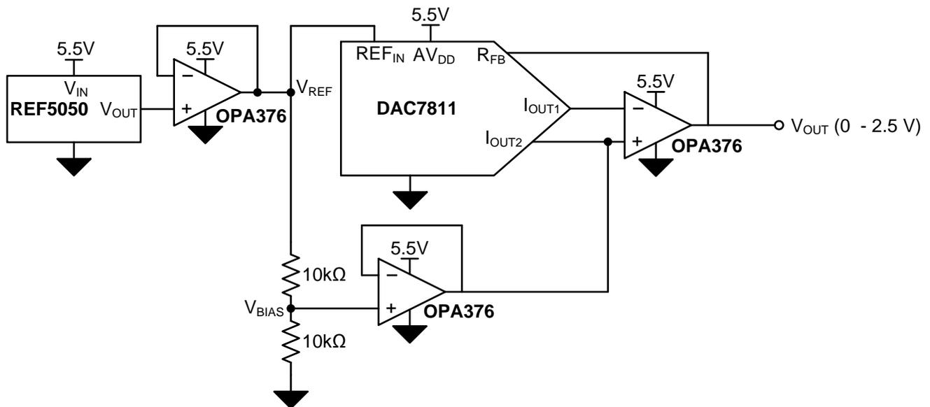
**Figure 2: Complete Circuit Schematic**
