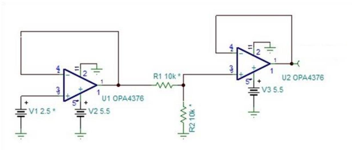
**Figure 6: TINA-TI schematic to calculate offset error**
