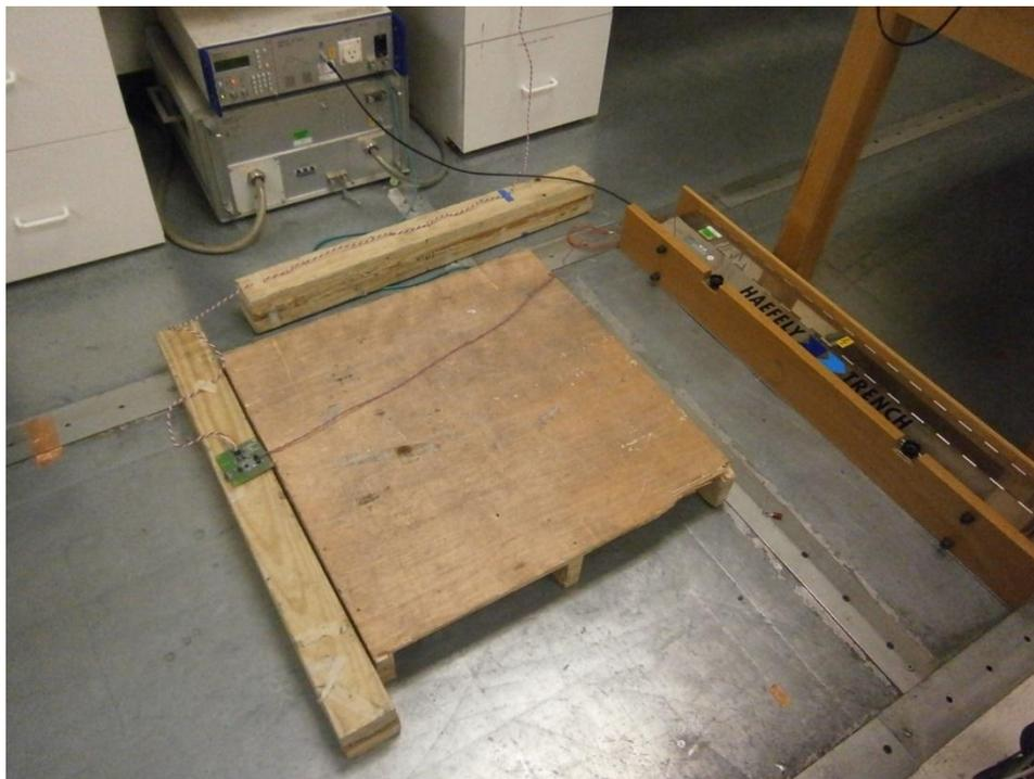
**Figure B-4: EFT Test Setup**
