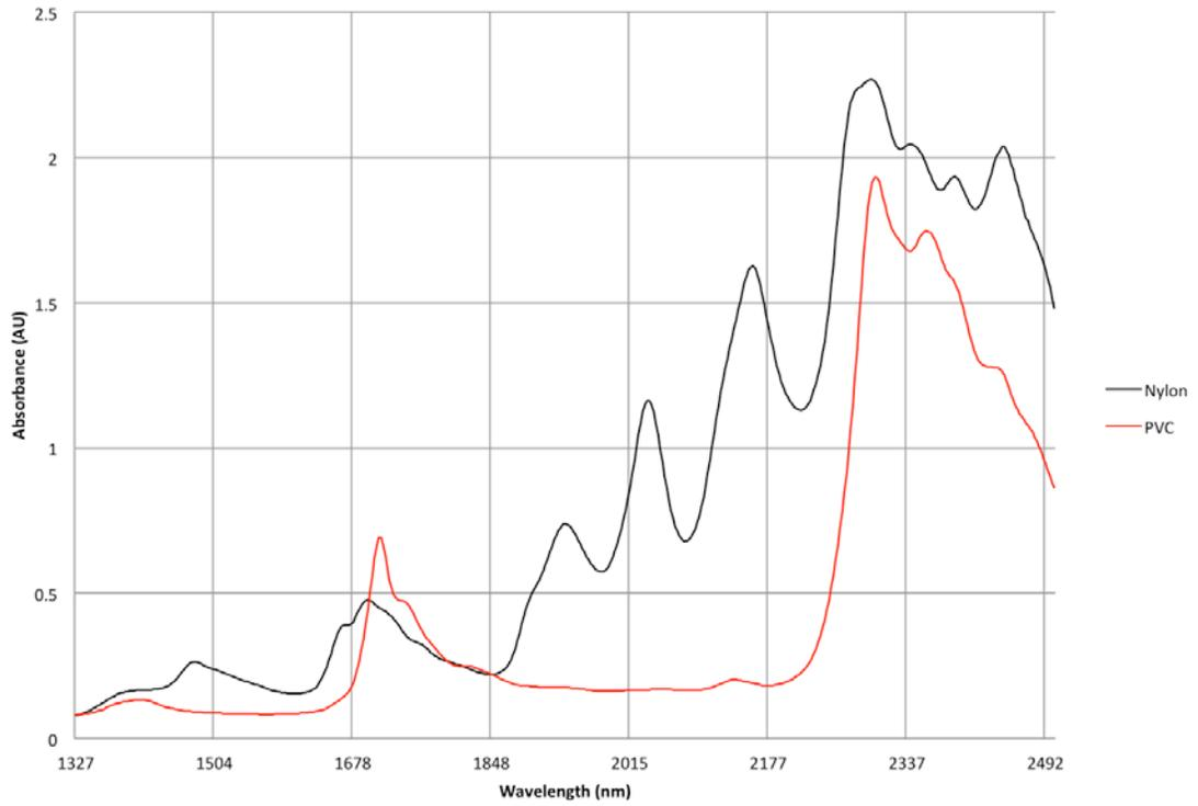
**Figure 2. Wavelength Absorbance Spectrum Comparison of Nylon and PVC**
