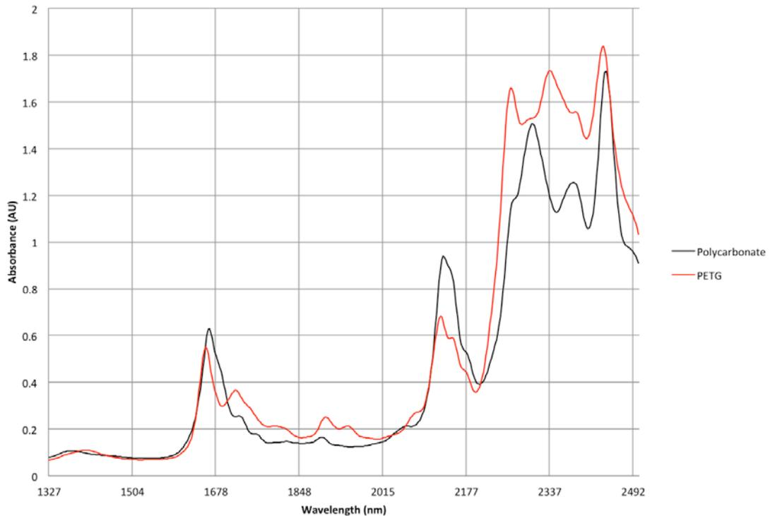
Figure 1. Wavelength Absorbance Spectrum Comparison of Polycarbonate and PETG
