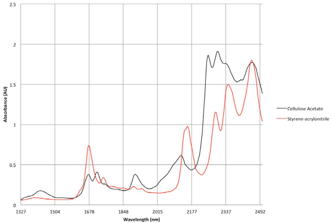
**Figure 3. Wavelength Absorbance Spectrum Comparison of Cellulose Acetate and Styrene-acrylonitrile**
