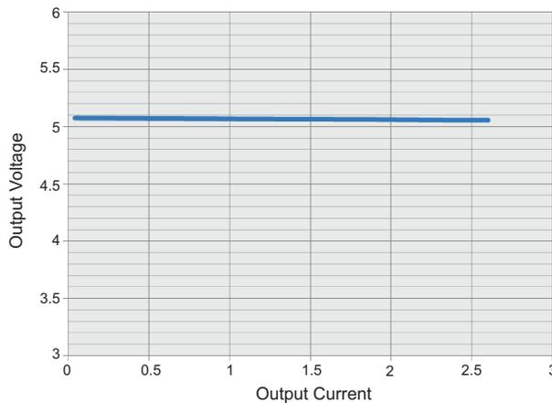
**Figure 10. Output Voltage Versus Load Current**
