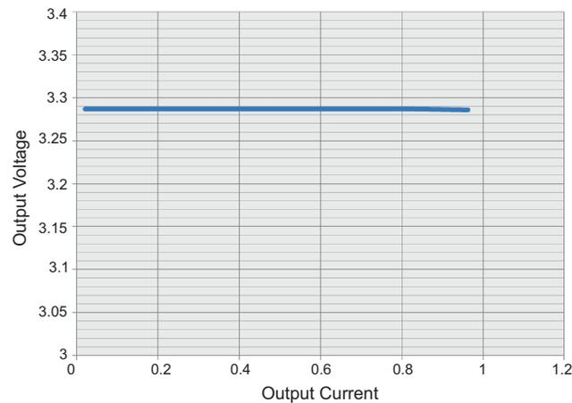
**Figure 20. Output Voltage Versus Load Current**
