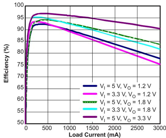
Figure 12. TPS5432 Efficiency Curve
