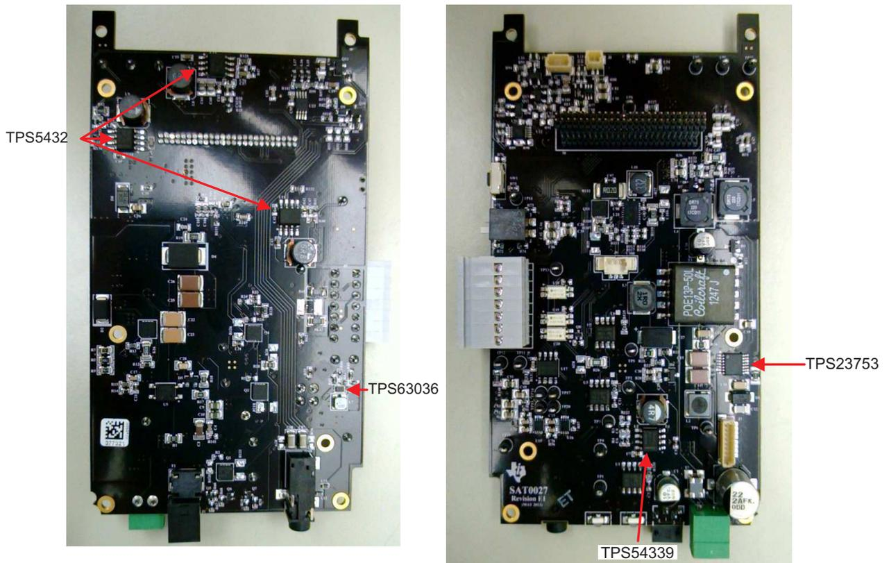
**Figure 4. Power Module Board Design Showing Location of Major Components**
