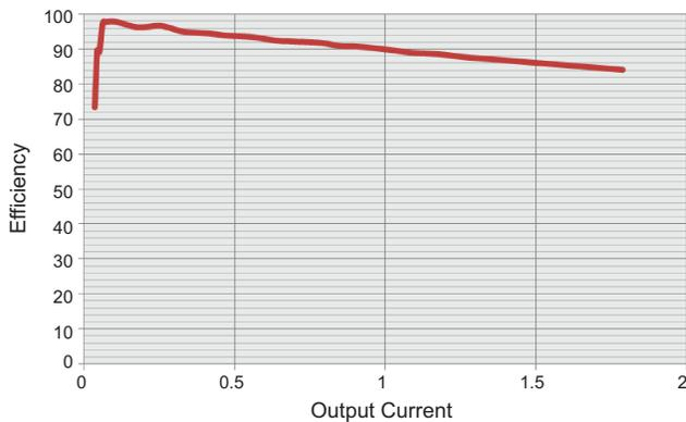
Output voltage = 1.2 V, input voltage = 5 V
