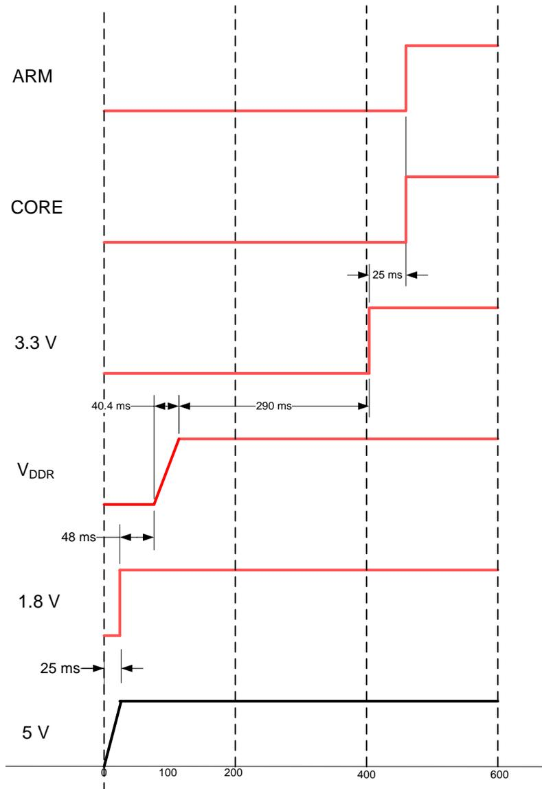
Figure 36. Power Supply Timing Sequence (Measured)
