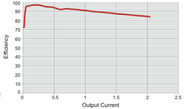
Output voltage = 1.35 V, input voltage = 5 V
