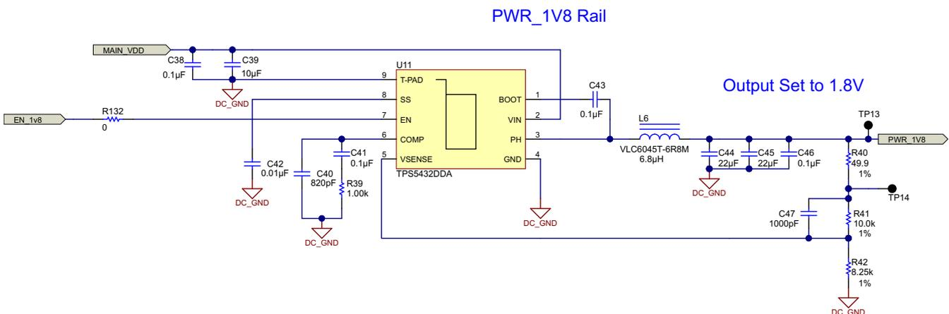
Figure 11. Power Module 1.8-V Circuit
