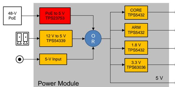
Figure 2. Power Module Block Diagram
