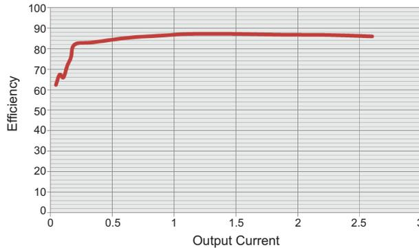
**Figure 9. PoE — TPS23753A Rail (No Other Rails Enabled)**
