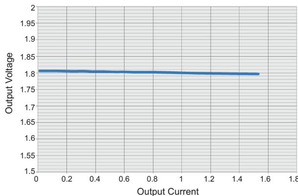
Figure 14. Output Voltage Versus Load Current
