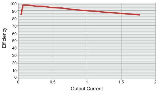
Output voltage = 1.2 V, input voltage = 5 V
