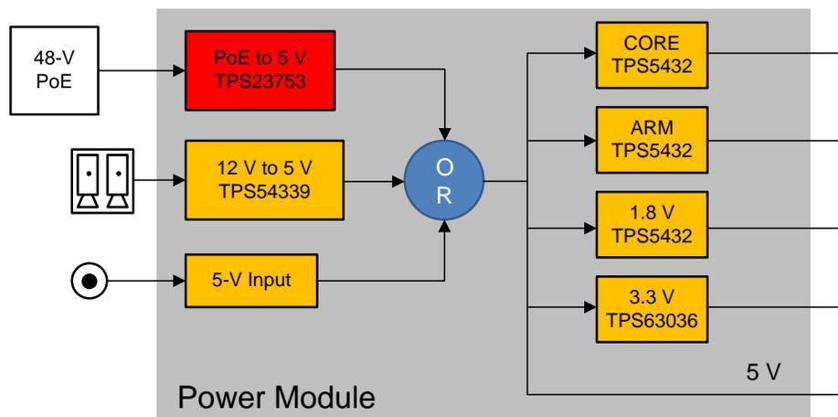
**Figure 3. Power Module Block Diagram**
