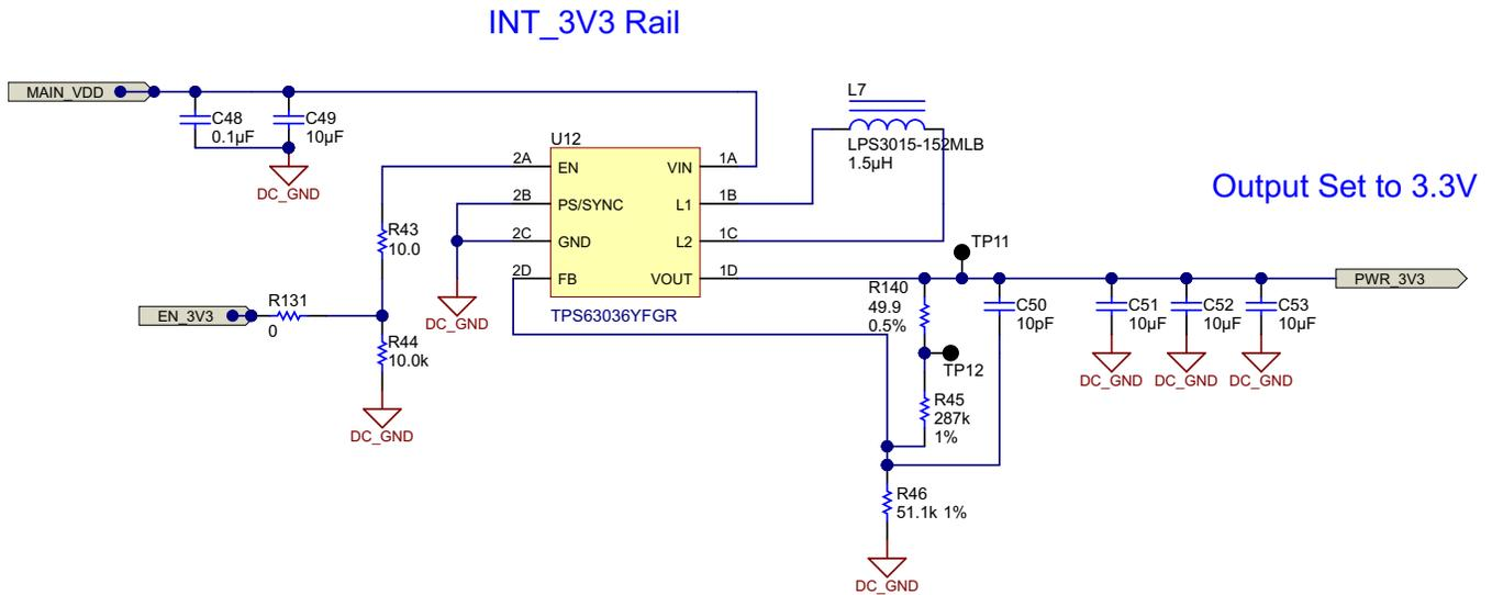
Figure 16. Power Module 3.3-V Circuit
