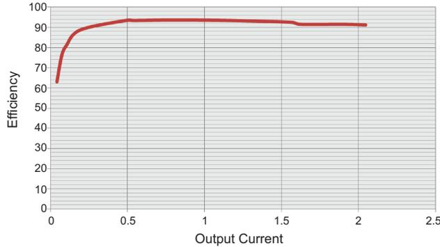
**Figure 6. Measured Efficiency Versus Output Current**
