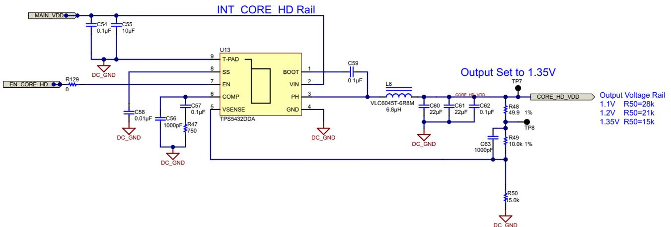
Figure 23. Power Module Core Supply Circuit
