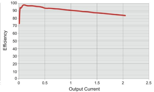
Output voltage = 1.35 V, input voltage = 5 V
