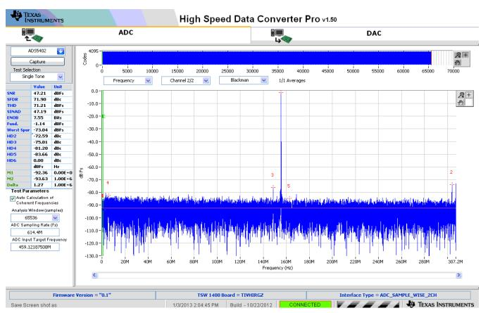
Figure 8. TSW1266 Sample Capture using the TSW1400
