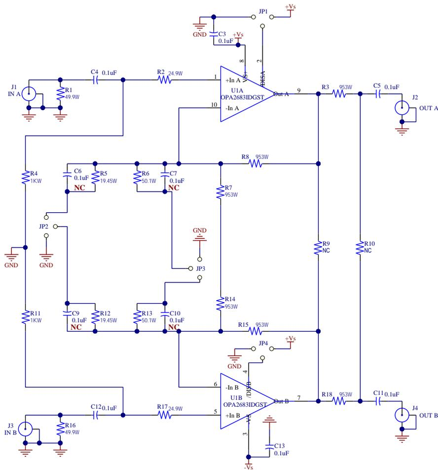
Figure 2: (Test Circuit)
