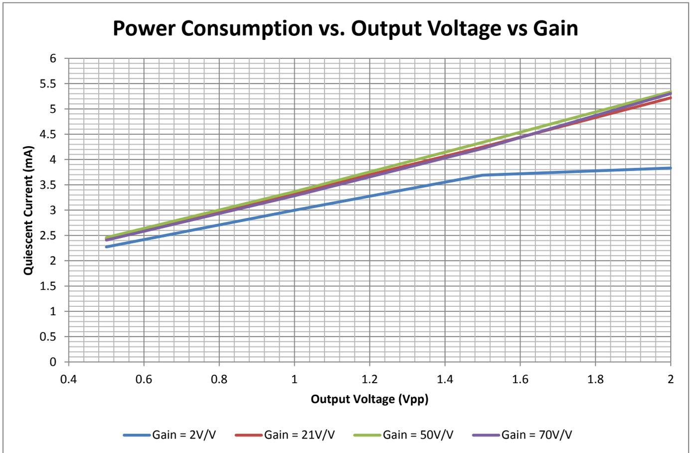
**Figure 9: Power Consumption vs. Output Voltage vs. Gain**
