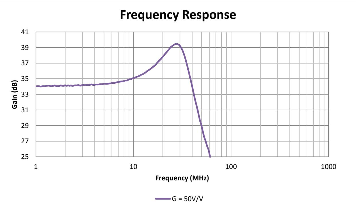
**Figure 5: ( $G = 50\text{V/V}$  -3dB BW = 45MHz)**
