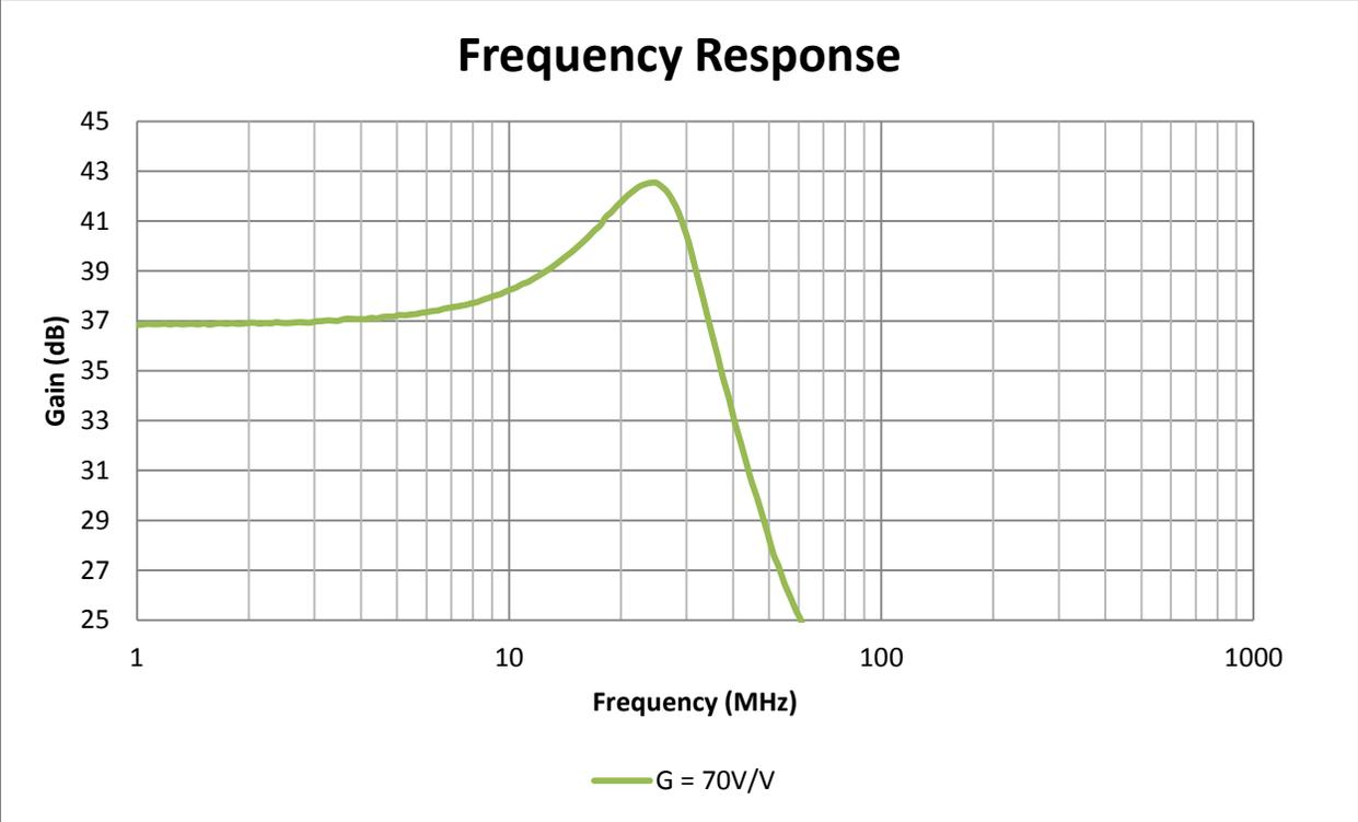
**Figure 6: ( $G = 70\text{V/V}$  -3dB BW = 40MHz)**
