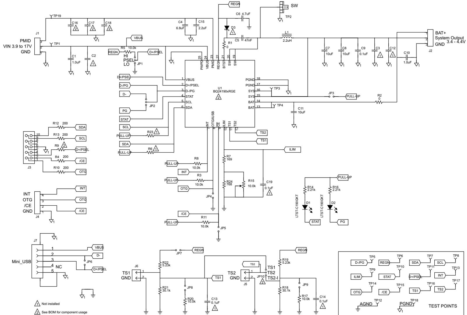
Figure 12. bq24x9xEVM Schematic
