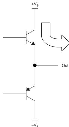
The output current flows through the output stage transistor and is originating from the power supply, as expected. If the supply is ideal and has constant low impedance over frequency,
