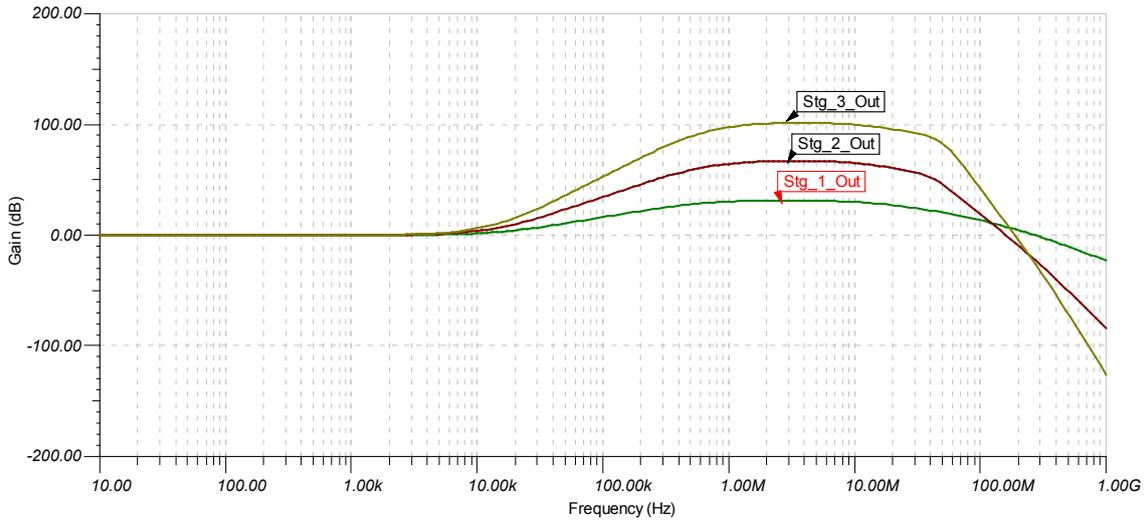
Figure 4.3: Simulated Frequency Response,  $C_{AC-GAIN} = 10\mu F$
