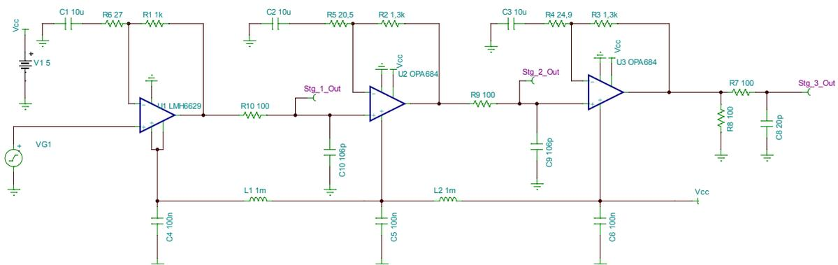
Figures 4.2 and 4.3 show simulated frequency responses with different gain AC coupling capacitor values. To ensure that the flat band is as wide as possible, select high capacitor values. On the stages featuring the current feedback OPA684 amplifier, the gain resistor shields the capacitor from the low impedance non-inverting input of the amplifier.
