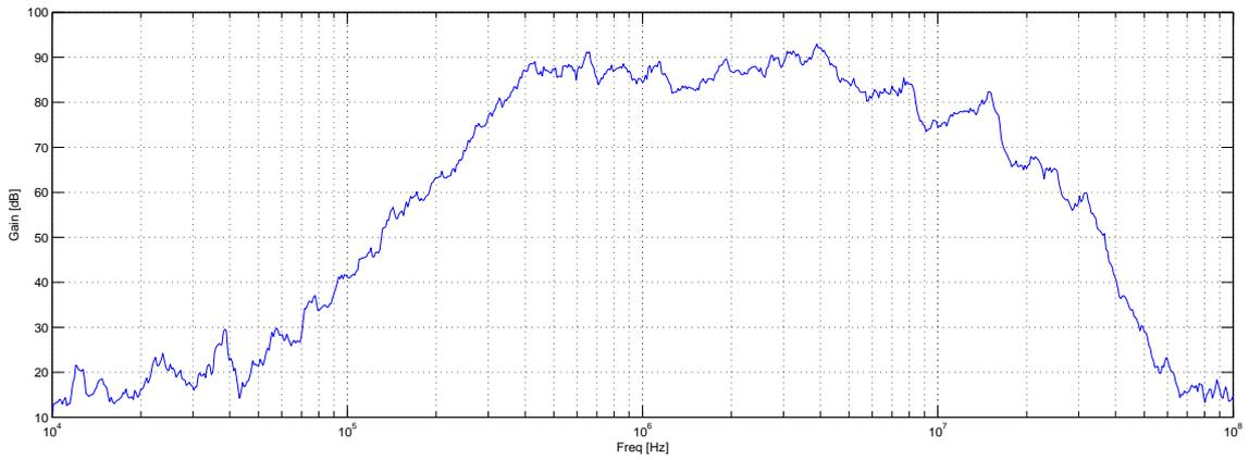
Figure 6.5: Measured Frequency Response, 10kHz-100MHz,  $C_{AC-GAIN} = 10\mu F$
