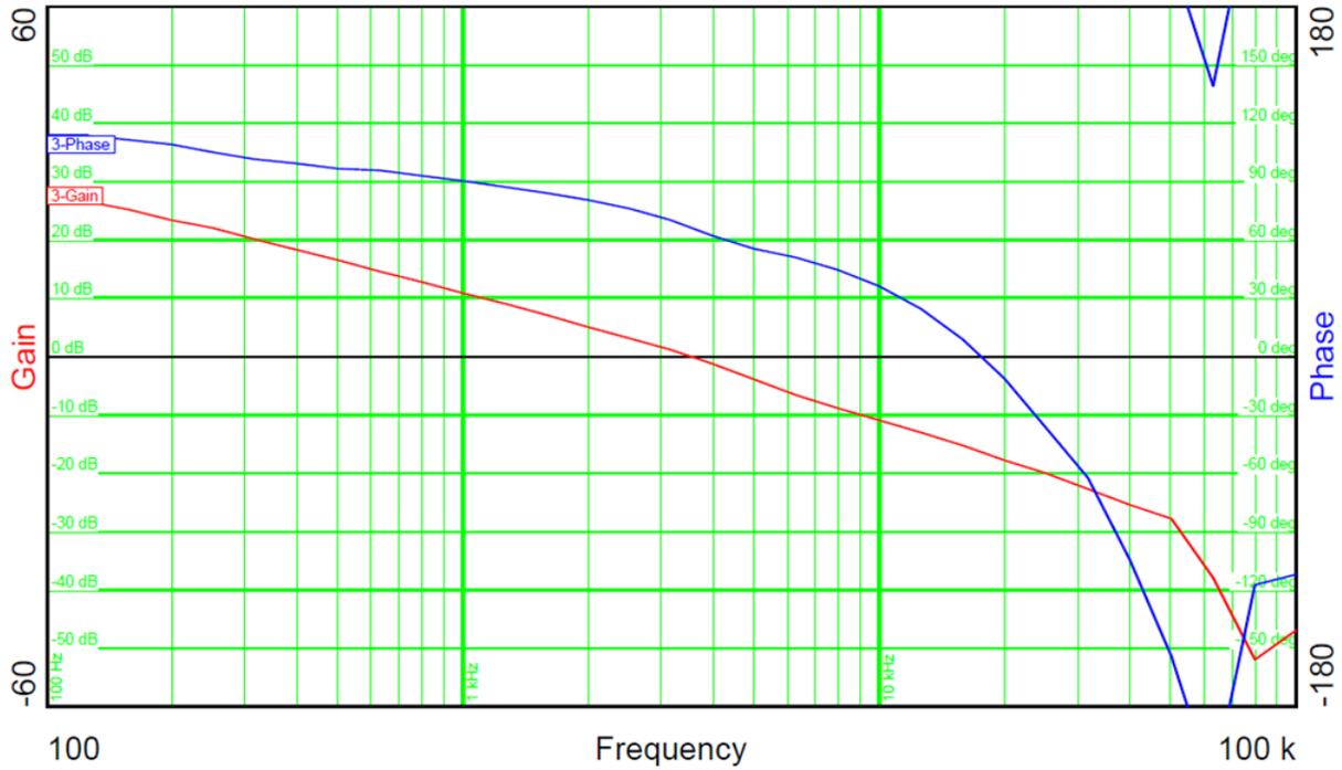
Figure 2-5. Bode Plot With Electronic Load
