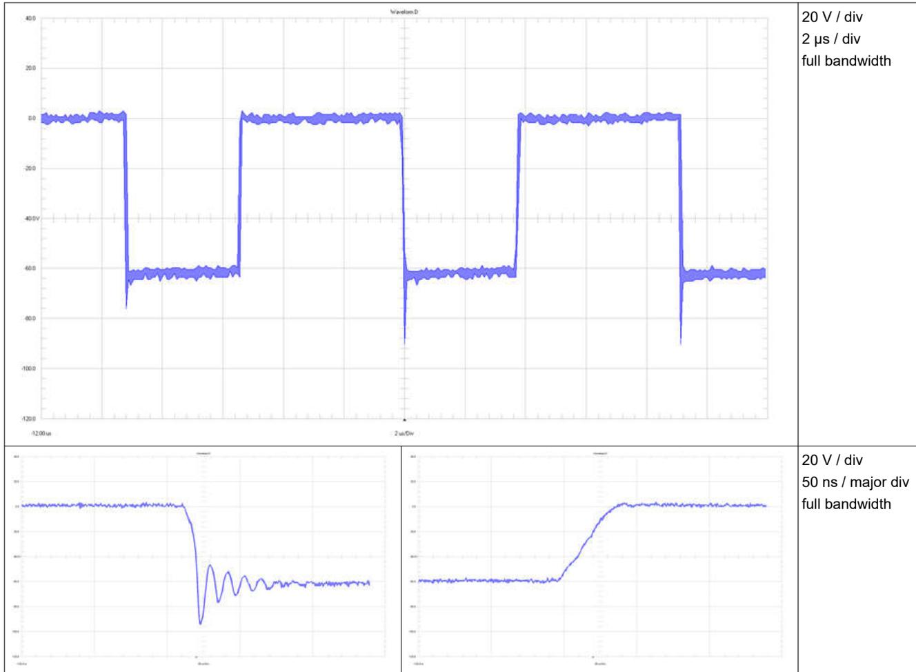
**Figure 3-4. Switching Q1 at 36-V Input Voltage**
