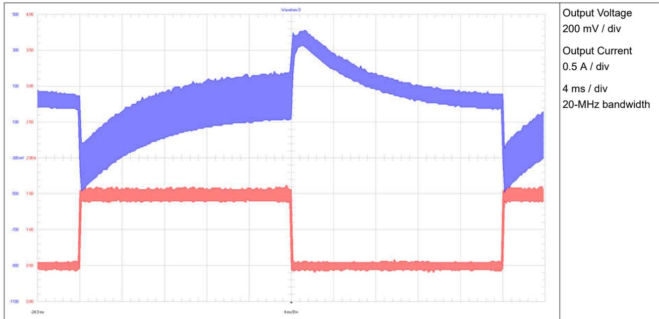
**Figure 3-6. Load Transient 0.5 A to 1.5 A**
