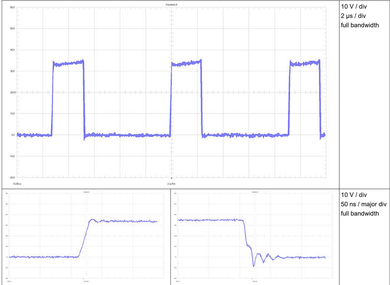
Figure 3-1. Switching Q2 at 9-V Input Voltage
