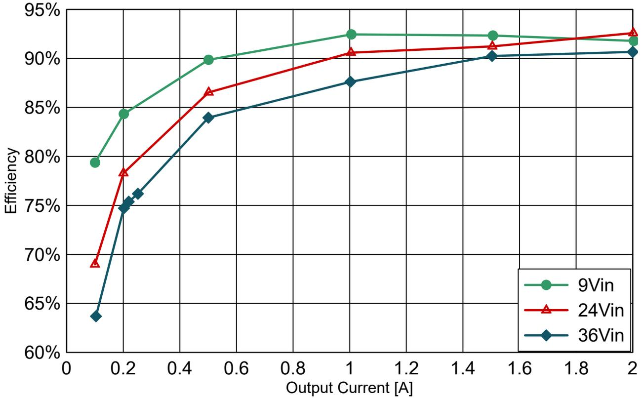
Figure 2-1. Efficiency Graph
