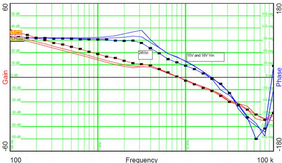
Figure 2-3. Bode Plot With Battery During Recharging Phase
