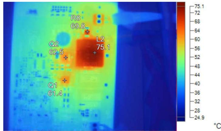
Figure 2-2. Thermal Image (9-V Input voltage, 24-V Output Voltage, 2-A Output Current)
