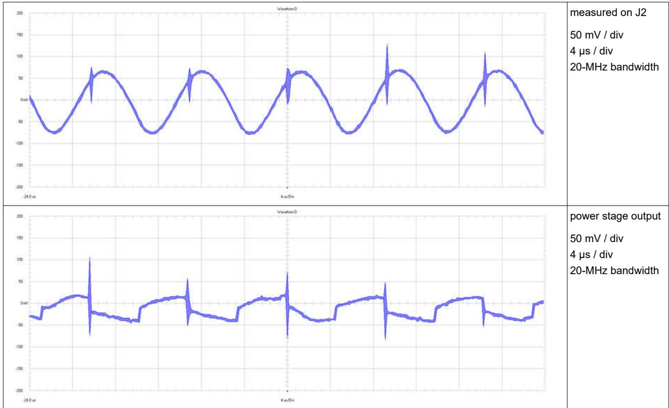
Figure 3-5. Output Voltage Ripple
