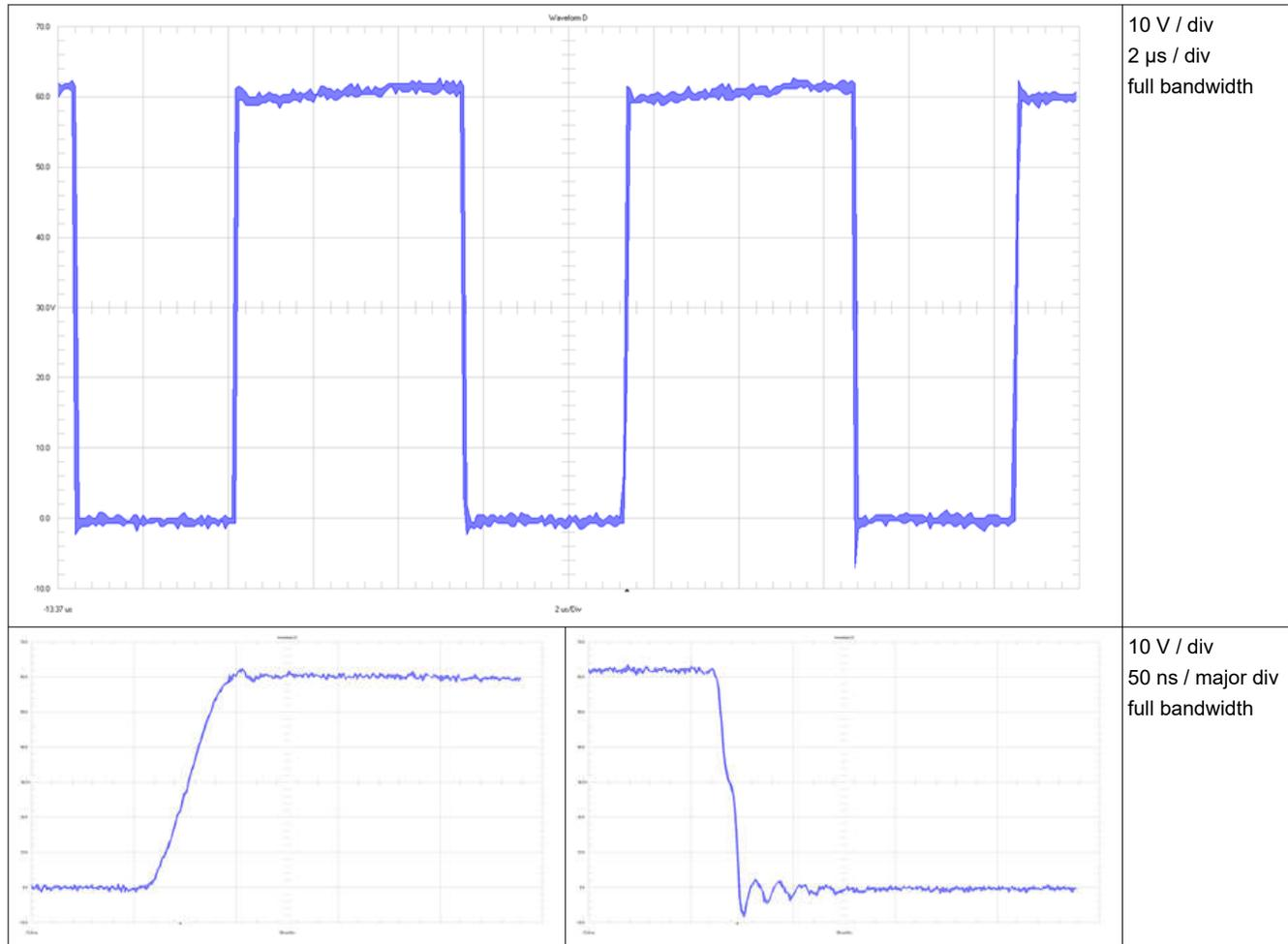
Figure 3-2. Switching Q2 at 36-V Input Voltage
