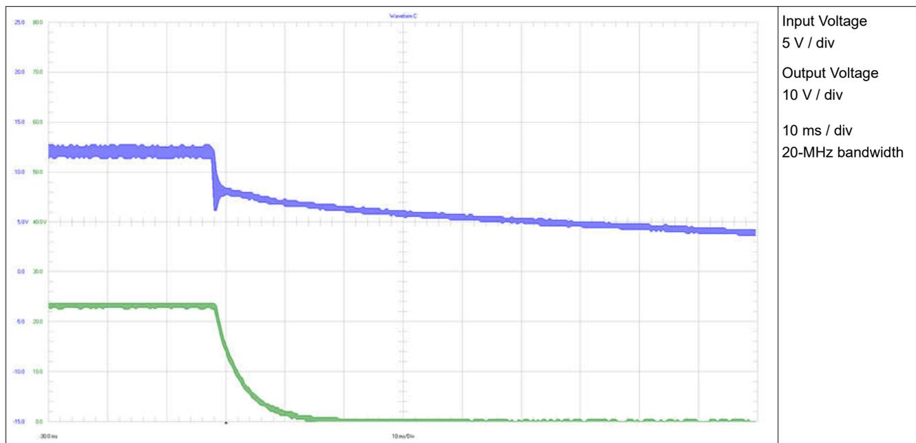
Figure 3-8. Shutdown With 12-V Input Voltage
