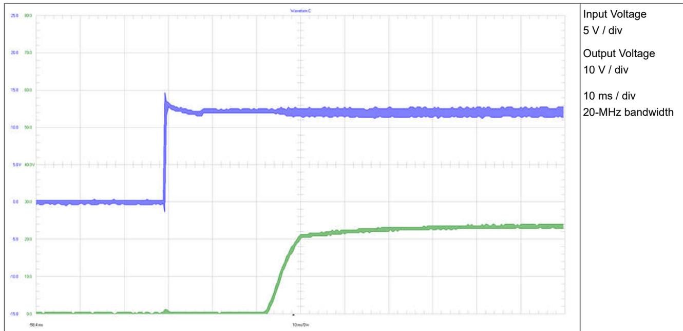
Figure 3-7. Start-up With 12-V Input Voltage
