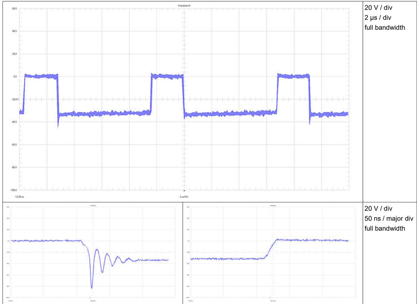
**Figure 3-3. Switching Q1 at 9-V Input Voltage**
