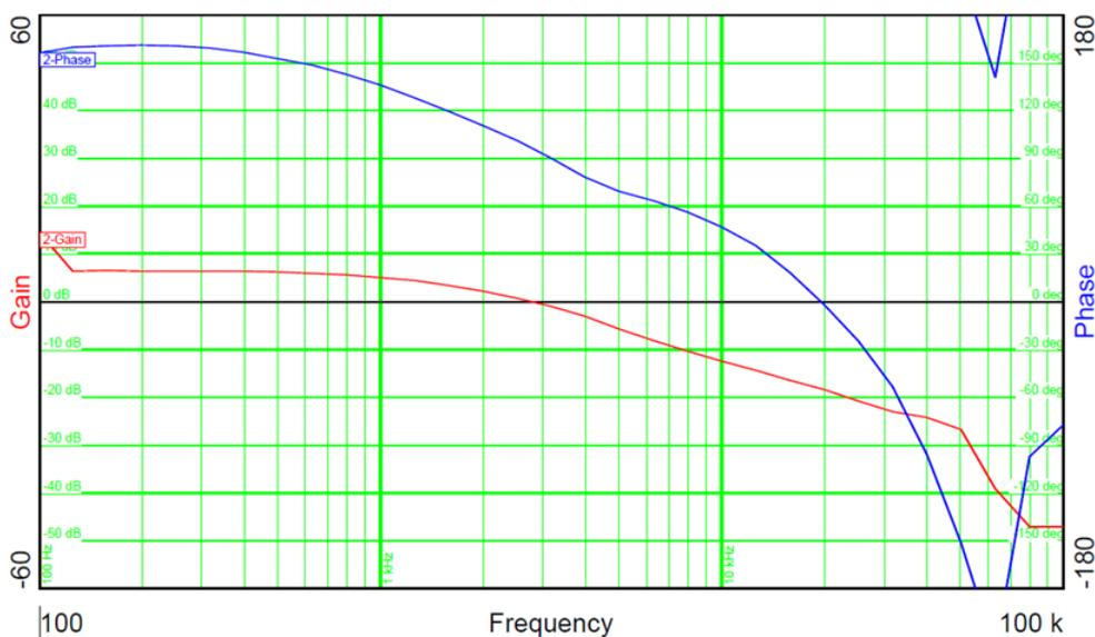
Figure 2-4. Bode Plot With Battery at Constant Battery Voltage
