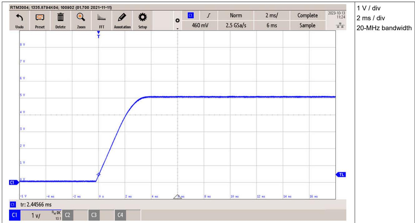
Figure 3-3. Start-Up Into 32-A Load
