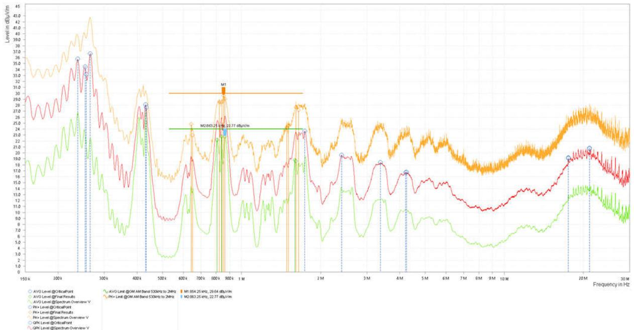
Figure 2-6. Radiated Emissions, 150 kHz to 30 MHz
