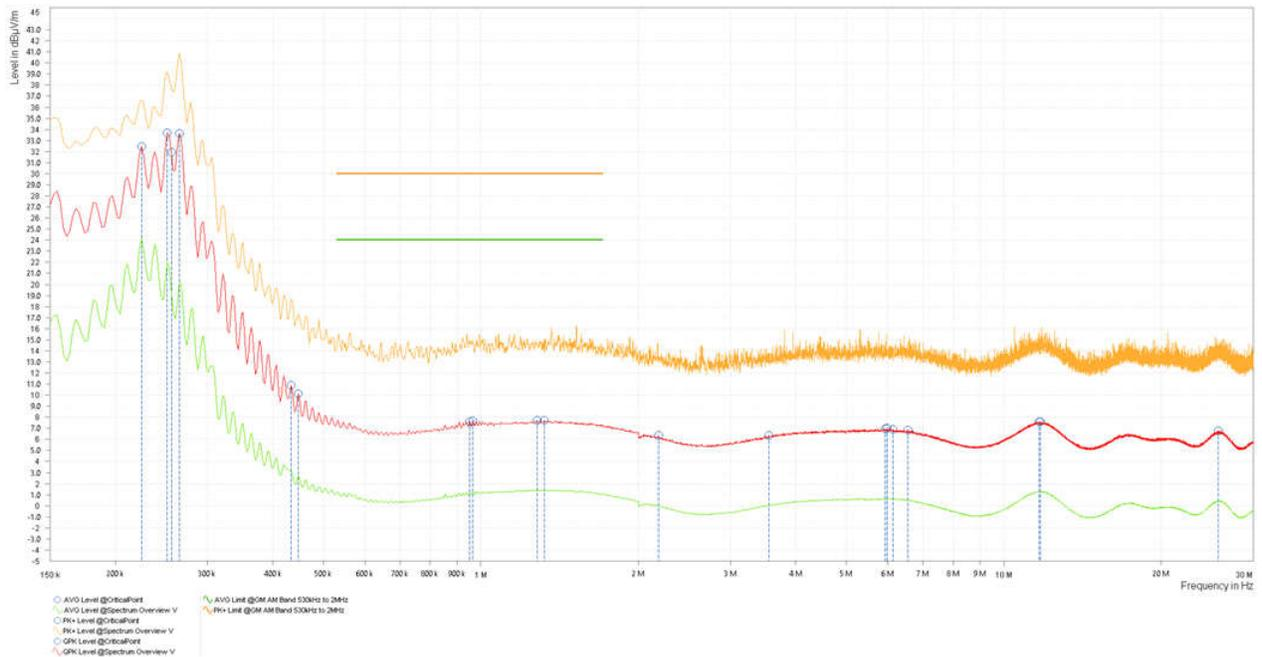
Figure 2-5. Noise Floor, 150 kHz to 30 MHz
