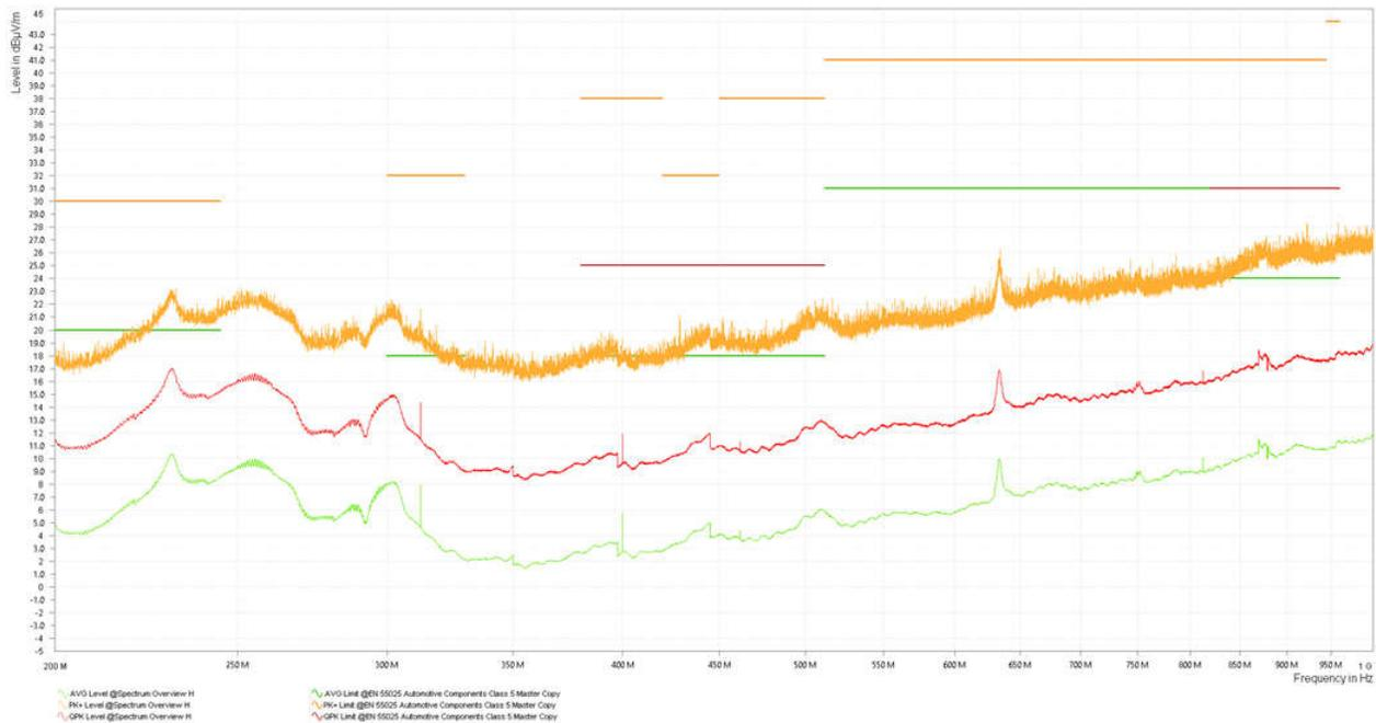
Figure 2-12. Radiated Emissions, 200 MHz to 1 GHz, Horizontal Polarization
