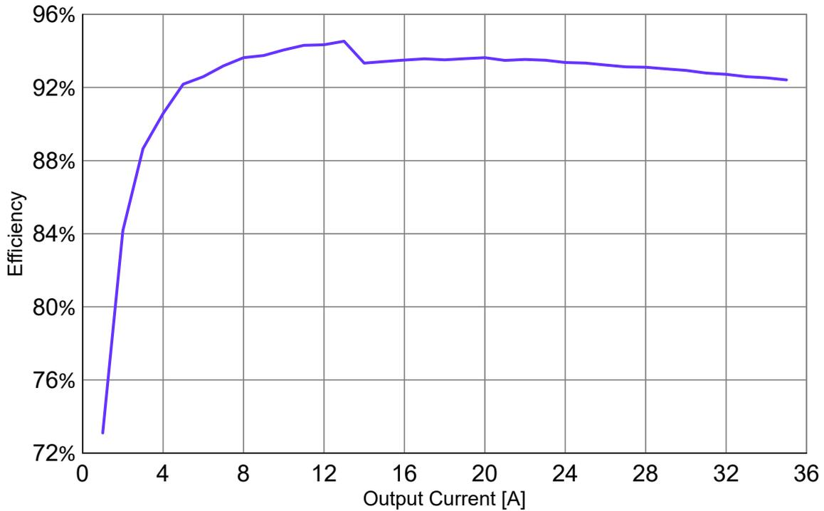
Figure 2-1. Efficiency Graph
