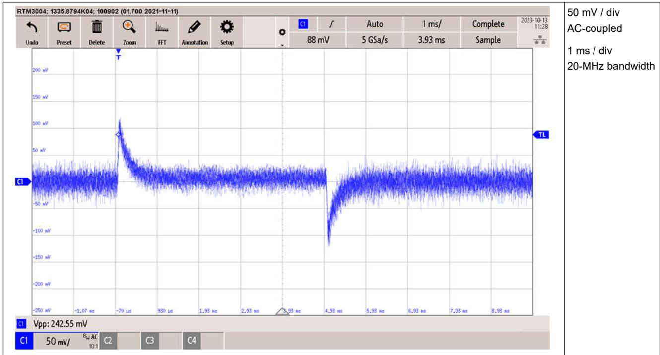
Figure 3-2. Load Step 5 A to 32 A to 5 A
