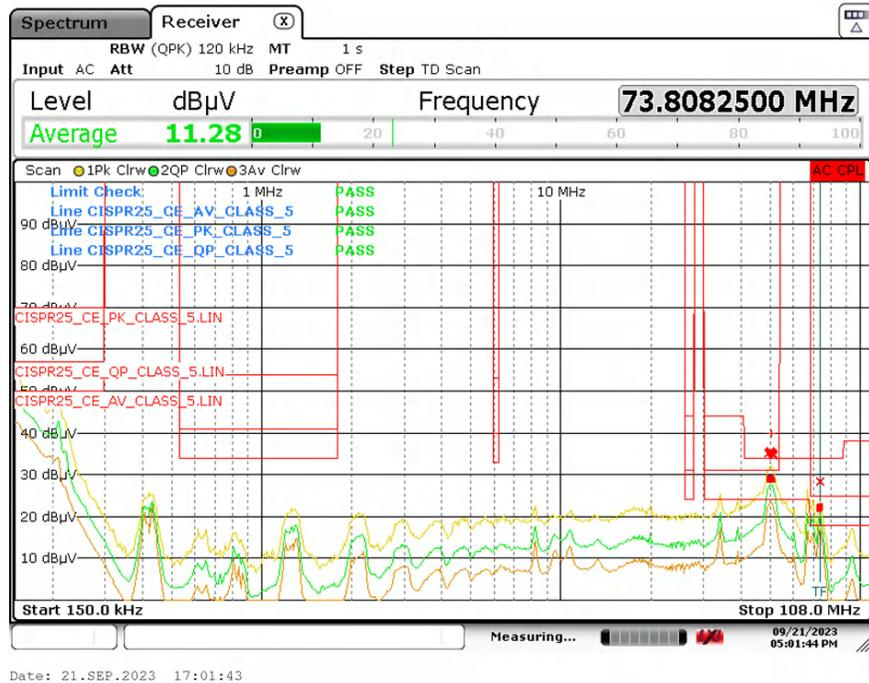
Figure 2-4. Results of Conducted Emissions
