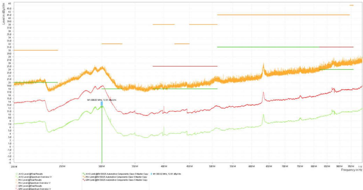
Figure 2-14. Radiated Emissions, 200 MHz to 1 GHz, Vertical Polarization
