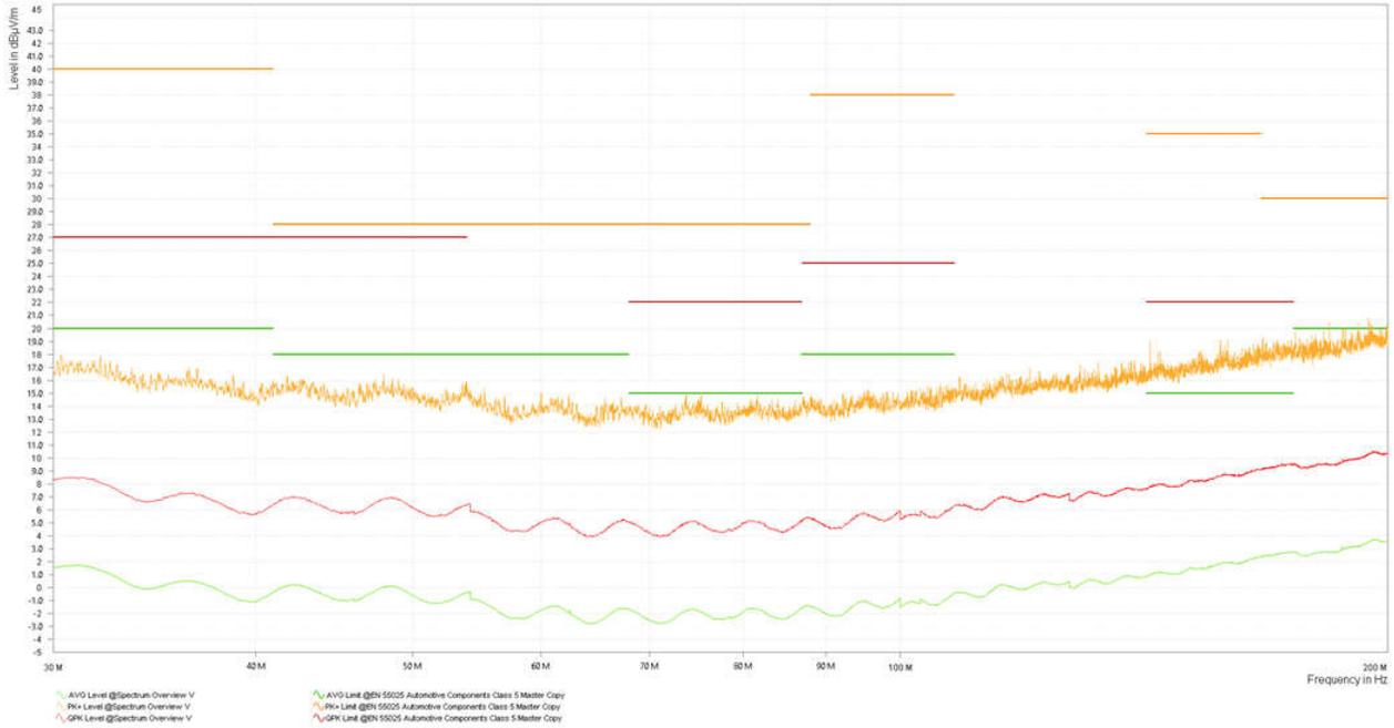
Figure 2-9. Noise Floor, 30 MHz to 200 MHz, Vertical Polarization
