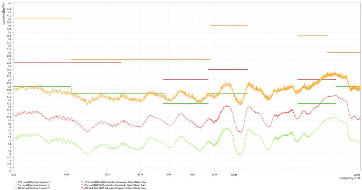
Figure 2-10. Radiated Emissions, 30 MHz to 200 MHz, Vertical Polarization
