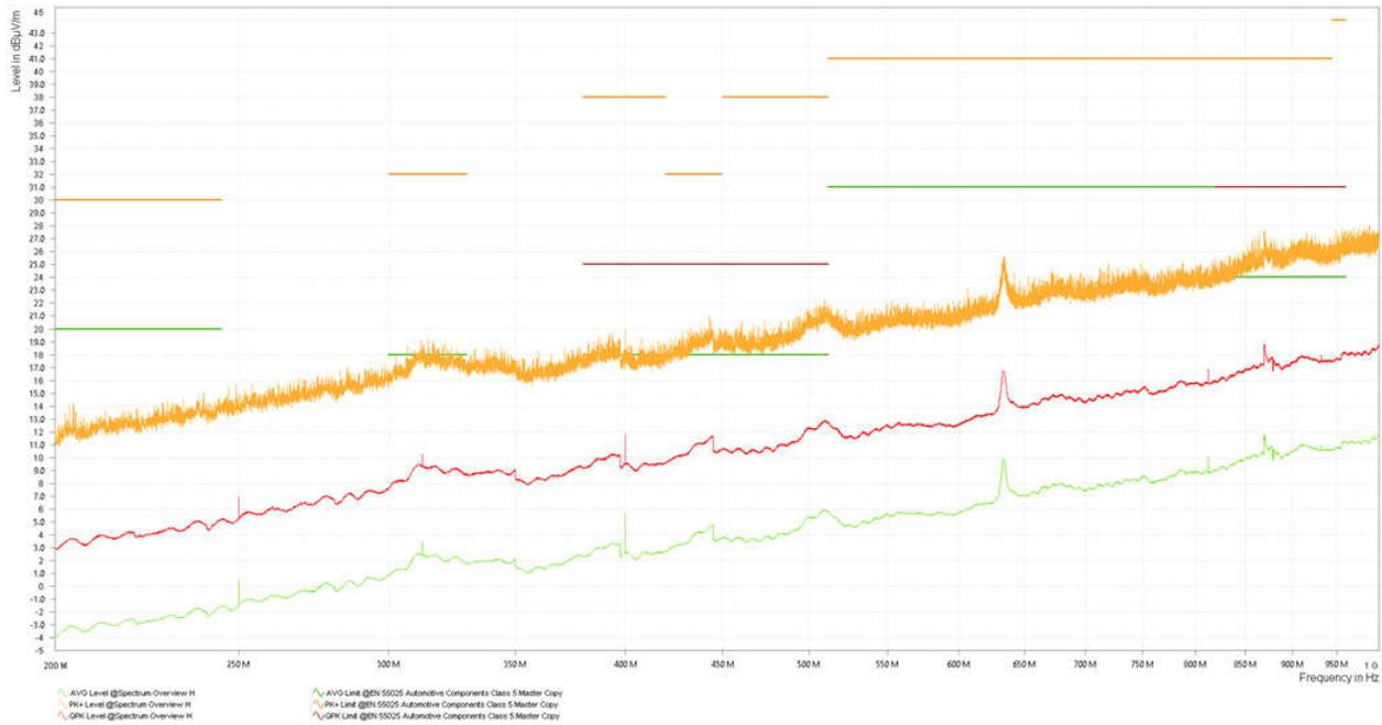
Figure 2-11. Noise Floor, 200 MHz to 1 GHz, Horizontal Polarization
