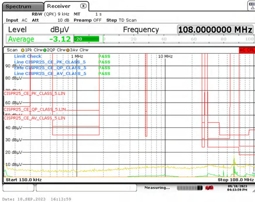
Figure 2-3. Noise Floor of the Conducted Measurement Setup
