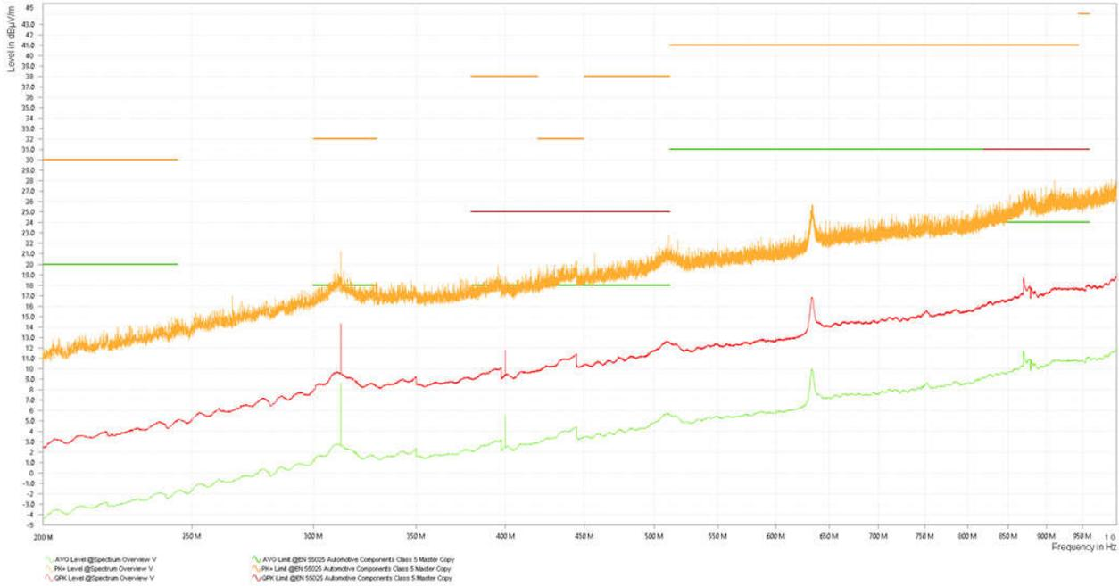
Figure 2-13. Noise Floor, 200 MHz to 1 GHz, Vertical Polarization
