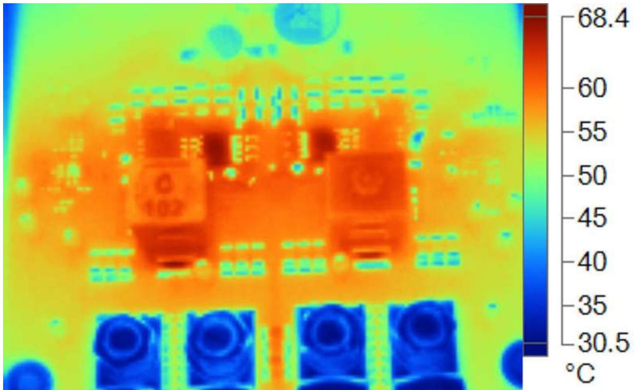
Figure 2-2. Thermal Image, 22-A Load Current
