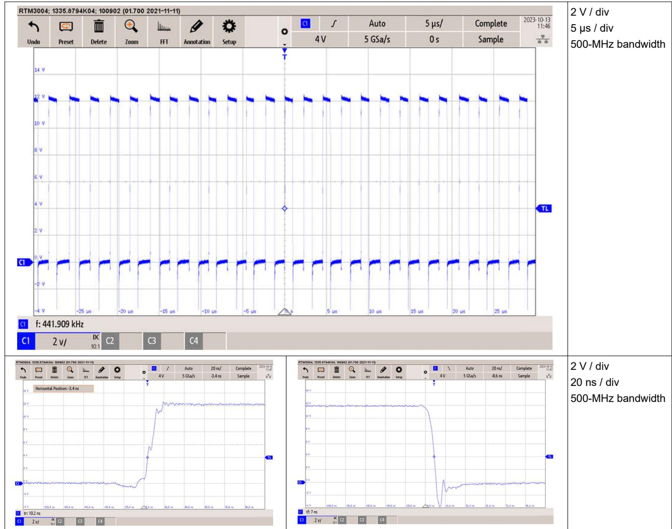
Figure 3-1. Switch Node at 32-A Load Current
