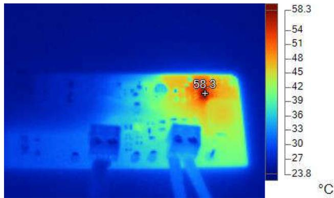
Figure 2-2. Thermal Image at Full DC Load ( $I_{OUT1} = 2\text{ A}$ ,  $I_{OUT2} = 1\text{ A}$ )
