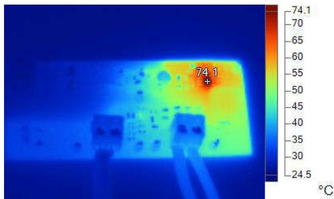
Figure 2-3. Thermal Image at Full Peak Load ( $I_{OUT1} = 2.5\text{ A}$ ,  $I_{OUT2} = 1\text{ A}$ )
