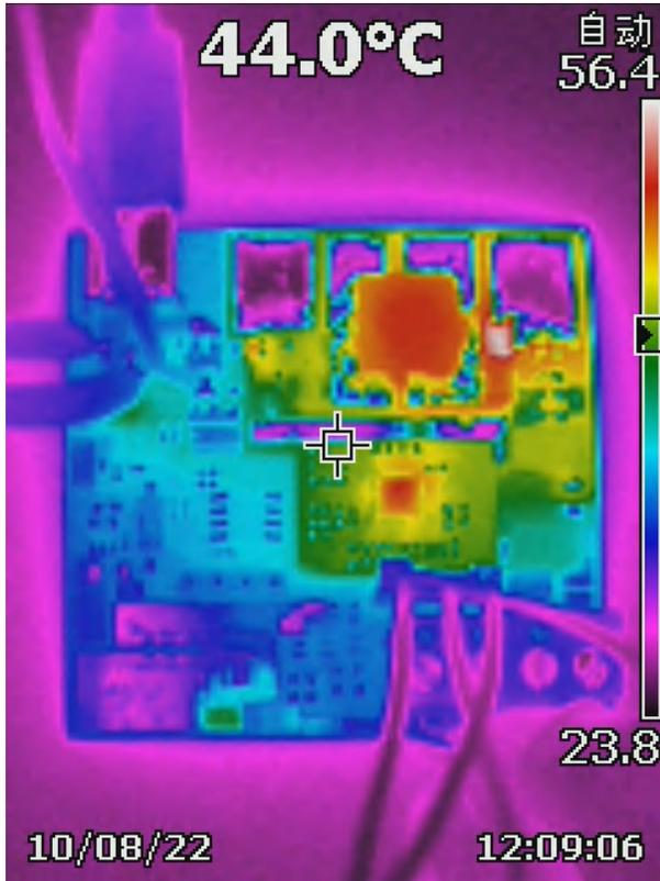
Figure 2-8. 18 V<sub>BAT</sub> to 9 V, 3 A OTG Full Load
