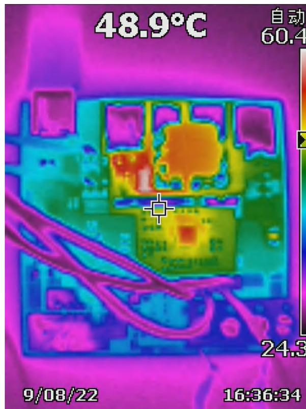
Figure 2-10. 18 V<sub>BAT</sub> to 20 V, 3 A OTG Full Load
