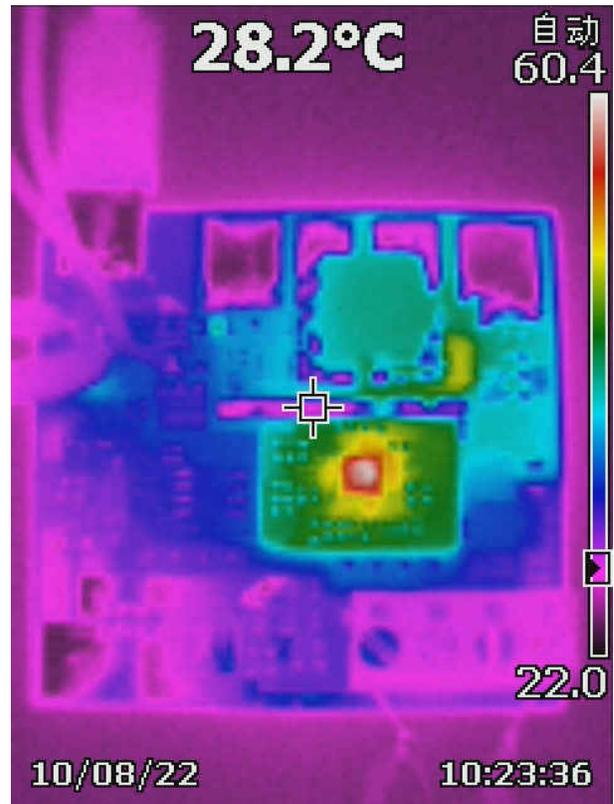
Figure 2-6. 9 V<sub>BUS</sub> and 20 V<sub>BAT</sub> Full Charging Mode
