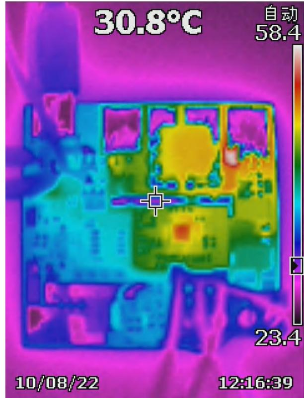
Figure 2-9. 18 V<sub>BAT</sub> to 15 V, 3 A OTG Full Load
