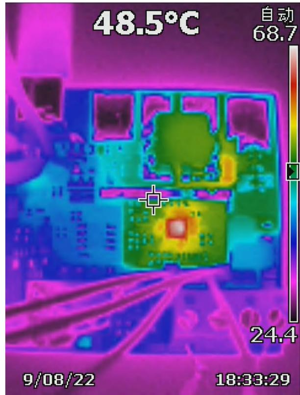
Figure 2-5. 15 V<sub>BUS</sub> and 20 V<sub>BAT</sub> Full Charging Mode
