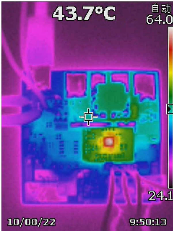
Figure 2-4. 20 V<sub>BUS</sub> and 20 V<sub>BAT</sub> Full Charging Mode
