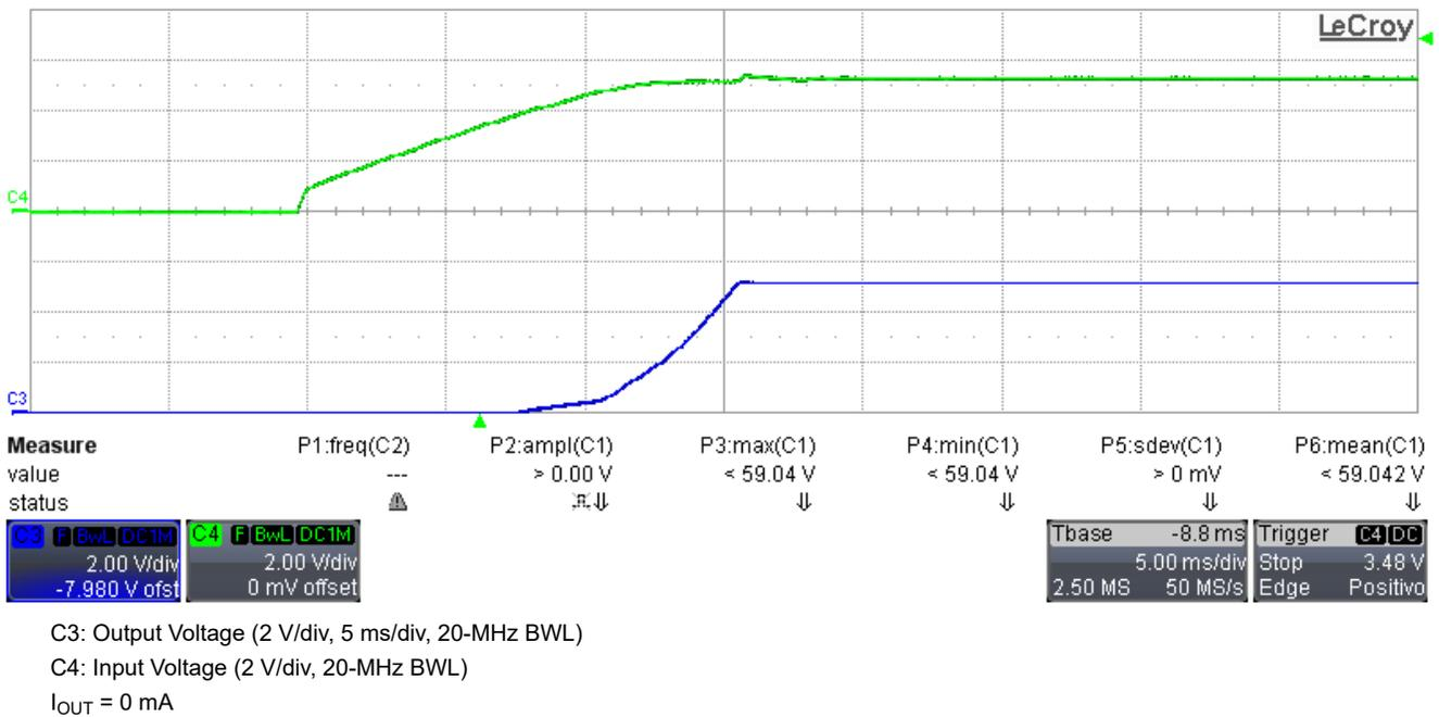
Figure 3-6. Start-Up With  $I_{OUT} = 0 \text{ A}$
