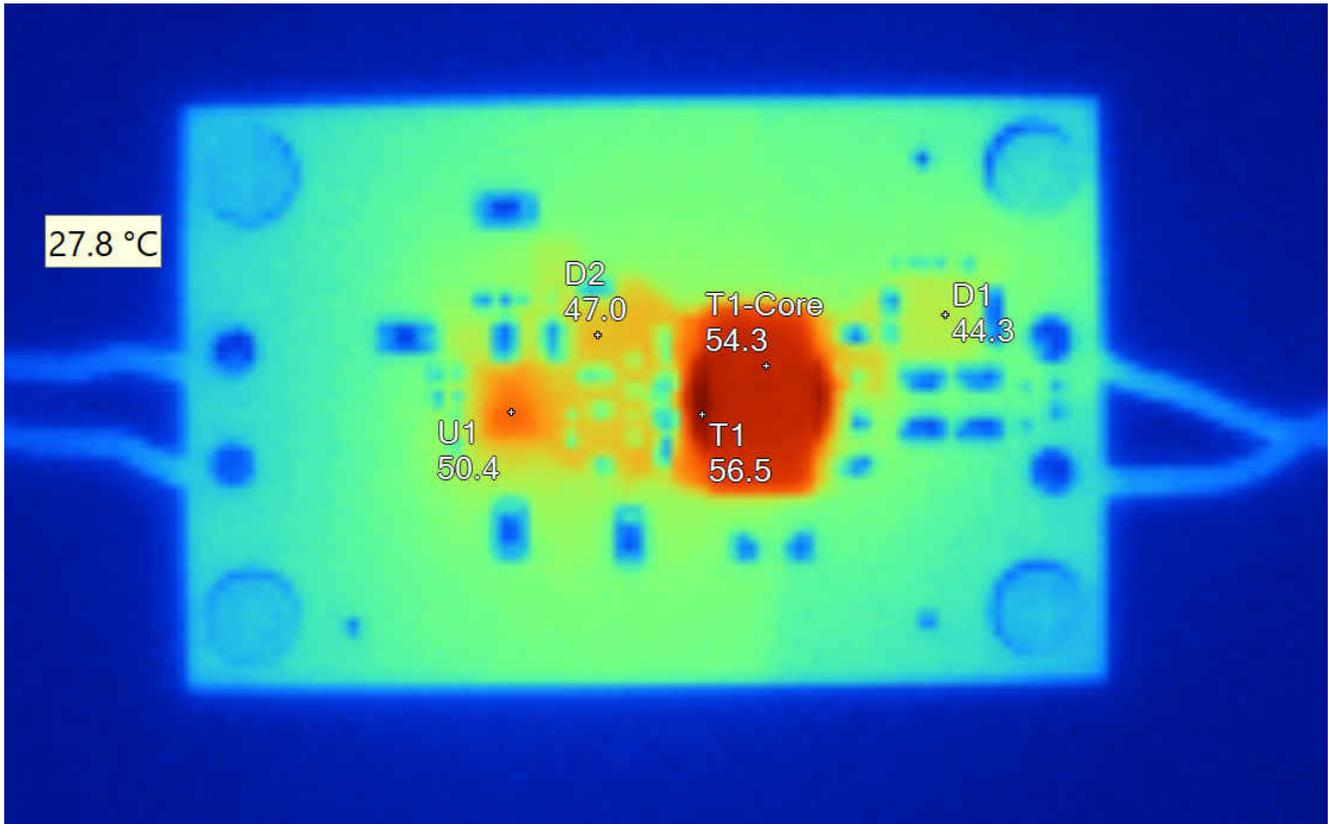
Conditions:  $V_{IN} = 5$  VDC, fully loaded; image taken after 60 minutes
