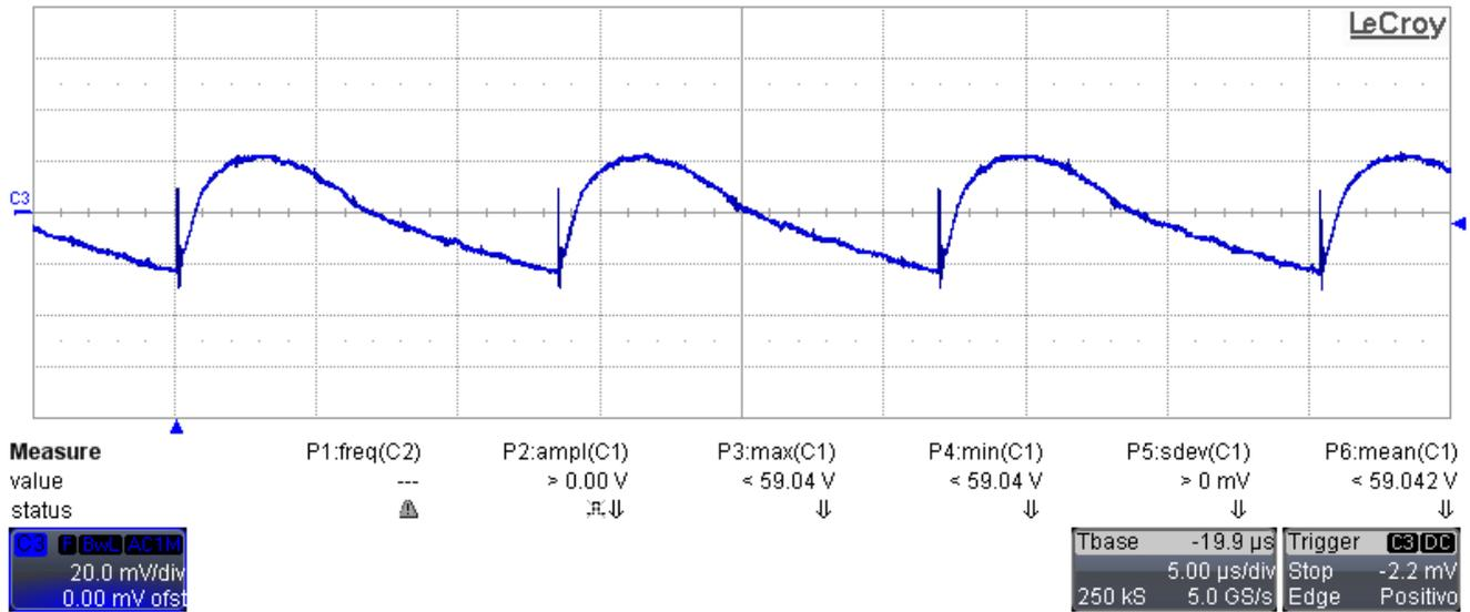
**Figure 3-4. C3: Output Voltage (20 mV/div, 5  $\mu$ s/div, AC coupling, 20-MHz BWL)**
