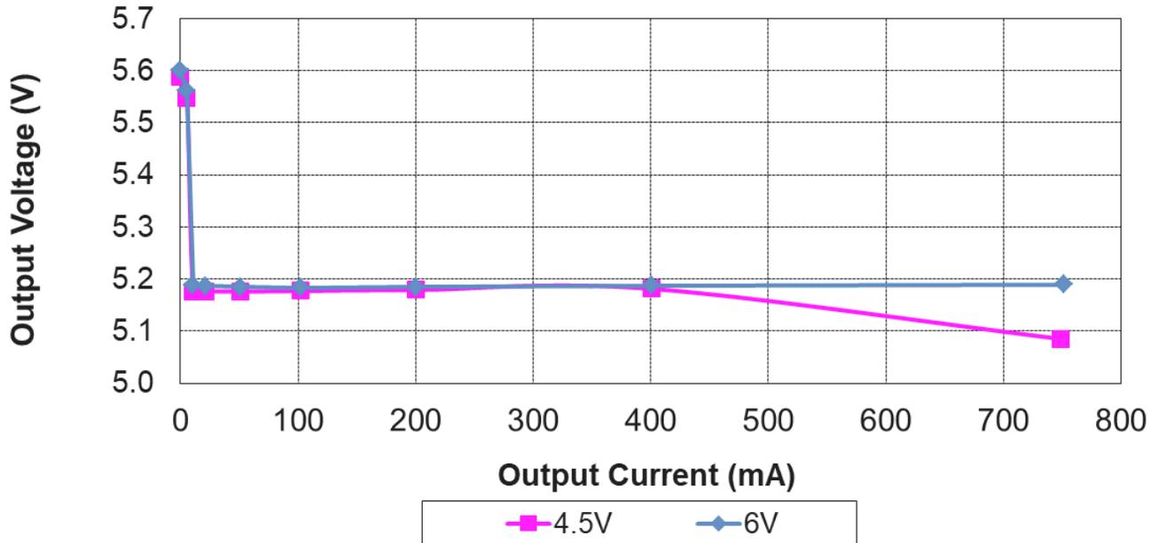
Figure 2-2. Output Voltage Regulation
