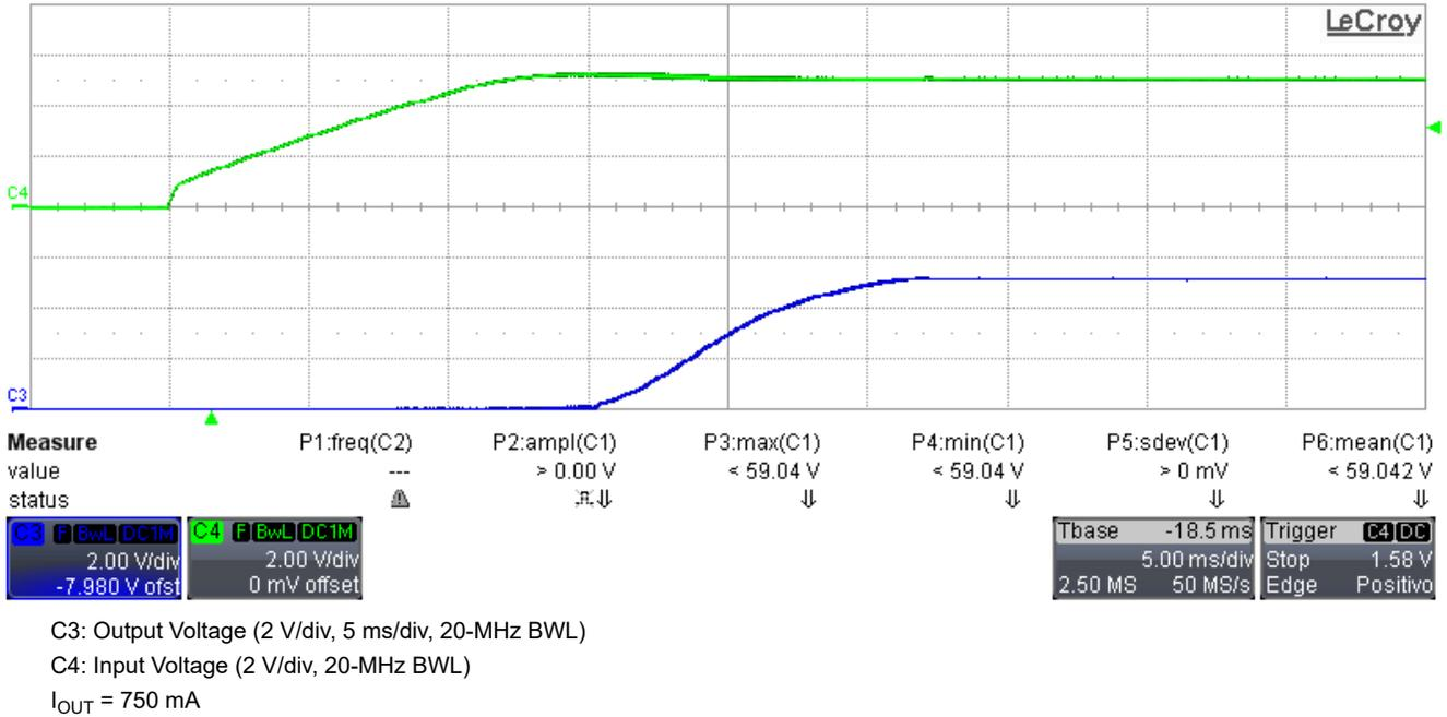
Figure 3-5. Start-Up With  $I_{OUT} = 750 \text{ mA}$
