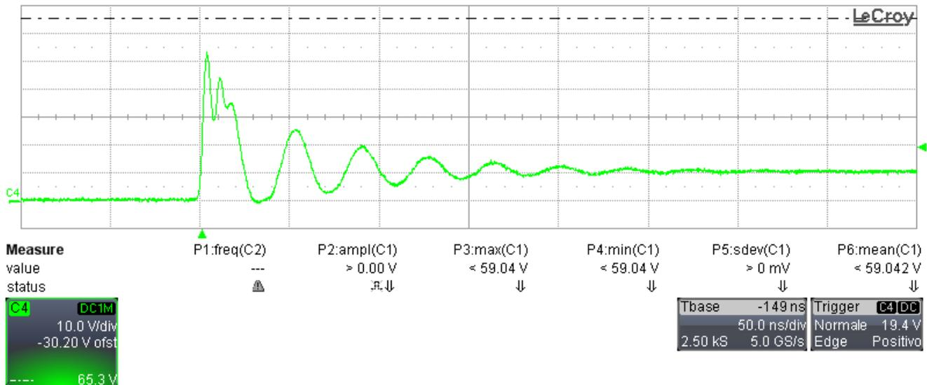
Figure 3-2. C2: Switch Node of U1 (TP2) (10 V/div, 50 ns/div, no BWL),  $V_{IN} = 5\text{ V}$
