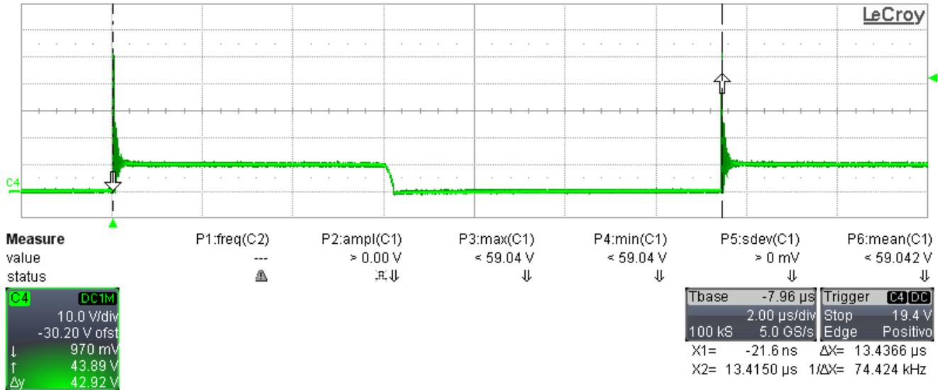
Figure 3-1. C2: Switch Node of U1 (TP2) (10 V/div, 2 μs/div, no BWL),  $V_{IN} = 5\text{ V}$
