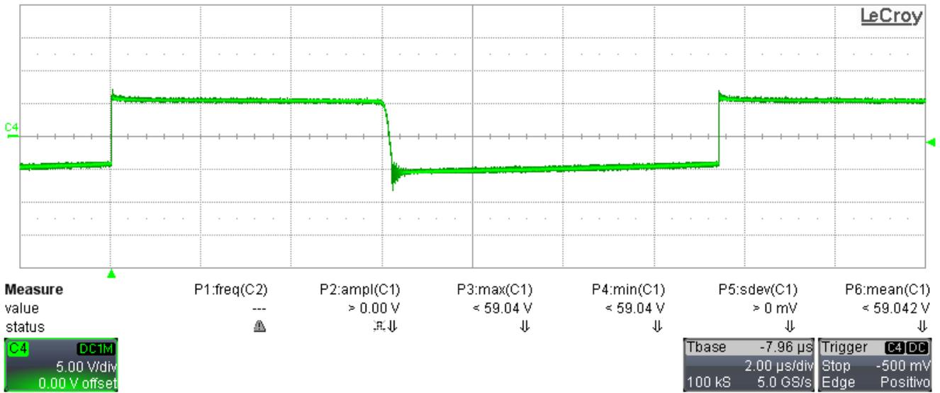
Figure 3-3. C4: Anode of D1 vs Secondary Ground (5 V/div, 2  $\mu$ s/div, no BWL)
