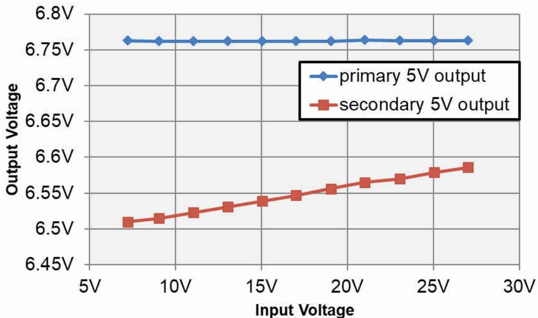
Figure 2-9. 5-V LDOs Input Voltages vs Input Voltage
