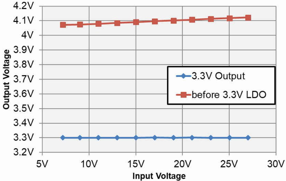
Figure 2-10. 3.3-V Output Voltage vs Input Voltage
