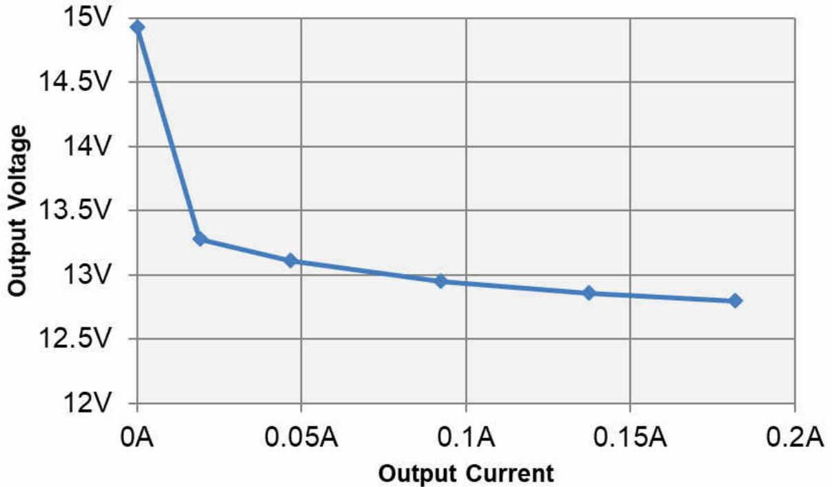
Due to peak detection at **zero** load, this output needs to be clamped by Zener diode or minimum load.
