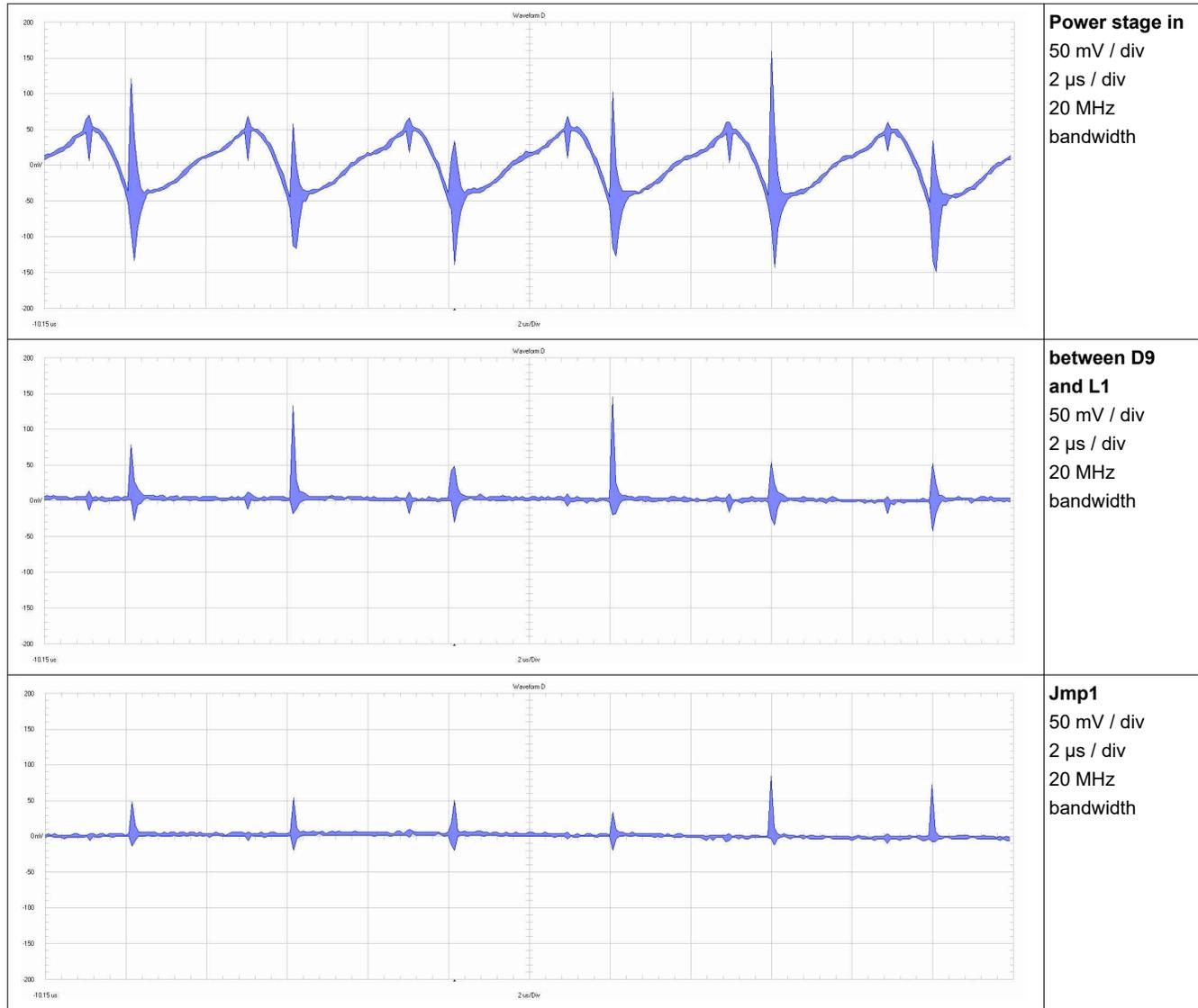
**Figure 3-4. Input Voltage Ripple**
