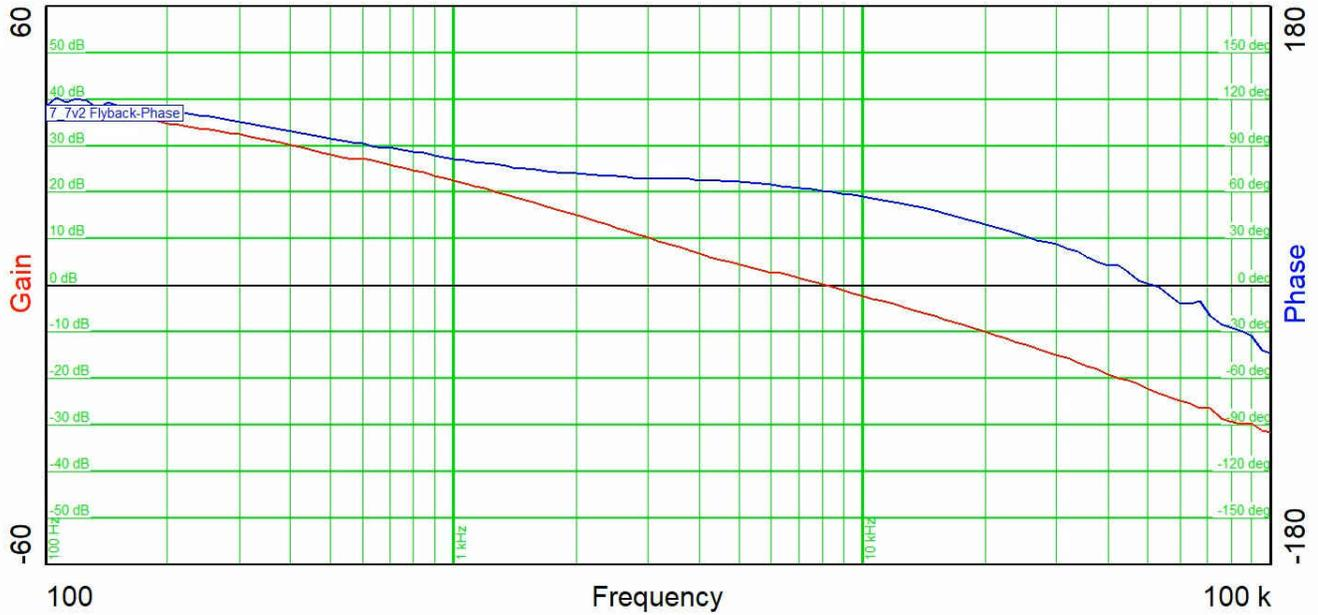
**Figure 2-15. Frequency Response for 7.2-V Input Voltage**
