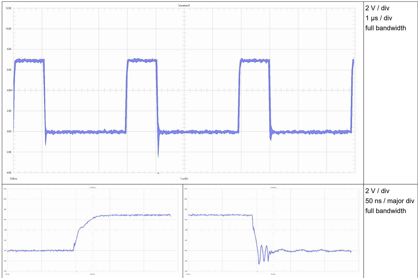
**Figure 3-2. Switching (Q1 Gate to GND)**
