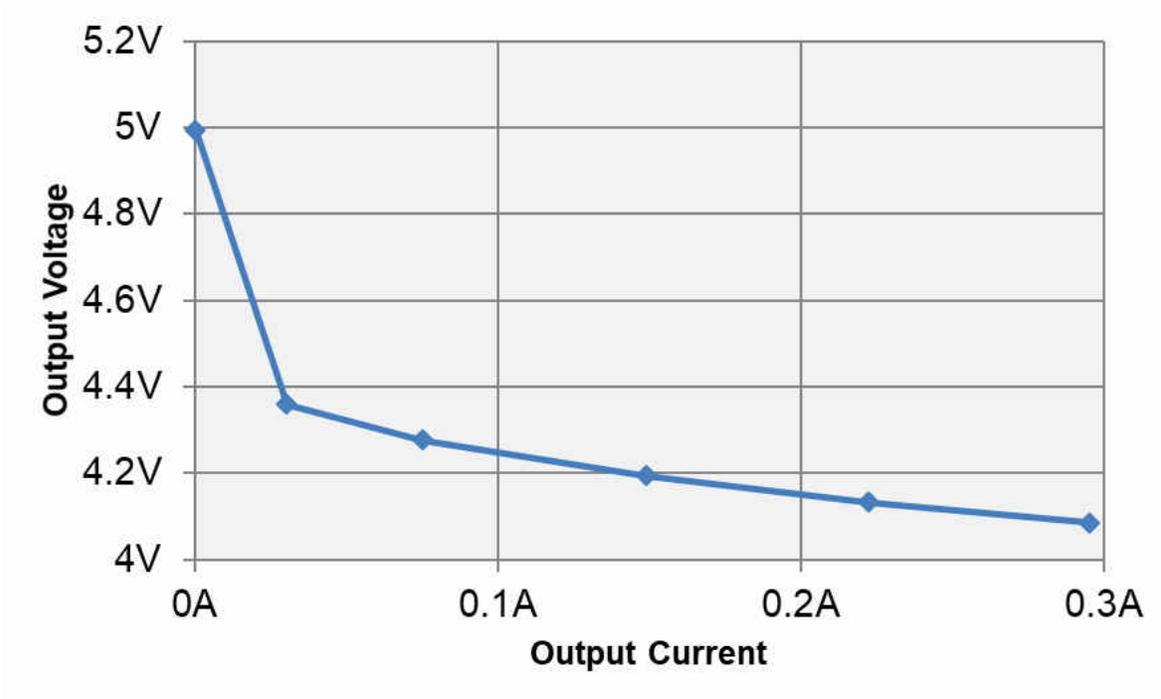
Figure 2-6. Voltage at 3.3-V LDO Input vs Output Current
