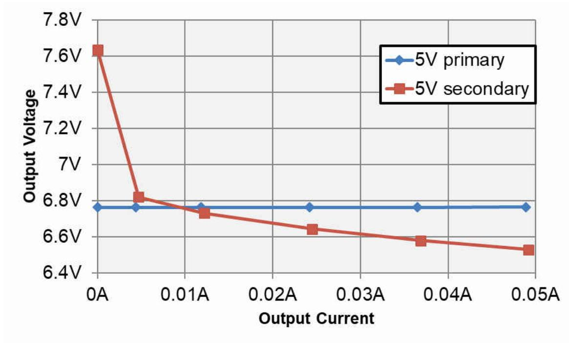
Figure 2-4. Voltages at 5-V LDO Inputs vs Output Current
