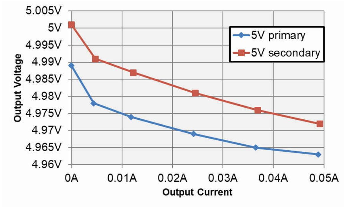
Figure 2-3. 5-V Output Voltages vs Output Current at LDO Output
