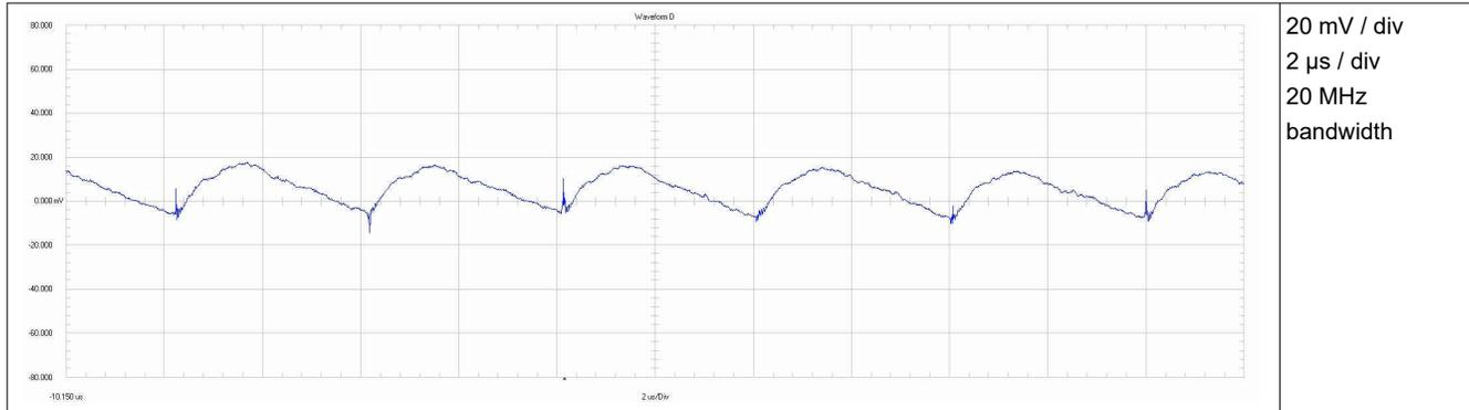
Figure 3-9. Output Voltage Ripple (12 V)
