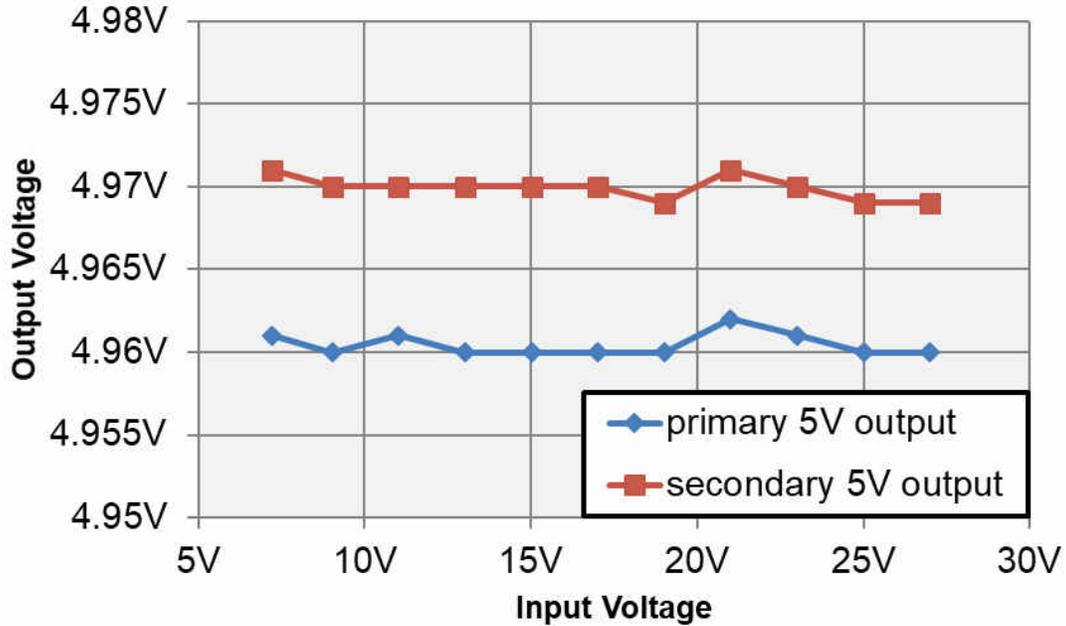
Figure 2-8. 5-V Output Voltages vs Input Voltage
