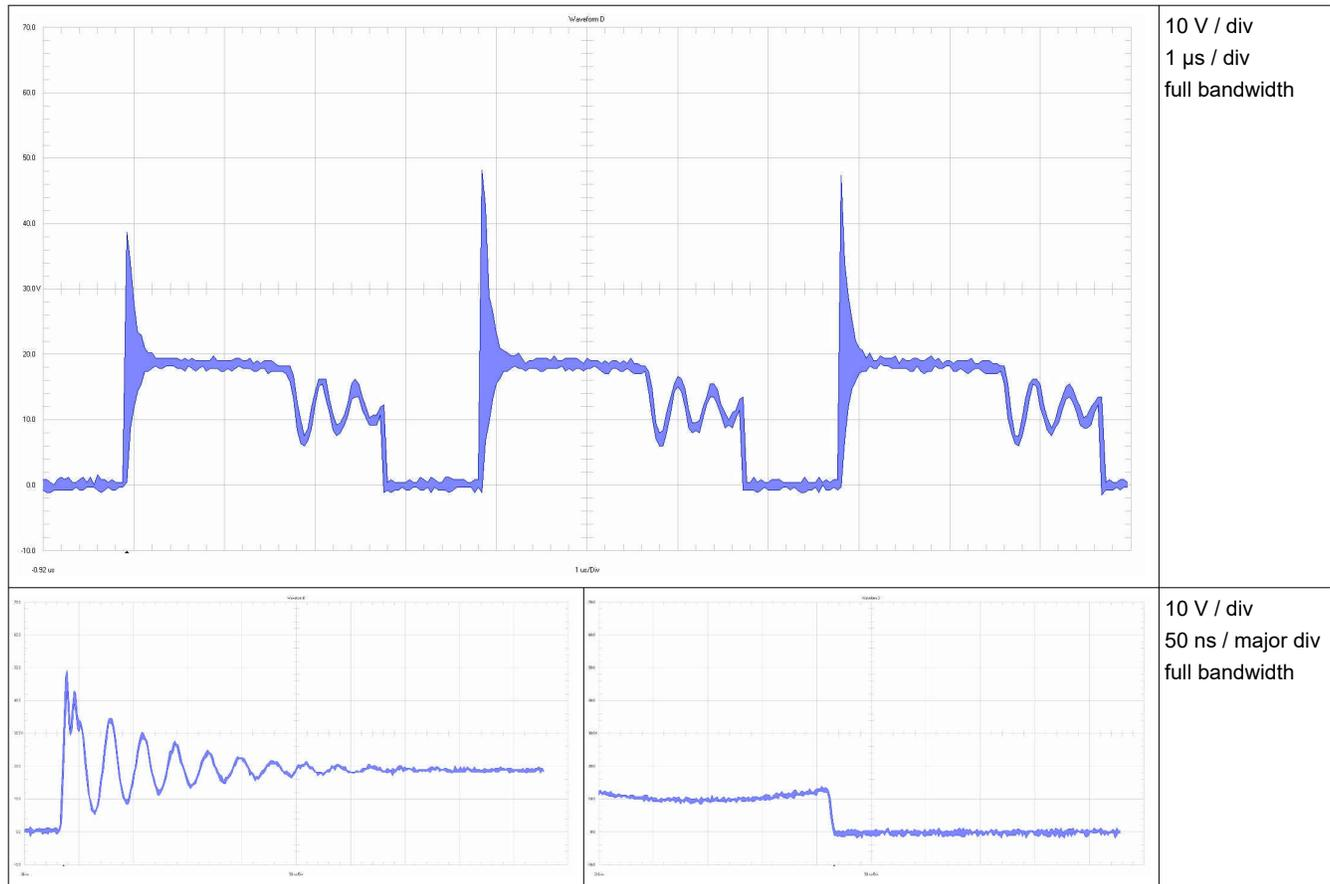
**Figure 3-1. Switchnode (Q1 Drain to GND)**
