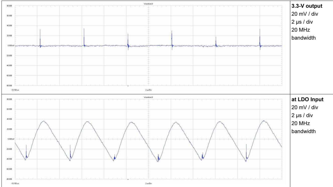
Figure 3-8. Output Voltage Ripple (3.3 V)
