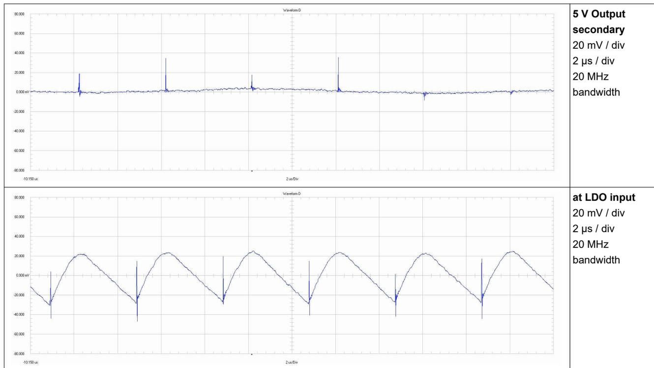
Figure 3-7. Output Voltage Ripple (5 V<sub>s</sub>)
