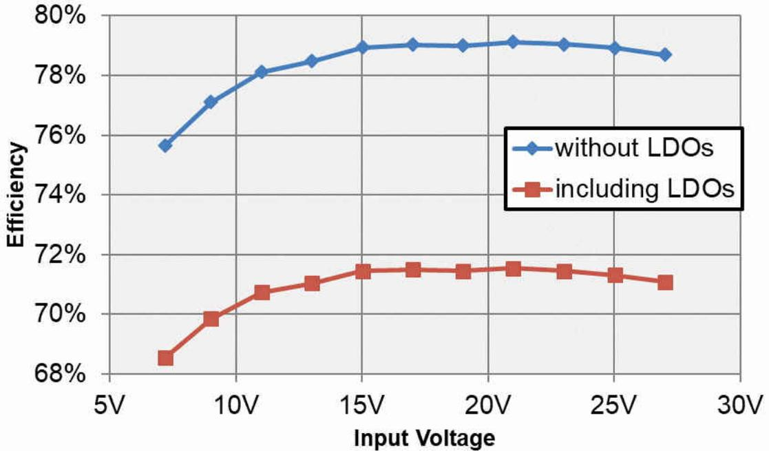
Figure 2-12. Efficiency vs Input Voltage
