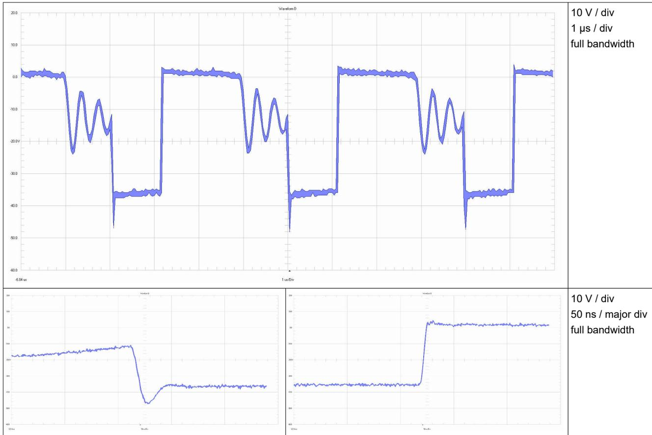
**Figure 3-3. D1 (Anode to 12 V<sub>OUT</sub>)**
