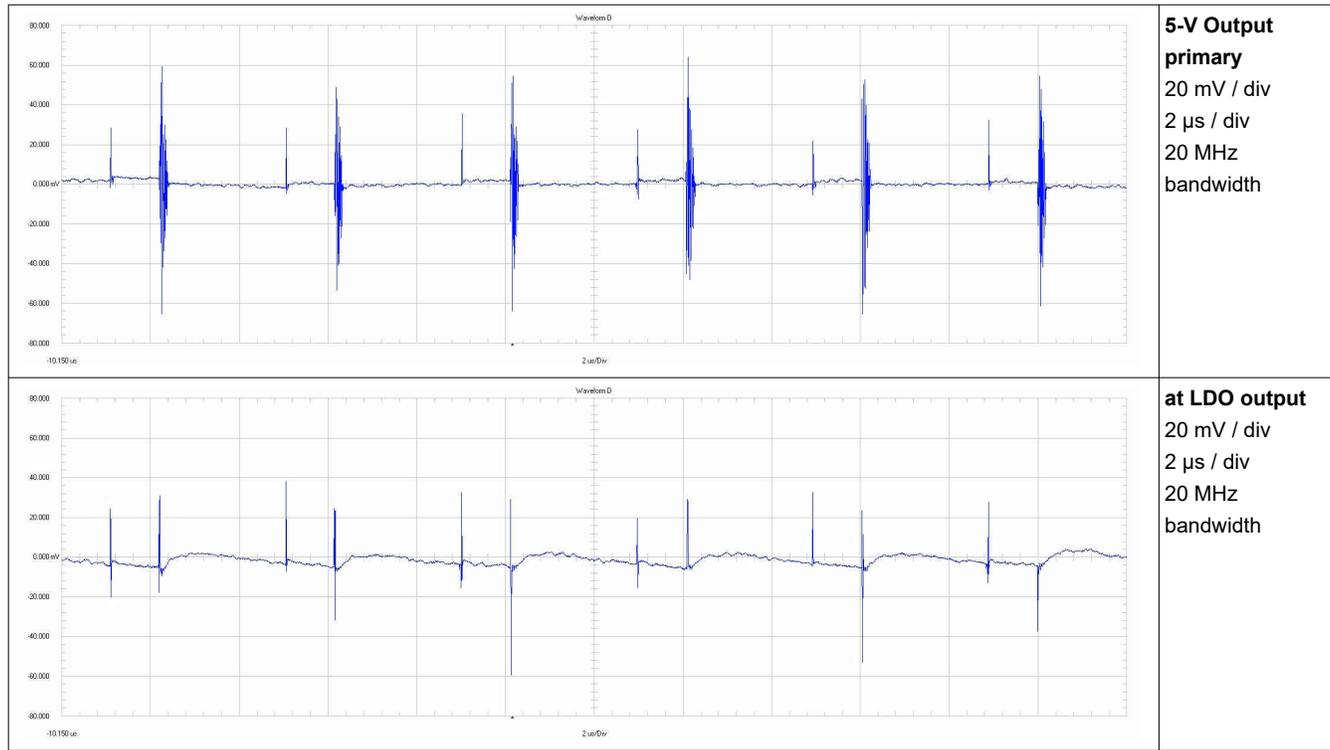
Figure 3-6. Output Voltage Ripple (5 V<sub>p</sub>)
