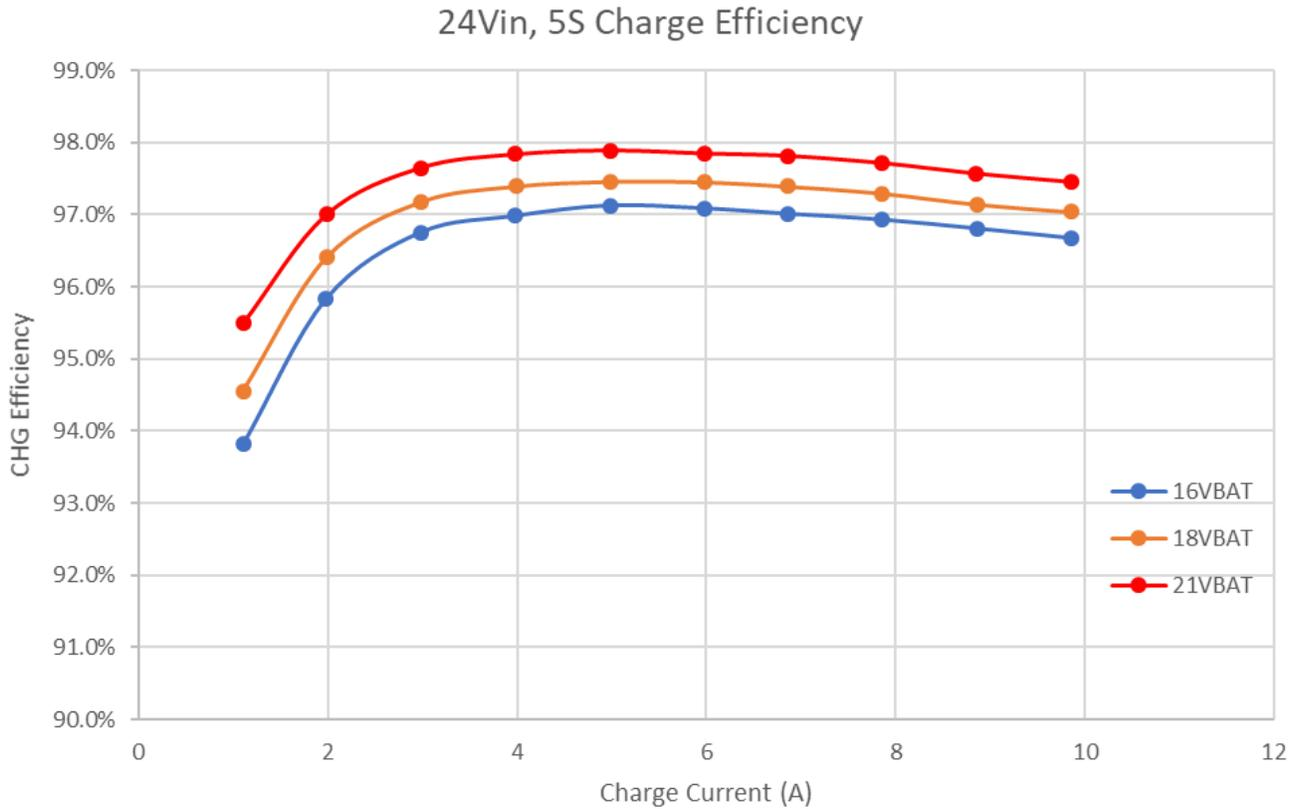
Figure 2-1. Charge Efficiency Graph
