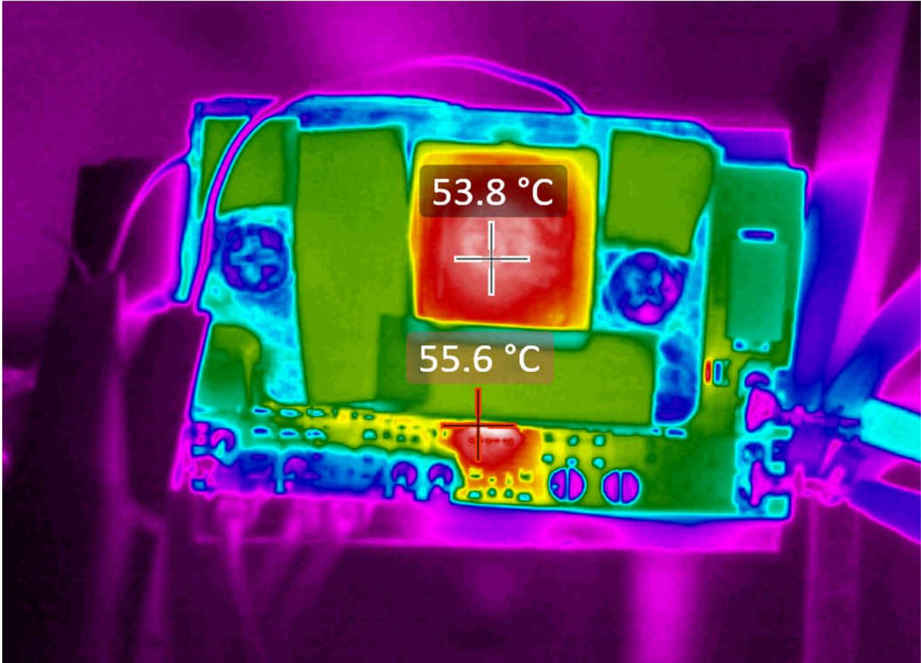
Figure 2-2. VBUS = 24 V, VBAT = 21 V, IBAT = 9.6 A, About 200 W, IC Temp = 55.6°C, Q1 FET = 53.6°C, IND Temp = 53.8°C (With Heat Sink, About 200 LFM Airflow)
