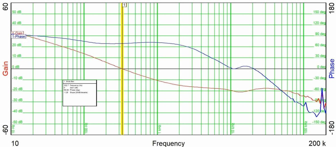
Figure 4-2. Control Loop - Bode Plot
