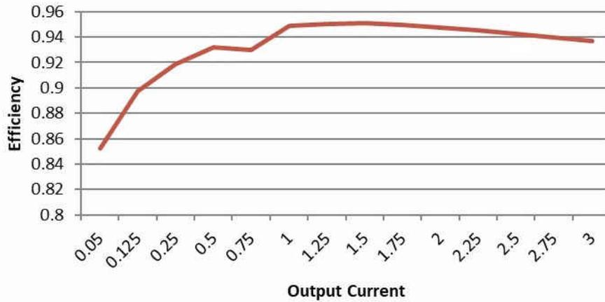
Figure 4-3. Efficiency, 3.6  $V_{IN}$
