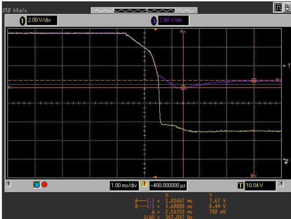
Channel 1 – Boost converter  $V_{IN}$  [2 V/div, 1 ms/div, DC coupled]
