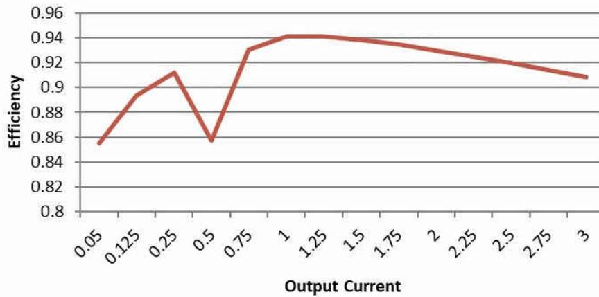
Figure 4-4. Efficiency, 3.0  $V_{IN}$
