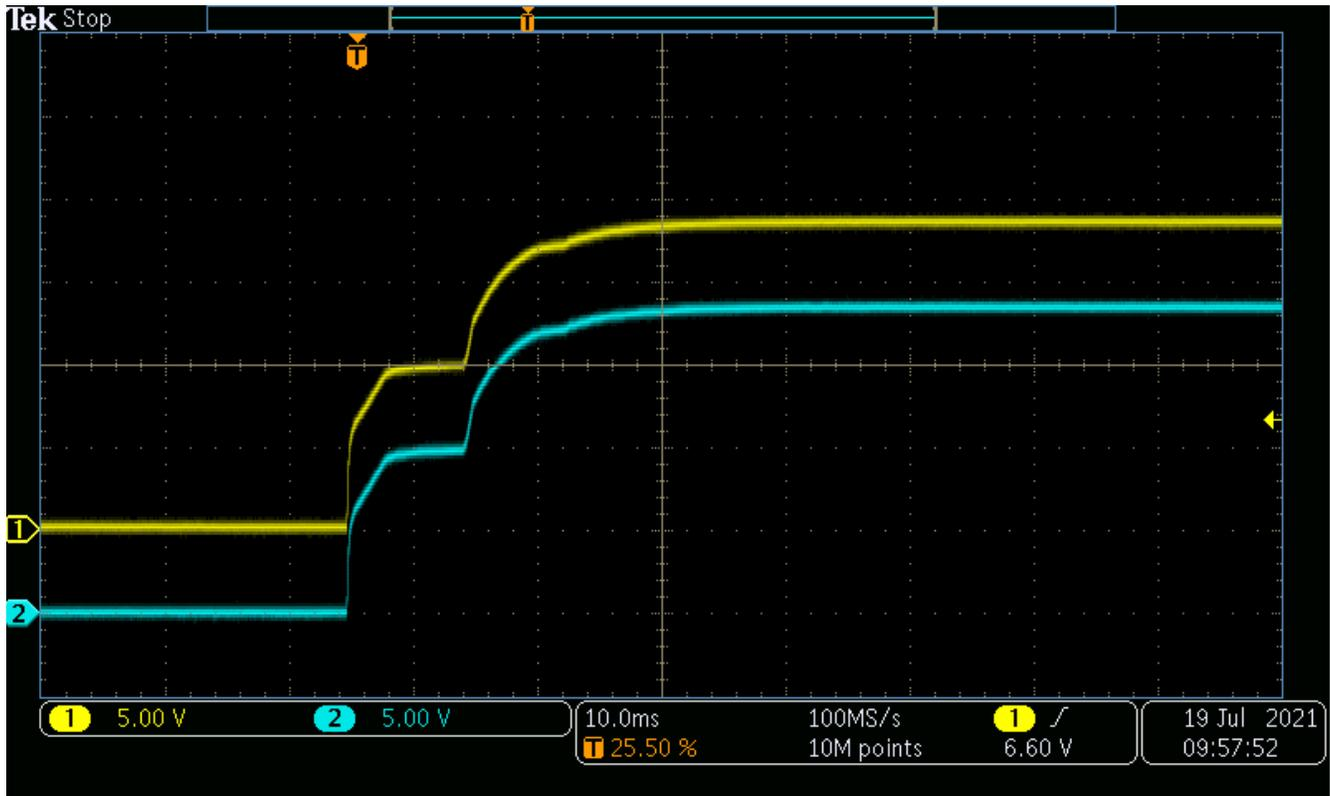
Figure 4-13. LLC Converter Start-up, 30 V<sub>IN</sub>, No Load
