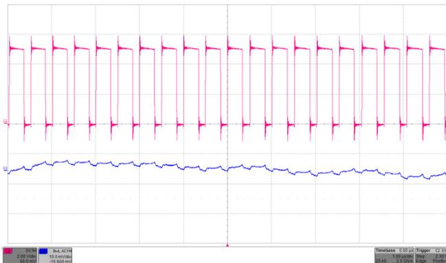
5Vin, 3.3V/1.5A, Vout ripple: 3mVpp
