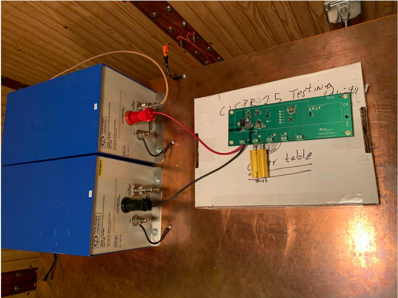
EMI setup with 2-ohm on board resistive load
