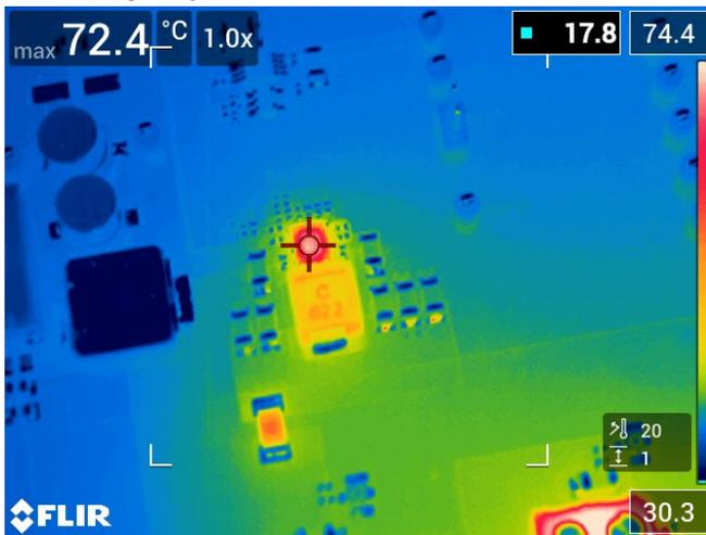
12Vin, 5V/2.5A, 1.1V/2.2A, 3.3V/1.65A, 1.8V/0.18A, Tmax(U1)=72.4C, Room Temp, Natural Convection
