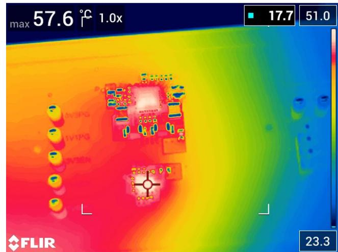
12Vin, 5V/2.5A, 1.1V/2.2A, 3.3V/1.65A, 1.8V/0.18A, Tmax(U2)=52.2C, Tmax(U3)=57.6C Room Temp, Natural Convection
