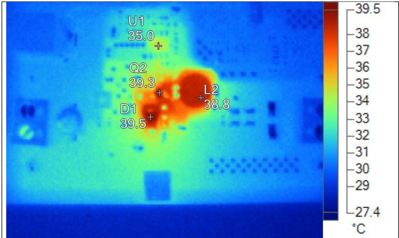
**Figure 3 Thermal Image (12Vin, 1Aout)**
