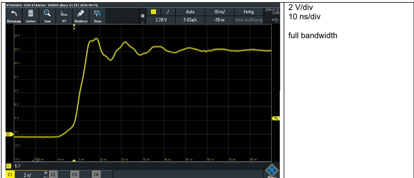
**Figure 6 Switch Node with 470pF**
