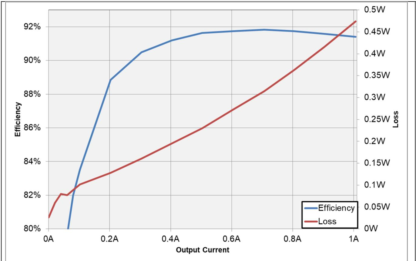
**Figure 1 Efficiency and Loss vs Output Current**
