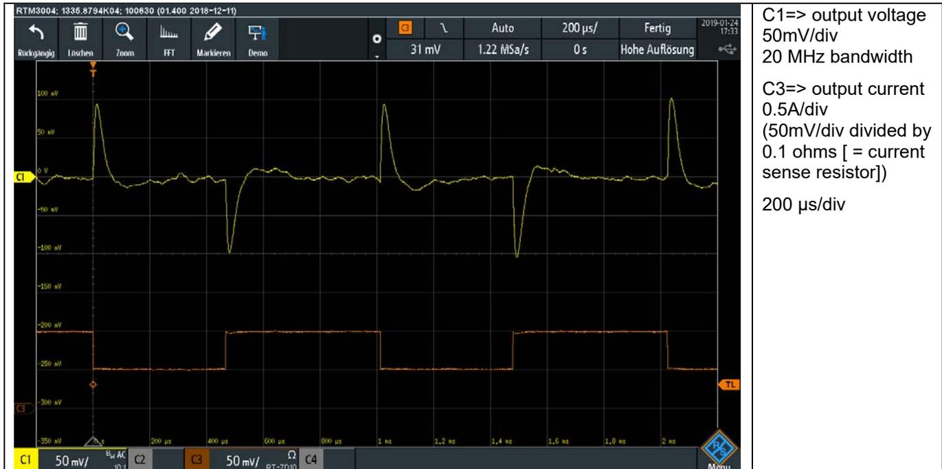
Figure 14 Load Transient
