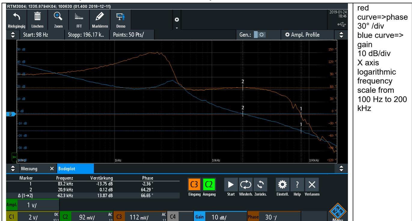
**Figure 12 Bode Plot generated with R&S Oszi**
