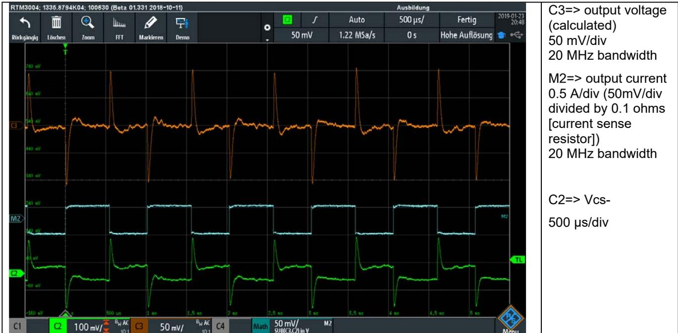
Figure 15 Load Transient
