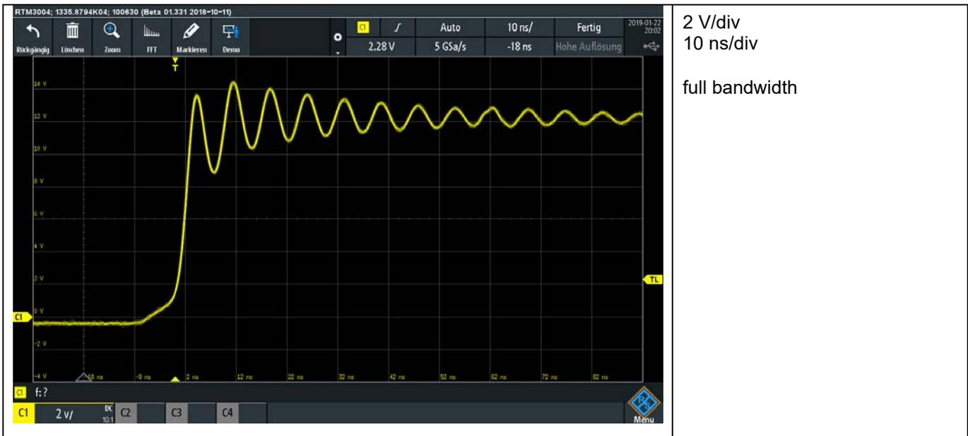
**Figure 5 Switch Node without snubber**
