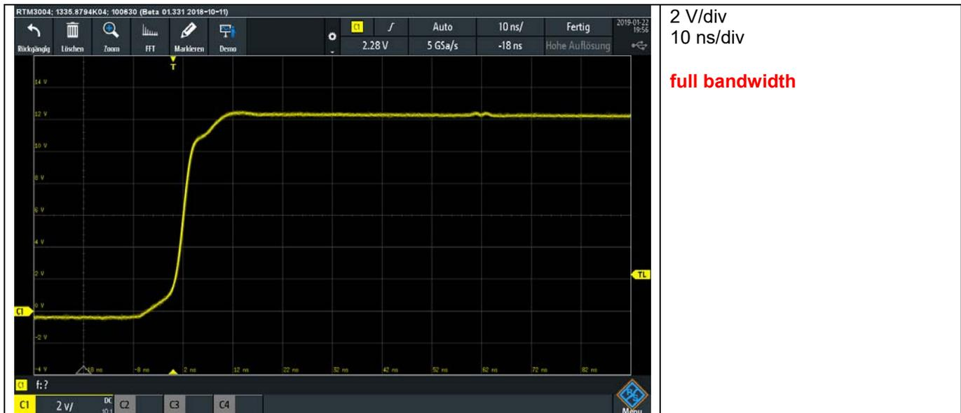
**Figure 7 Switch Node with C111=470pF and R111=7.5 Ohms**
