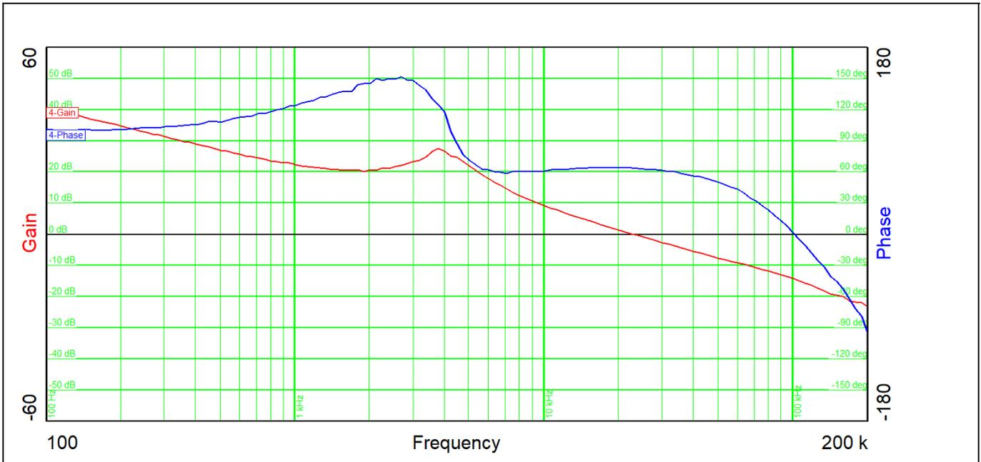
**Figure 13 Bode Plot generated with Venable NWA**
