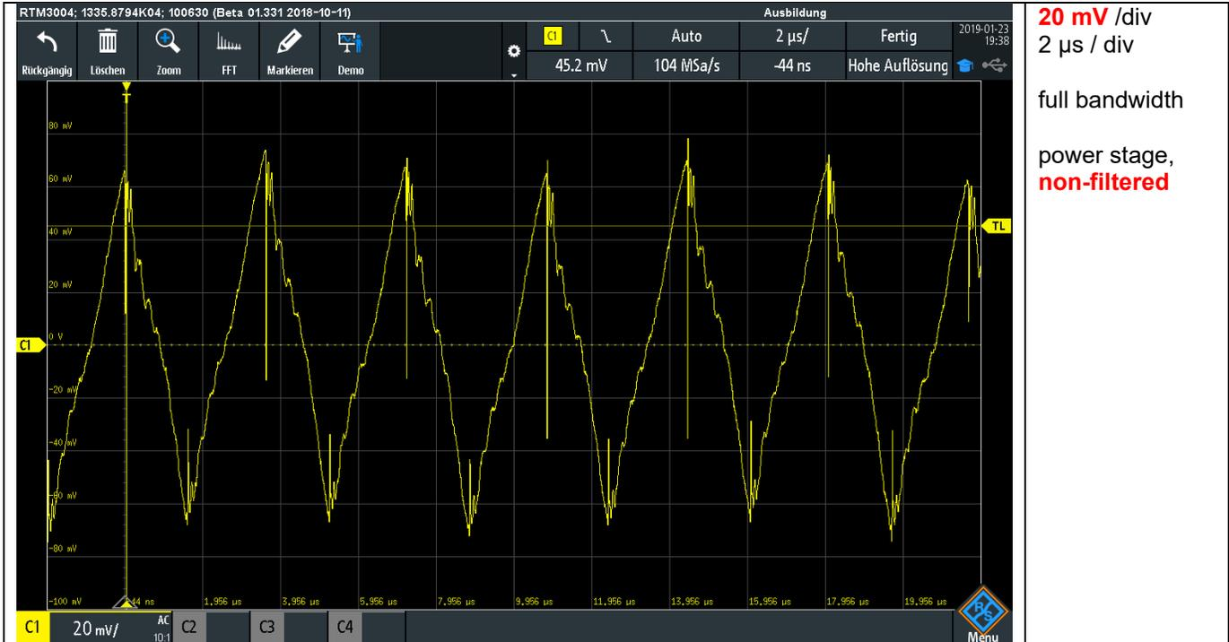
Figure 11 Power Stage Input (C1)
