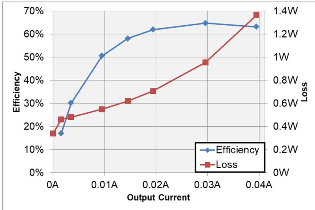
Figure 1 Efficiency and Loss vs Output Current
