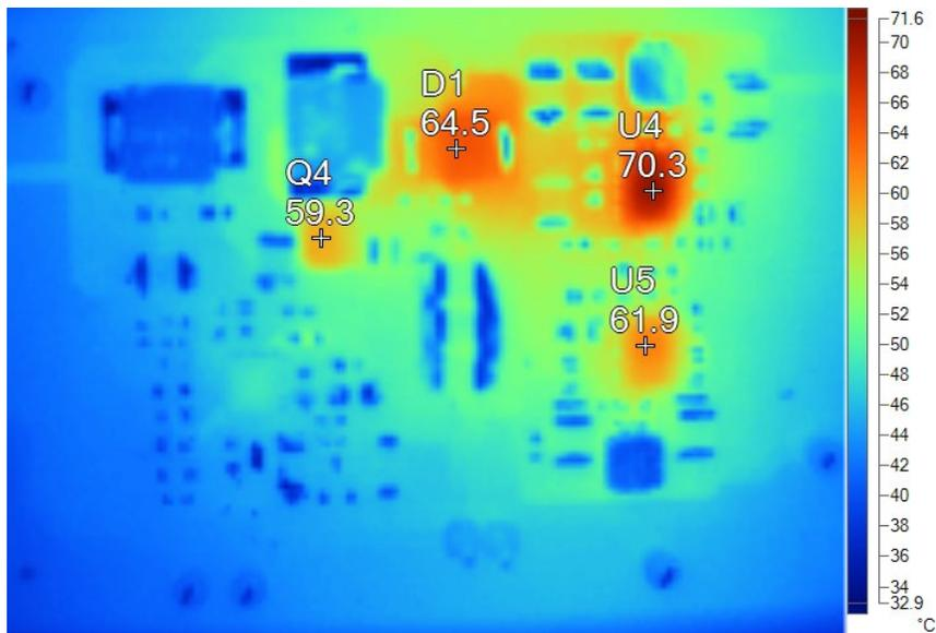
**Figure 3: Thermal @ VIN = 6 V**
