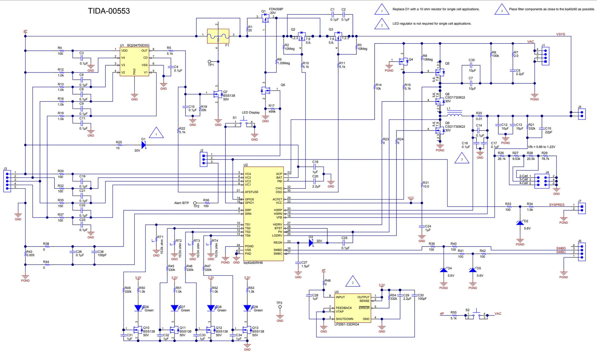
1 Replace D1 with a 10 ohm resistor for single cell applications.
