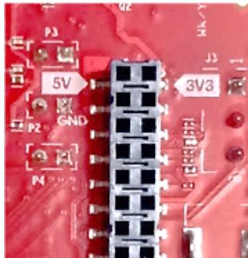
**Figure 9.** 3V3 and 5V Marking on BoosterPack
