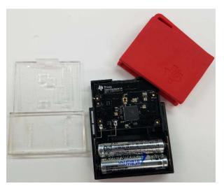
Figure 11. Replacing the Batteries
