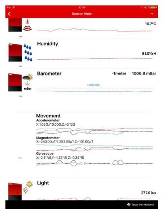
Figure 7. SensorTag Sensor Data
