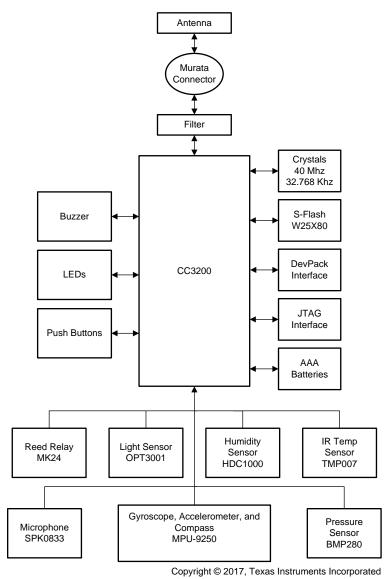
Figure 2. CC3200 SensorTag Block Diagram
