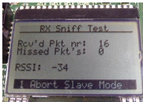
**Figure 30 RX Sniff Test Slave Statistics 2**
