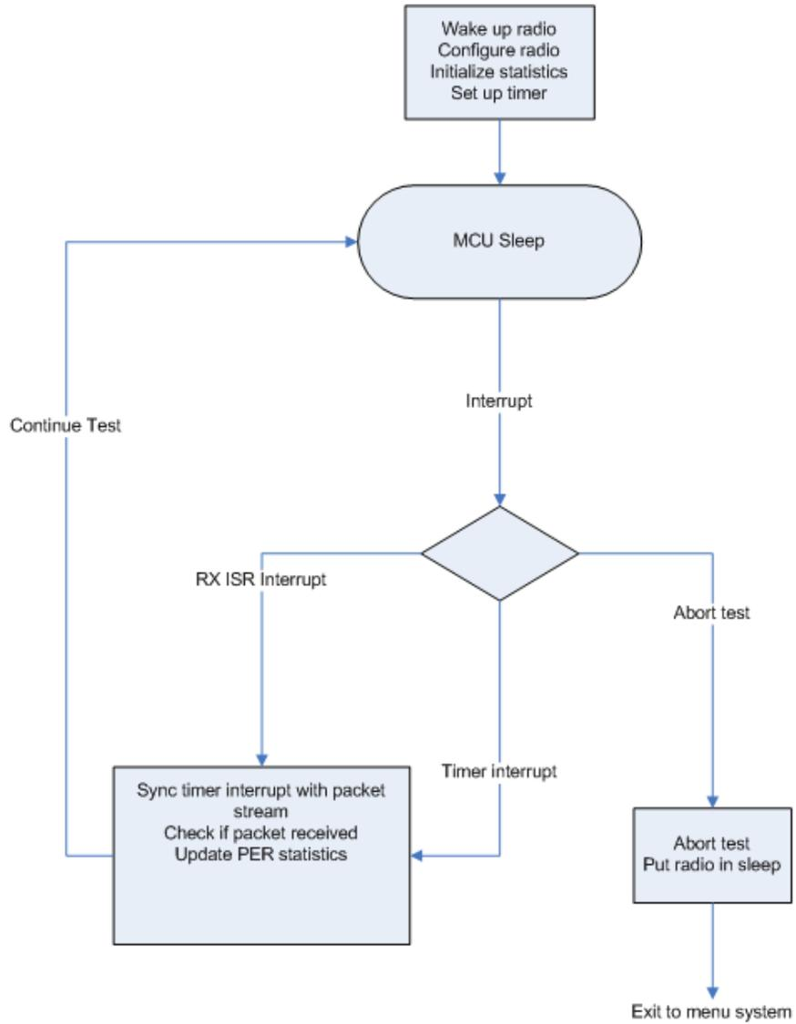
**Figure 16 One-way PER test at Master**
