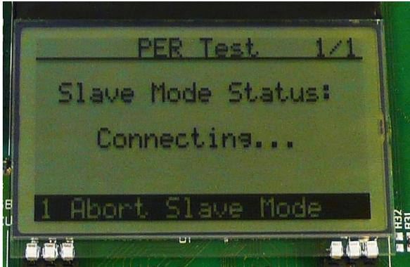
**Figure 10 Slave node waiting for configuration packet**
