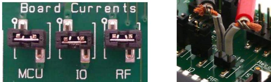
**Figure 32 Current measurement**
