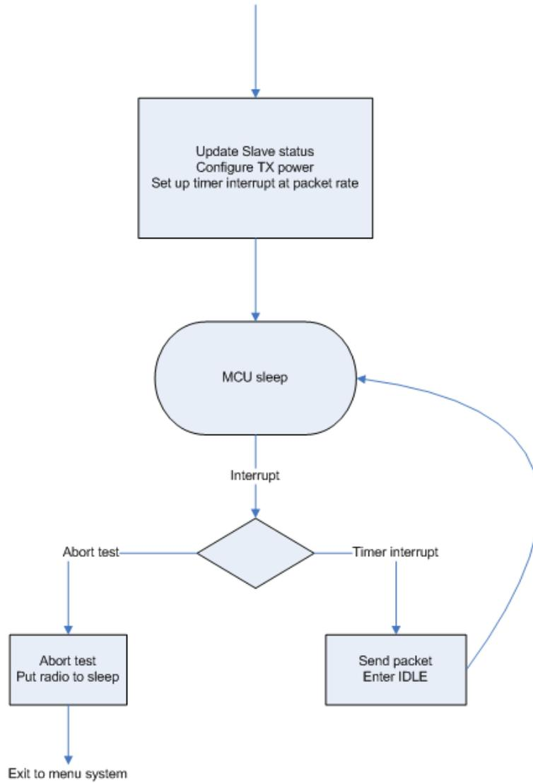
**Figure 17 One-way PER test at Slave**
