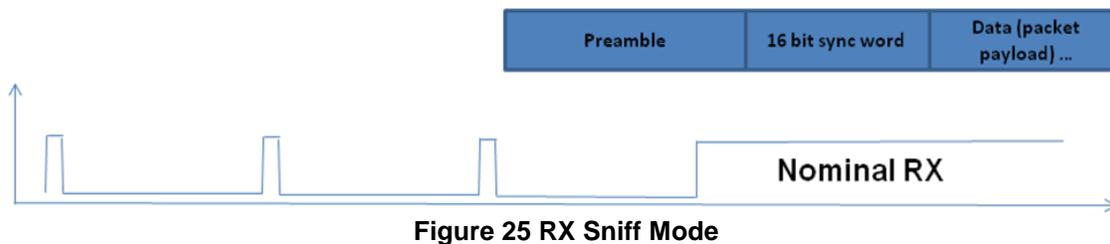
The configuration uses 1.2 kbps data rate with 4 byte preamble. In this example the average current consumption when the radio is duty cycling is measured to 1.9 mA opposed to 25.1 mA which is the current consumption when the receiver is set in continuous RX.
