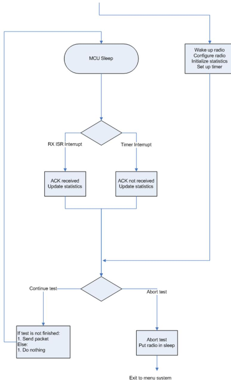
**Figure 18 Two-way PER test at Master**
