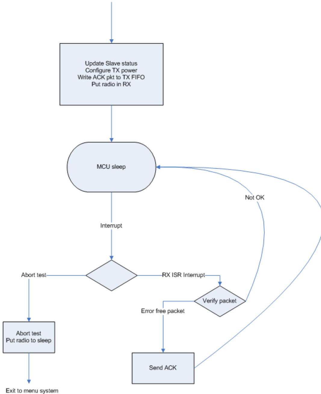
**Figure 19 Two-way PER test at Slave**
