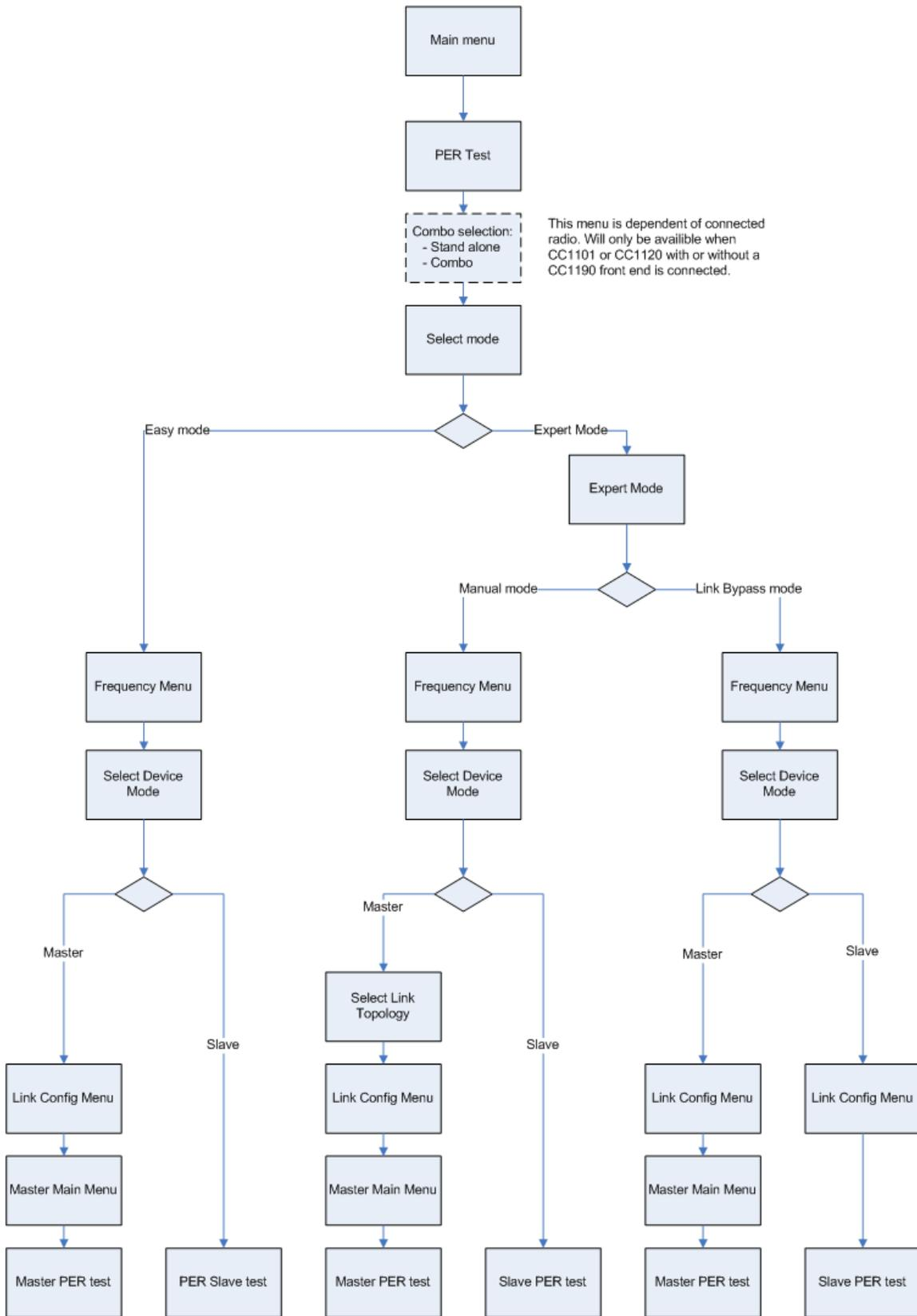
**Figure 6 PER test Menu Tree**
