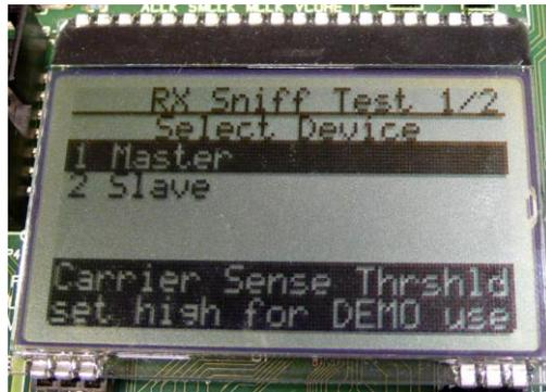
**Figure 28 RX Sniff Test Device Mode Menu**
