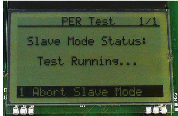
**Figure 11 Slave node running PER test**
